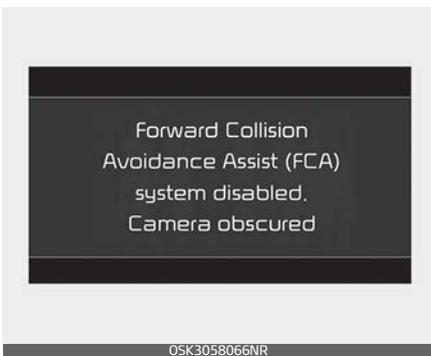
When the camera is covered with dirt, snow, or debris, Forward Collision-Avoidance Assist operation may not be able to detect other vehicles. In this case, the warning message appears to warn the driver.
