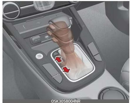
Whether the vehicle is stationary or in motion, manual mode is selected by pushing the shift lever from the
