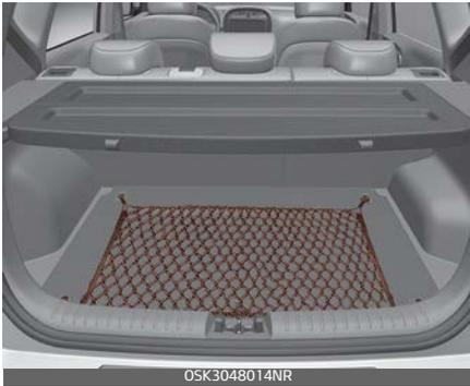
To keep items from shifting in the cargo area, you can use the 4 holders located in the cargo area to attach the luggage net.
