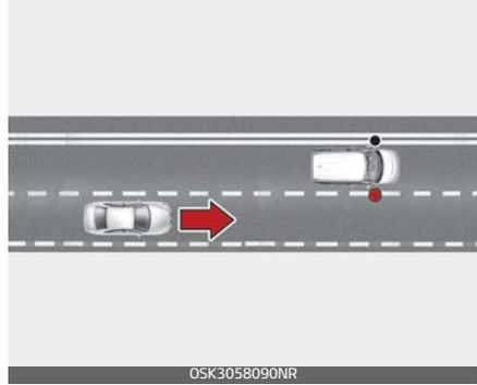
Blind-Spot Collision Warning will warn you when it detects a vehicle is approaching in an adjacent lane at a high rate of speed. If the driver activates the turn signal when the system detects an oncoming vehicle, the system sounds an audible warning.
