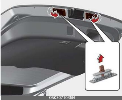
1. Remove the lamp assembly by using a flat-blade screwdriver.
