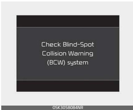
If there is a problem with Blind-Spot Collision Warning, a warning message will appear and the light on the switch will turn off. The function will turn off automatically. Have your vehicle inspected by an authorized Kia dealer.
