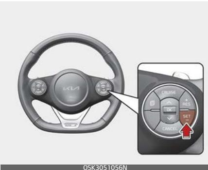
4. Release the accelerator pedal. The desired speed will automatically be maintained.
