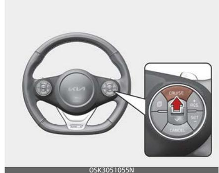
1. Press the CRUISE button on the steering wheel, to turn the function on. The cruise indicator light will illuminate.
