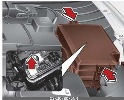
4. Check the removed fuse; replace it if it is blown. Spare fuses are provided in the engine compartment fuse panel.
