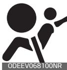
If any of the following conditions occur, this indicates a malfunction in the air bag system. Have an authorized Kia dealer inspect the air bag system as soon as possible.
