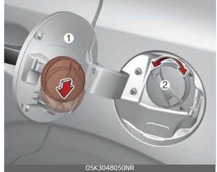
4. To remove the cap turn the fuel filler cap (2) counterclockwise.
