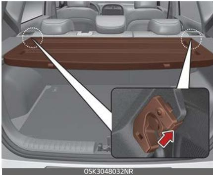
3. While lifting the cover up, hold the area near the front slots. Then, pull up the cover at approximately 45 ° angle.
