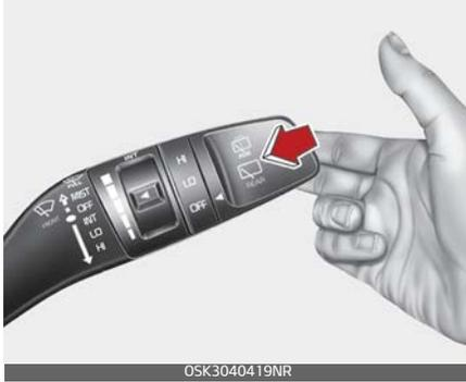
1. Move the wiper speed control switch to the OFF position.
