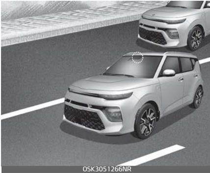
When the function detects the vehicle straying from its lane, it warning the driver with a visual and audible warning, while applying a slight countersteering torque, trying to prevent the vehicle from moving out of its lane.
