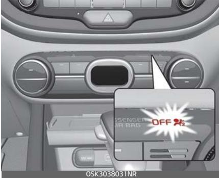
The occupant detection system is designed to detect the presence of a properly-seated front passenger and determine if the passenger's front air bag should be enabled (may inflate) or not. Only the front passenger front air bag is controlled by the Occupant Detection System.
