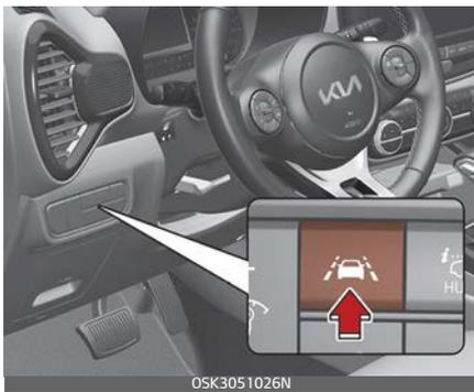
To activate/deactivate Lane Keeping Assist, with the ignition switch or ENGINE START/STOP button in the
