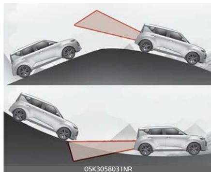
Blind-Spot Collision Warning may not operate properly when driving on a slope. In certain instances the
