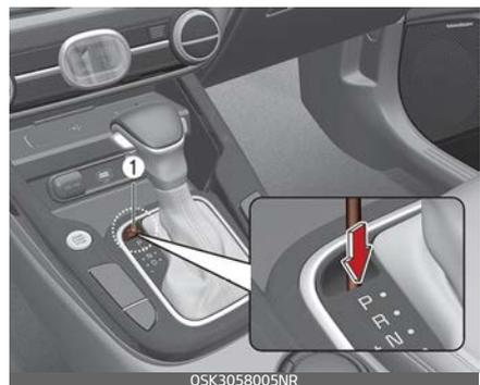
If the shift lever cannot be moved from the P (Park) position into R (Reverse) position with the brake
