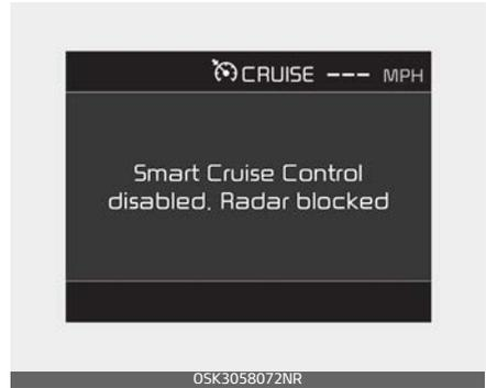
When the sensor lens cover is blocked with dirt, snow, or debris, Smart Cruise Control operation may stop temporarily. If this occurs, a warning message will appear on the LCD display. Remove any dirt, snow, or debris and clean the radar sensor lens cover before operating Smart Cruise Control.
