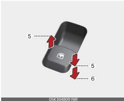
Pressing the power window switch momentarily to the second detent position (6) completely lowers the window even when the switch is released. To stop the window at the desired position while the window is
