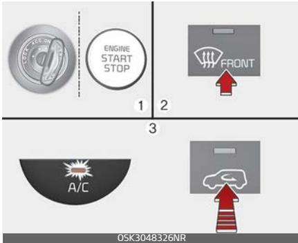
1. Turn the ignition switch or ENGINE START/STOP button to the ON position.
