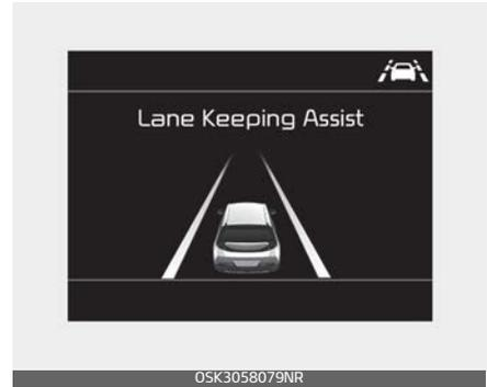
If the speed of the vehicle is over 40 mph (64 km/h) and the function detects lane markers, the color changes from gray to white.
