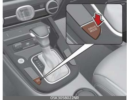
The mode changes whenever the DRIVE MODE button is pressed.
