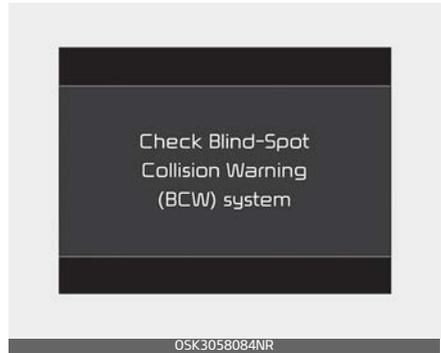
If there is a problem with Blind-Spot Collision Warning, a warning message will appear and the light on the switch will turn off. The function will turn off automatically. Rear Cross-Traffic Collision Warning and Rear Cross-Traffic Collision-Avoidance Assist will not operate also if Blind-Spot Collision Warning turns off due to malfunction. Have your vehicle inspected by an authorized Kia dealer.
