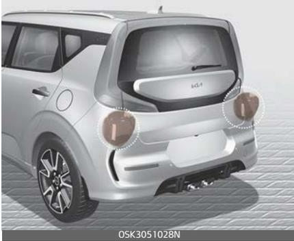
The rear corner radars are located inside the rear bumper for detecting the side and rear areas. Always keep the rear bumper clean for proper operation of the function.
