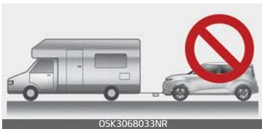
Your vehicle is not designed to be dinghy towed (with 4 wheels on the ground) behind a motor home. To avoid serious damage to your vehicle, do not tow your vehicle with four wheels on the ground.
