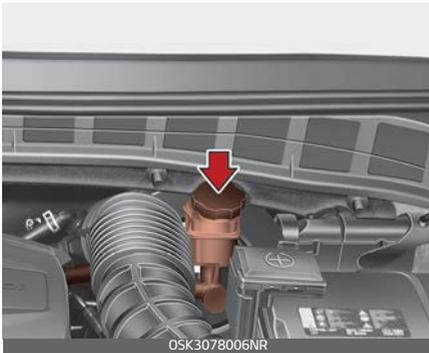
1. Before removing the reservoir cap and adding brake fluid, clean the area around the reservoir cap thoroughly to prevent brake fluid contamination.
