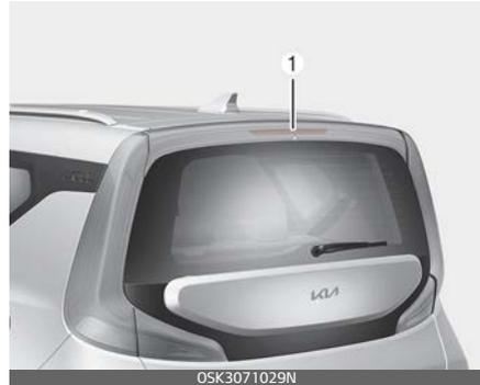
The LED lamps cannot be replaced as a single component because it is an integrated unit. The LED lamps has to be replaced with the unit.
