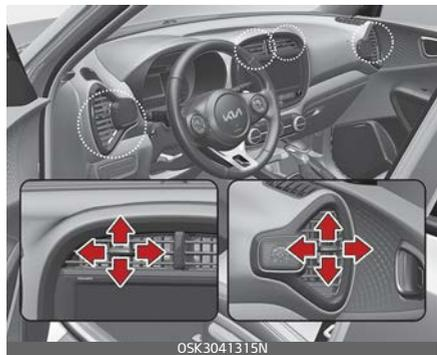
Also, you can adjust the direction of air delivery from these vents using the vent control lever as shown.
