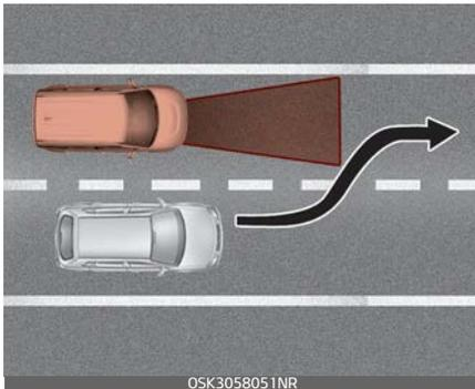
When a vehicle changes lanes in front of you, Forward Collision-Avoidance Assist may not immediately detect the vehicle, especially if
