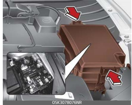
3. Check the removed fuse; replace it if it is blown. To remove or insert the fuse, use the fuse puller in the engine compartment fuse panel.
