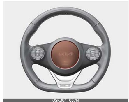
The horn will operate only when this area is pressed. Check the horn regularly to be sure it operates properly.
