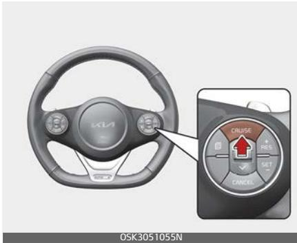
When Smart Cruise Control is not needed, press the [CRUISE] switch and deactivate the function.
