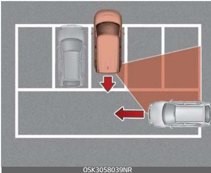
If the vehicle is parked rearward and the sensor detects the another vehicle in the rear area of the parking space, the function can warn or control braking.
