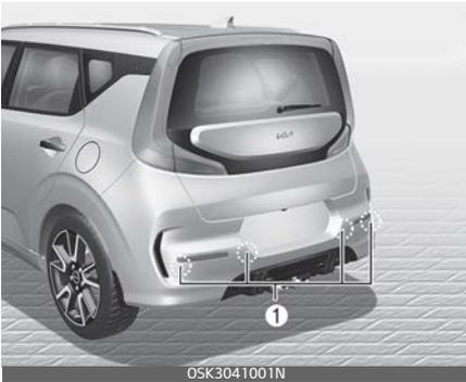
Reverse Parking Distance Warning is a supplemental function and it is not intended to nor does it replace the need for extreme care and attention of the driver. The sensing range and objects detectable by the back sensors (1) are limited. Whenever backing-up, pay as much attention to what is behind you as you would in a vehicle without Reverse Parking Distance Warning.
