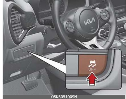
ESC checks where you are steering and where the vehicle is actually going. ESC applies the brakes on individual wheels and intervenes with the vehicle management system to stabilize the vehicle.
