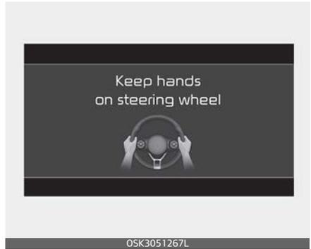
If the driver still does not have their hands on the steering wheel after several seconds, the function will only warn the driver when the driver crosses the lane lines. In this scenario, the function does not provide any steering inputs into the vehicle for you. Accordingly, you must take the necessary steps to maintain control of the vehicle and keep it within the lanes.
