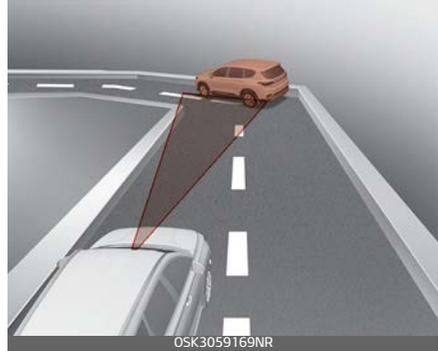
Forward Collision-Avoidance Assist may recognize a vehicle in the next lane or outside the lane when driving on a curved road. If this occurs, the function may unnecessarily alarm the driver and apply the brake.
