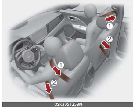
The pre-tensioner seat belts may be activated, when a frontal collision is severe enough, together with the air bags.
