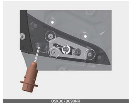
4. Remove the bulb from the socket by pressing it in and rotating it counterclockwise until the tabs on the bulb align with the slots in the socket. Pull the bulb out of the socket.
