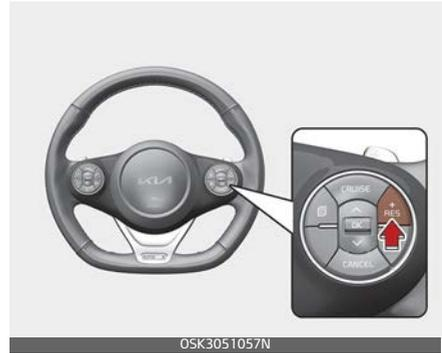
If any method other than the CRUISE button was used to cancel cruising speed and the function is still activated, the most recent set speed will automatically resume when you push the RES+ button.
