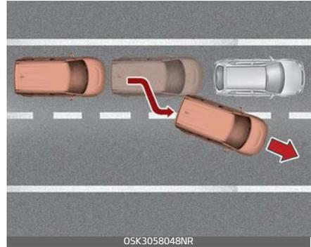
When driving in stop-and-go traffic, and a stopped vehicle in front of you merges out of the lane, Forward Collision-Avoidance Assist may not immediately detect the new vehicle that is now in front of you. In this case, you must maintain a safe braking distance, and if necessary, depress the brake pedal to reduce your driving speed in order to maintain a safe distance.
