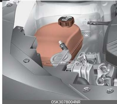
Do not remove the radiator cap when the engine and radiator are hot. Scalding hot coolant and steam may blow out under pressure which may result in serious injury.
