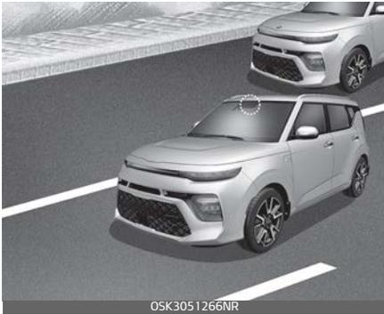
Dirt, snow, or foreign substances on the lens may adversely affect the sensing performance of the sensor.
