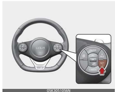
3. Push the SET- button, and release it at the desired speed. The cruise set indicator light will illuminate. Release the accelerator pedal at the same time. The
