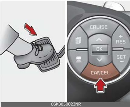
Smart Cruise Control is temporarily canceled when the brake pedal is depressed or the CANCEL button is pressed.
