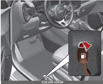
If the fuel filler door does not open because ice has formed around it, tap lightly or push on the door to break the ice and release the door. Do not pry on the door. If necessary, spray around the door with an approved de-icer fluid (do not use radiator anti-freeze) or move the vehicle to a warm place and allow the ice to melt.
