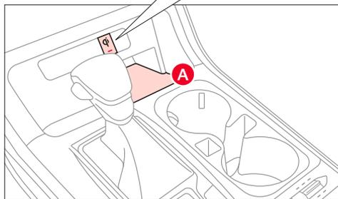
Requires Qi-enabled device or Qi-enabled case
