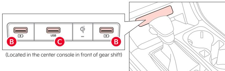
(Located in the center console in front of gear shift)
