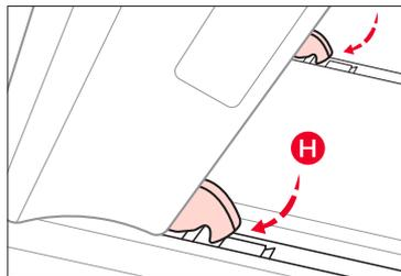
(Hooks highlighted are inserted into channel between bar and white adjustment device)
