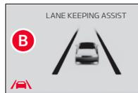
When the front-view camera does **not** detect the lane traveling in, the lanes are not illuminated gray
