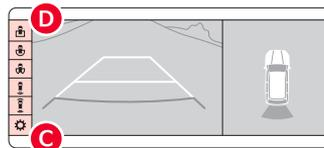
**REMINDER:** The SVM camera is equipped with an optical lens to provide a wider range of vision and may appear different from the actual distance.
