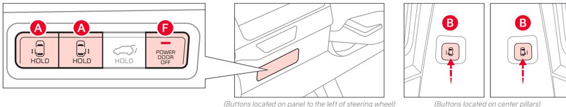
**REMINDER:** If the POWER DOOR OFF button **F** is depressed, the Smart Power Liftgate\* will not operate.
