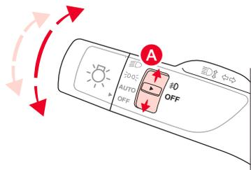
The **One-Touch Lane Change Signal** is activated by briefly pressing the Turn Signal Lever slightly for less than 1 second and then releasing. The lane change signal will blink 3 times.
