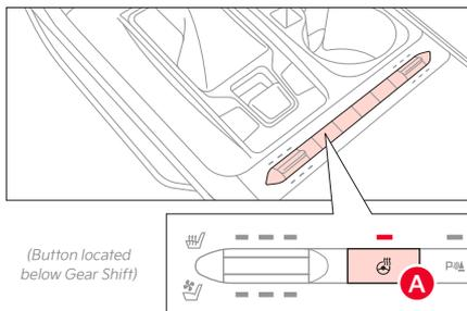
**REMINDER:** If the steering wheel becomes too warm, turn the system off. The heated steering wheel may cause burns even at low temperatures, especially if used for long periods of time.
