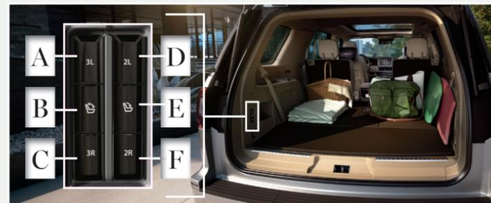
The control buttons are on the left-hand rear quarter trim panel (accessible from the liftgate area).
