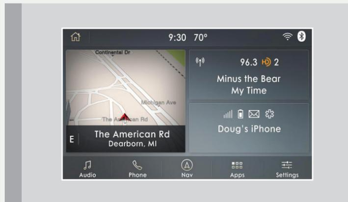
SYNC 3 allows you to interact with a variety of features using the touchscreen and voice commands. The system provides easy use of the system elements like audio, phone, mobile apps and settings.
