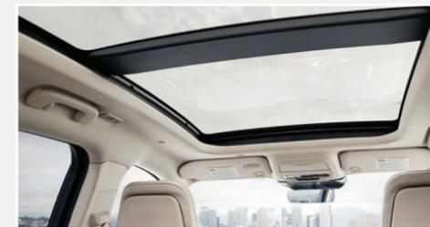
The moonroof controls are on the overhead console and have a one-touch open and close feature. To stop the movement during one-touch operation, press the control a second time.
