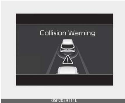
This warning message appears on the LCD display with a warning chime. Additionally, some vehicle system intervention occurs by the engine management system to help decelerate the vehicle.
