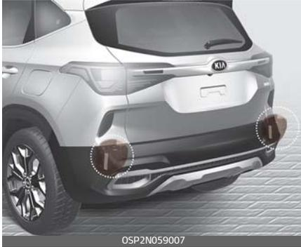
The rear corner radars are the sensors inside the rear bumper for detecting the side and rear areas. Always keep the rear bumper clean for proper operation of the system.
