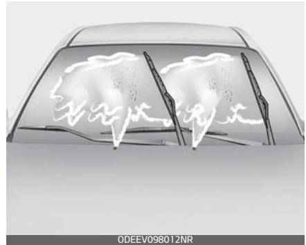
Commercial hot waxes applied by automatic vehicle washes have been known to make the windshield difficult to clean.
