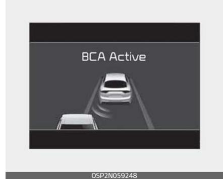
BCA gently applies braking power on the tire that is located in the opposite side of the possibly-colliding point. The instrument cluster will inform the driver of the BCA activation.
