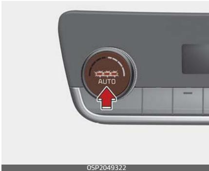
You can control the wind strength in three stages by pushing the AUTO button during automatic operation.
