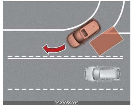
BCW and BCA systems may not operate properly when driving where the road is merging/dividing. In certain instances, the system may not detect the vehicle in the next lane.
