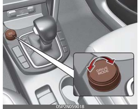
The Drive mode is activated by turning the knob.
