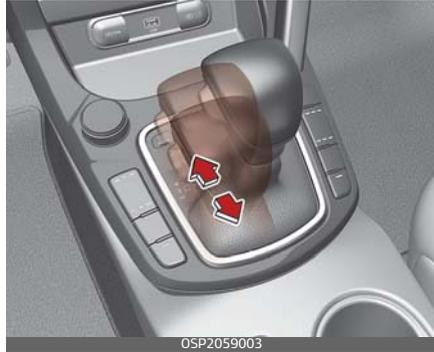
Whether the vehicle is stationary or in motion, sports mode can be selected by pushing the shift lever from the D (Drive) position into the manual gate. To return to D (Drive) range operation, push the shift lever back into the main gate.
