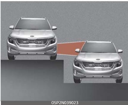
BCW and BCA systems may not operate properly when driving where the heights of the lanes are different.
