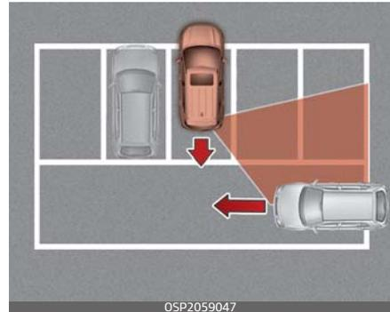
If the vehicle is parked rearward and the radar sensor detects the another vehicle in the rear area of the parking space, the system can warn or control braking. Always pay attention to your surroundings while driving.
