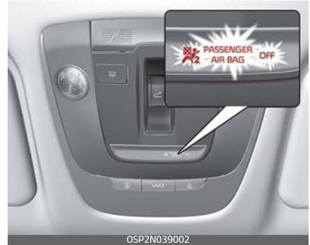
The ODS is designed to detect the presence of a properly-seated front passenger and determine if the passenger's front air bag should be enabled (may inflate) or not. Only the front passenger front air bag is controlled by the ODS.
