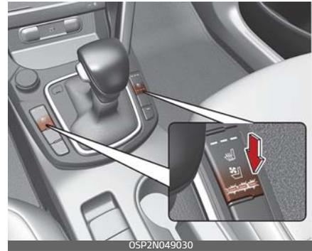
The temperature setting of the seat changes according to the switch position.
