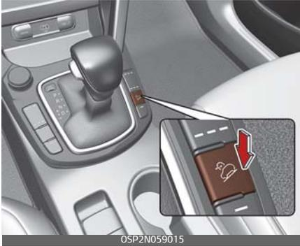
The Downhill Brake Control (DBC) feature assists the driver to descend down a steep hill without having to depress the brake pedal.
