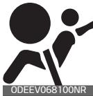
If the air bag warning light is illuminated for more than 6 seconds after the ENGINE START/STOP button has been turned to the ON position, or if it illuminates during vehicle operation, an SRS component may not be functioning properly and you should have your vehicle checked by an authorized Kia dealer.
