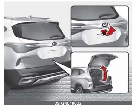
To open the liftgate, press the handle and pull it up.
