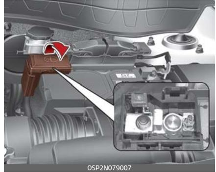
3. Replace the fuse with a new one of the same rating.
