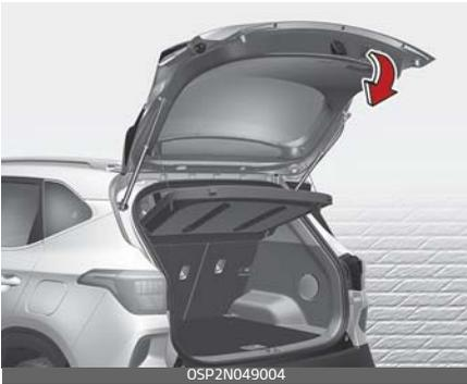
1. Lower and push down the liftgate firmly.
