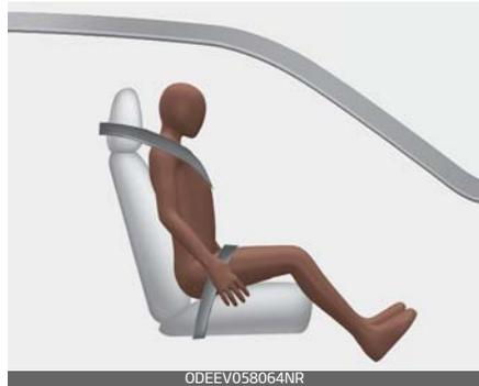
When an adult is seated in the front passenger seat, if the PASSENGER AIR BAG "⊗" indicator is on, change the ENGINE START/STOP button to the OFF position and ask the passenger to sit properly (sitting upright with the seatback in an upright position, centered on the seat cushion with their seat belt on, legs comfortably extended and their feet on the floor). Restart the vehicle and have the person remain in that position. This will allow the sys-
