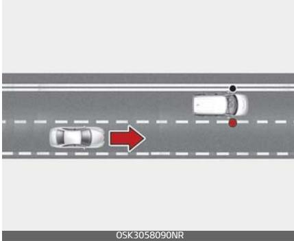
Blind-Spot Collision Warning system will alert you when it detects a vehicle is approaching in an adjacent lane at a high rate of speed.
