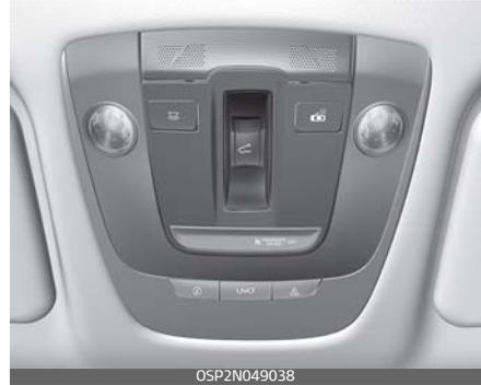
The sunroof can only be opened, closed, or tilted when the ignition switch is in the ON position.
