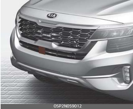
Dirt, snow, or foreign substances on the sensor cover or sensor may adversely affect the sensing performance of the sensor.
