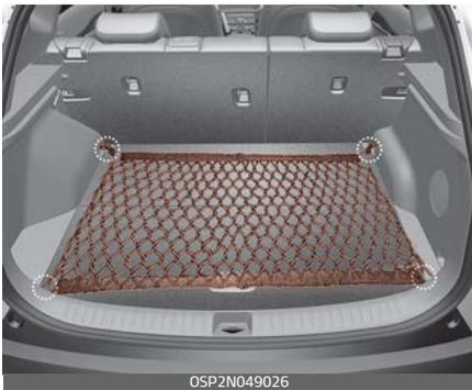
To keep items from shifting in the cargo area, you can use the 4 holders located in the cargo area to attach the luggage net<sup>\*1</sup>.
