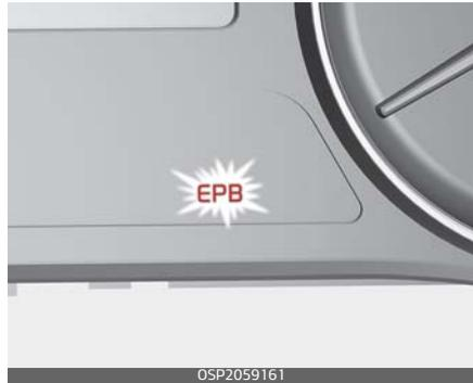
If the EPB malfunction indicator remains on, comes on while driving, or does not come on when the ENGINE START/STOP button is changed to the ON position, this indicates that the EPB may have malfunctioned.
