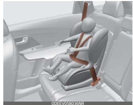
A forward-facing child seat provides restraint for the child's body with a harness. Keep children in a forward-facing child seat with a harness until they reach the top height or weight limit allowed by your child restraint's manufacturer.
