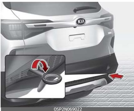
1. Open the liftgate, and remove the towing hook from the tool case.
