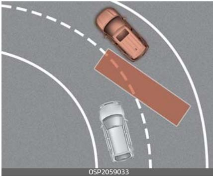
BCW and BCA systems may not operate properly when driving on a curved road. In certain instances, the system may not detect the vehicle in the next lane.
