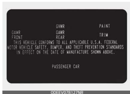
This label shows the maximum allowable weight of the fully loaded vehicle. This is called the GVWR (Gross Vehicle Weight Rating). The GVWR includes the weight of the vehicle, all occupants and cargo.
