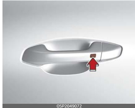
Pressing the button of the front driver side door handles with all doors (and liftgate) closed and any door unlocked, locks all the doors (and liftgate). If all doors (and liftgate) and engine hood are closed, the hazard warning lights will blink once and the chime will sound once to indicate.
