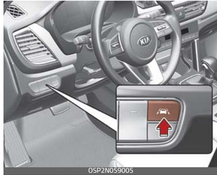
With the ignition switch in the ON position, LKA turns on automatically. The indicator (
