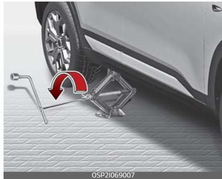
Before removing the wheel lug nuts, make sure the vehicle is stable and that there is no chance for movement or slippage.
