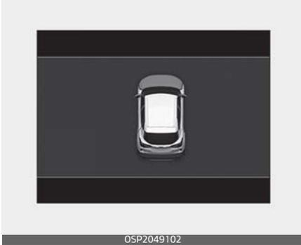
The warning chime will operate when the vehicle is being driven above 2 mph (3 km/h) with the hood open.
