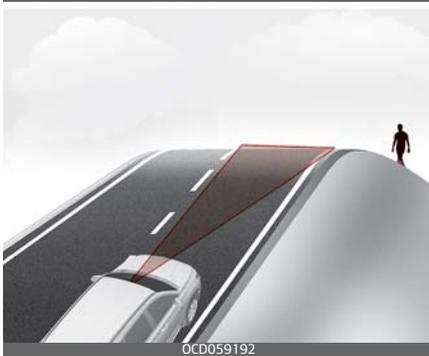
The performance of FCA decreases while driving upward or downward on a slope, not recognizing the vehicle in front in the same lane. It may unnecessarily produce the warning message and the warning alarm, or it may not produce the warning
