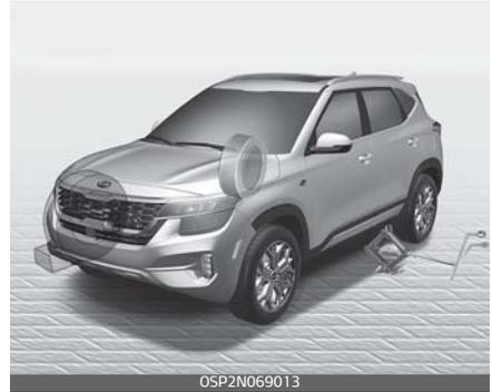
5. Block both the front and rear of the wheel that is diagonally opposite from the jack position.
