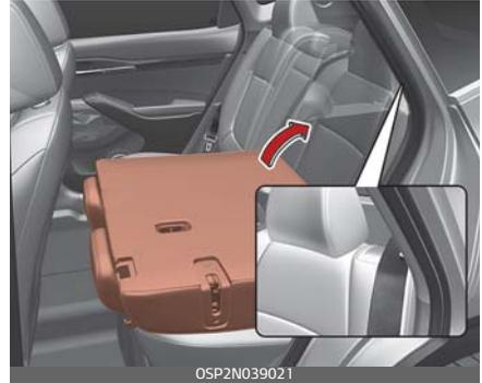
1. To use the rear seat, lift and pull the seatback backward. Pull the seatback firmly until it clicks into place. Make sure the seatback is locked in place. When you return the seatback to its upright position, always be sure it has locked into position by pushing on the top of the seatback.
