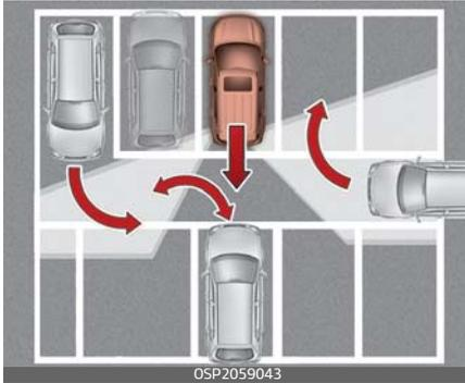
RCCW/RCCA may not operate properly when the vehicle is in a complex parking environment.
