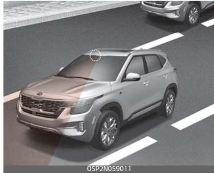
The front view camera is a sensor detecting the lane. If the sensors are covered with snow, rain or foreign substance, the system may temporarily be canceled and not work properly. The system may also be canceled due to the degradation of the sensor's detection performance. Always keep the sensor clean.
