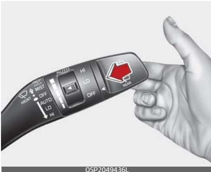
1. Move the wiper speed control switch to In OFF position.
