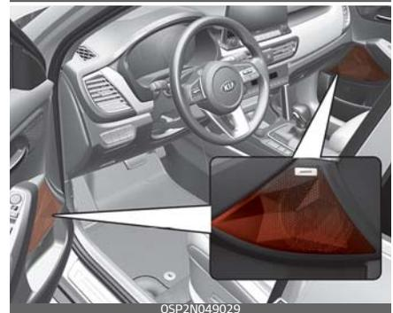
When the headlamp light is on, the ambient light is on at the same time Sound mood lamps (if equipped) could be set in the audio or infotainment menu.
