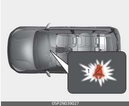
If you start to drive without the passenger seat belt fastened or you unfasten the seat belt when you drive 12 mph (20 km/h) and faster, the warning light will blink and warning chime will sound for approximately 100 seconds. When the passenger seat belt is unfastened during driving, the warning light will illuminate when the speed is under 12 mph (20 km/h). When the speed is 12 mph (20 km/h) and faster, the warning light will blink and warning chime will sound for approximately 100 seconds.
