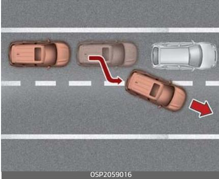
When driving in stop-and-go traffic, and a stopped vehicle in front of you merges out of the lane, FCA system may not immediately detect the new vehicle that is now in front of you. In this case, you must maintain a safe braking distance, and if necessary, depress the brake pedal to reduce your driving speed in order to maintain a safe distance.
