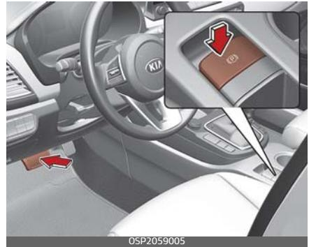
Releasing the parking brake with EPB switch,
