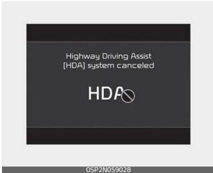
If you keep your hands off the steering wheel even with the hands-off warning on, the steering assist and Smart Cruise Control will be temporarily released automatically.
