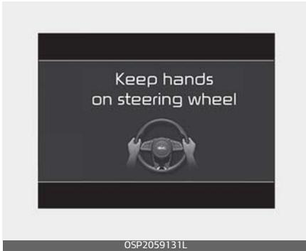
If you keep your hands off the wheel while driving with LFA is in steering assist mode, the hands-off warning will be triggered.
