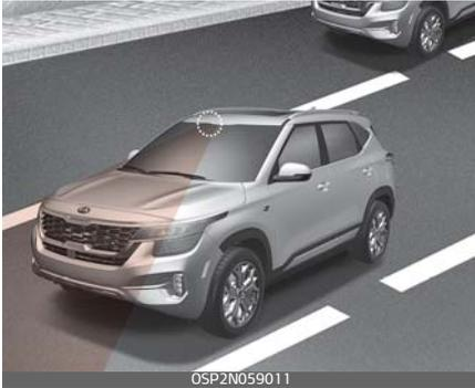
When the system detects the vehicle straying from its lane, it alerts the driver with a visual and audible warning, while applying a counter-steering torque, trying to prevent the vehicle from moving out of its lane.
