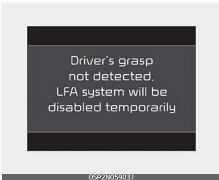
If the driver keeps hands off the wheel even with the hands-off warning on, the steering assist is temporarily deactivated automatically.
