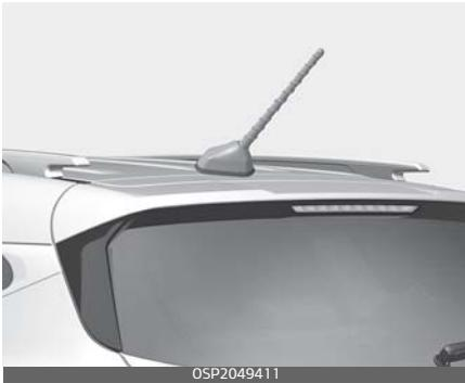
Your vehicle uses a roof antenna to receive AM or/and FM broadcast signals. This antenna pole is removable. To remove the roof antenna pole, turn it counterclockwise.
