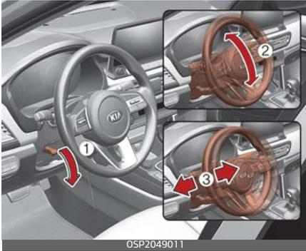
1. To change the steering wheel angle, pull down the lock release lever (1).
