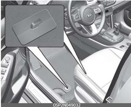
When using a floor mat on the front floor carpet, make sure it attaches to the floor mat anchor(s) in your vehicle. This keeps the floor mat from sliding forward.
