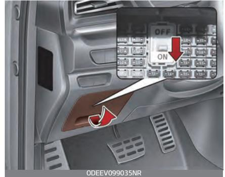
Always set the fuse switch to the ON position before using the vehicle. If you move the switch to the OFF position, some items such as audio and digital clock must be reset and transmitter (or smart key) may not work properly. When the switch is Off, the caution indicator will be displayed on the instrument cluster.
