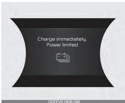
When the high voltage battery level reaches around 3% or less, this warning message is displayed.
