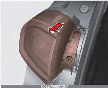
5. Disconnect the rear combination lamp connector.
