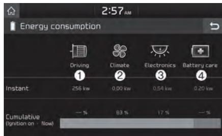
1. 'Driving' shows the total power and energy consumption of the driving motor's driving energy and regenerative energy.
