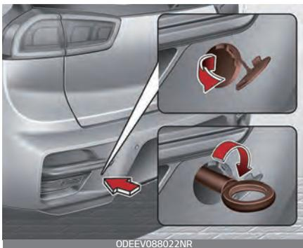
2. Remove the hole cover pressing the upper (front) / lower (rear) part of the cover on the bumper.
