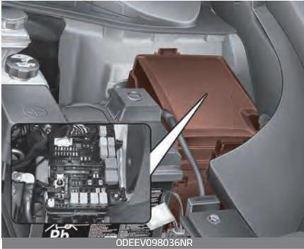
3. Check the removed fuse; replace it if it is blown. To remove or insert the fuse, use the fuse puller in the motor compartment fuse panel.
