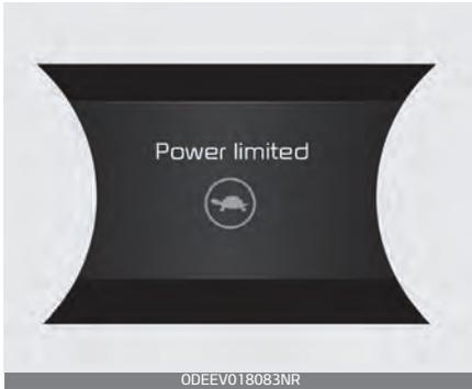
In the following cases, this warning message is displayed when the vehicle's power is limited for safety.
