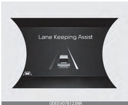
If the vehicle moves out its lane because steering torque for assistance is not enough, the lane indicator will blink.
