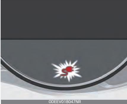
When the charging connector is not connected properly, reconnect the charging cable to charge it again.
