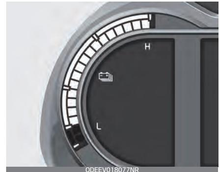
The SOC gauge shows the charging status of the high voltage battery. "L (Low)" position on the indicator indicates that there is not enough energy in the high voltage battery. "H (High)" position indicates that the driving battery is fully charged.
