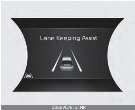
To see LKA screen on the LCD display in the cluster, Tab to the Driving Assist mode (
