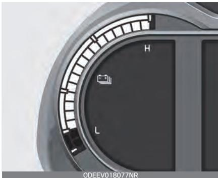
"L (Low)" position on the indicator indicates that there is not enough energy in the high voltage battery.
