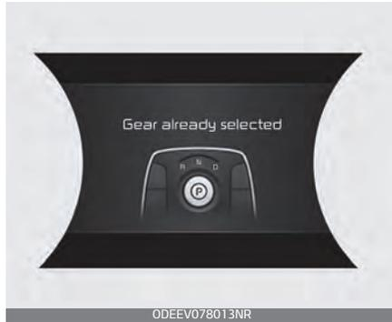
The message appears on the LCD display when the selected gear button is pressed again.
