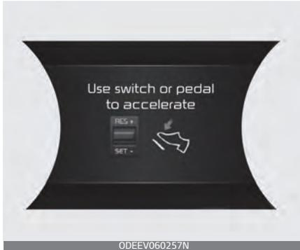
When Highway Driving Assist is operating, your vehicle will stop if the vehicle ahead of you stops. Also, if the vehicle ahead of you starts moving within 30 seconds after the stop, your vehicle will start as well. In addition, after the vehicle has stopped and 30 seconds have passed, the 'Use switch or pedal to accelerate' message will appear on the cluster. Depress the accelerator pedal or push the RES+, SET- switch or CANCEL button to start driving.
