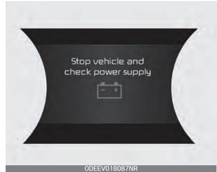
This warning message is displayed when a failure occurs in the 12 V power supply system.
