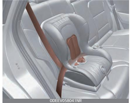
Since all passenger seat belts move freely under normal conditions and only lock under extreme or emergency conditions (emergency locking mode), you must manually pull the seat belt all the way out to shift the retractor to the "automatic locking" mode to secure a child restraint.
