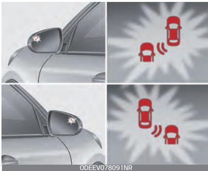
If a vehicle is detected within the boundary of the function, a warning light will illuminate on the outer side view mirror.
