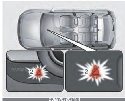
If a front passenger continues not to fasten the seat belt and the vehicle is driven 6 mph (9 km/h) or more but less than 12 mph (20 km/h), the warning light will stay illuminated.
