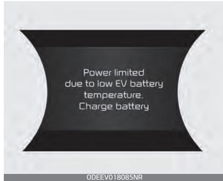
The warning message is displayed to protect the electric vehicle system when you turn off or turn on the vehicle while outside temperature is low. If the high voltage battery charging level is low and parked outside in low temperature for a long time, vehicle power could be limited. Charging the battery before driving, increases the battery temperature, and helps increase power.
