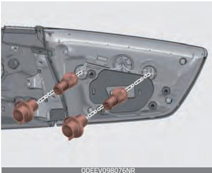
4. Remove the bulb from the socket by pressing it in and rotating it counter-clockwise until the tabs on the bulb align with the slots in the socket. Pull the bulb out of the socket.
