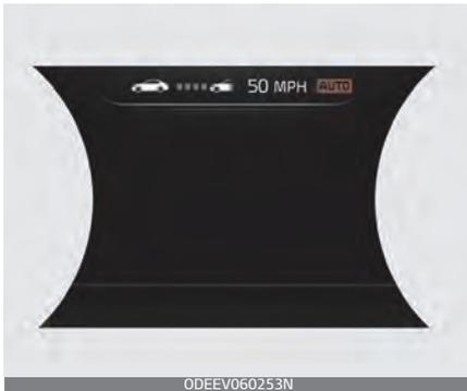
If temporary deceleration is required in the standby state and Navigation-based Smart Cruise Control is operating, the green
