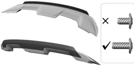
**Note:** The Gurney flap comes with longer size bolts to install it onto the rear spoiler. **Do not use the longer size bolts without the Gurney flap attached or damage to the spoiler may occur.**
