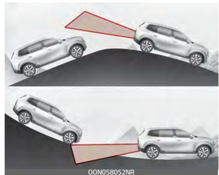
The BCW and BCA may not operate properly when driving on a slope. In certain instances the BCW/BCA may not detect the vehicle in the next lane.
