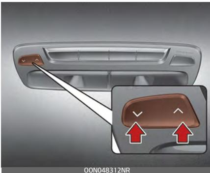
1. To change the rear air temperature, press the button (∧) for warmer air or press the button (∨) for cooler air.
