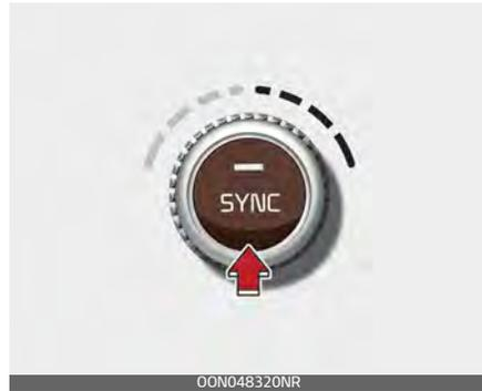
1. Press the "SYNC" button to adjust the driver and front/rear passenger side temperature, fan speed and air flow direction equally. The front and rear passenger side temperature, fan speed and air flow direction will be set to the same temperature, fan speed and air flow direction as the driver's side.
