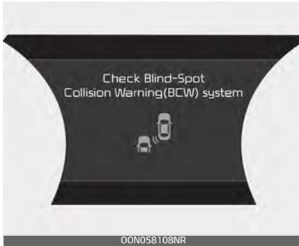
If there is a problem with the BCW, a warning message will appear and the light on the switch will turn off. The BCW will turn off automatically. The BCA will not operate also if the BCW turns off due to malfunction. In this case, have your vehicle inspected by an authorized Kia dealer.
