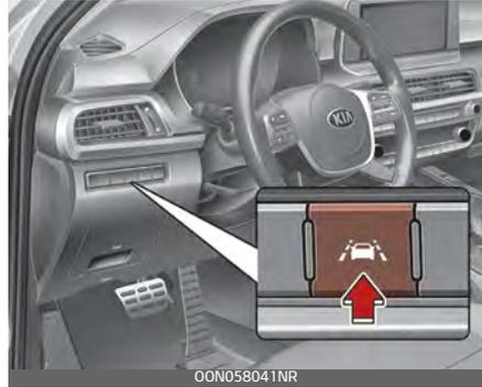
To activate/deactivate the LKA, with the ENGINE START/STOP button in the ON position, take the following steps:
