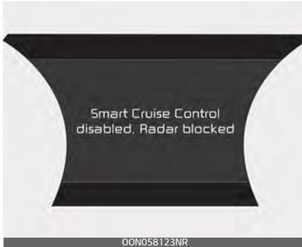
When the sensor lens cover is covered with dirt, snow, or debris, the SCC operation may stop temporarily. If this occurs, a warning message will appear on the LCD display. Remove any dirt, snow, or debris and clean the radar sensor lens cover before operating the SCC.
