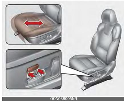
1. Press the front portion of the switch to raise the cushion extension, or the rear portion of the switch to lower it.
