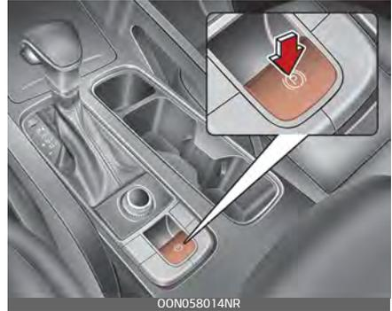
Releasing the parking brake with EPB switch,
