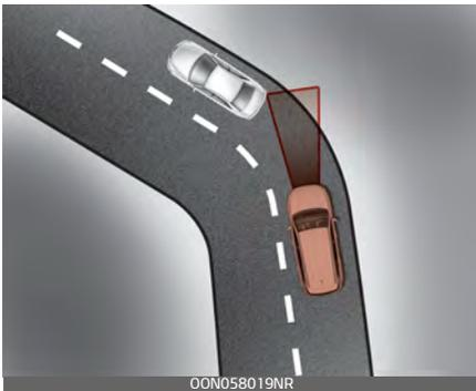
The Smart Cruise Control system may not detect a moving vehicle in your lane, and then your vehicle could accelerate to the set speed.
