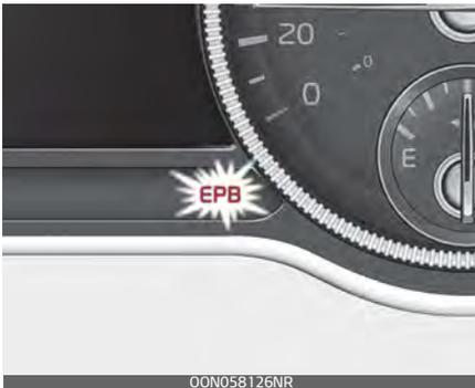
If the EPB malfunction indicator remains on, comes on while driving, or does not come on when the ENGINE START/STOP button is
