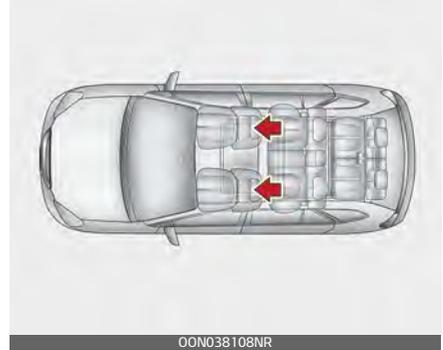
The headrest not only provides comfort for the driver and front passenger, but also helps protect the head and neck in the event of a rear collision.
