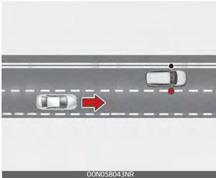
The Lane Change Assist feature will alert you when a vehicle is approaching in an adjacent lane at a high rate of speed. If the driver activates the turn signal when the system detects an oncoming vehicle, the system sounds an audible alert.
