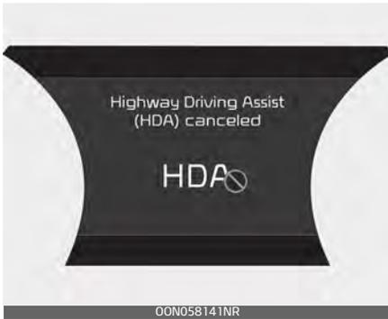
If you keep your hands off the steering wheel even with the hands-off warning on, the steering assist and Smart Cruise Control will be temporarily released automatically. If you activate the Smart Cruise Control system with the HDA released, the steering assist will re-start.
