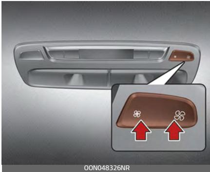
1. Adjust the fan speed by pressing the rear fan speed control button.
