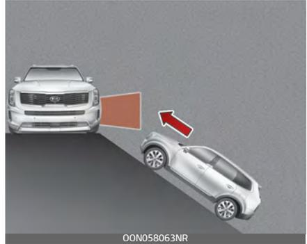
The RCCW/RCCA may not operate properly when the vehicle is on/near a slope.
