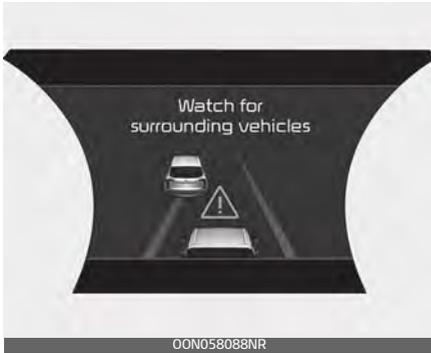
If the vehicle ahead (vehicle speed: less than 20 mph (30 km/h) moves to the next lane, the warning chime will sound and a message will appear. Adjust your vehicle speed for vehicles or objects that can suddenly appear in front of you by depressing the brake pedal according to the road and driving conditions.
