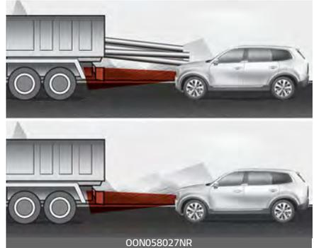
If the vehicle in front of you has cargo that extends rearward from the cab, or when the vehicle in front of you has higher ground clearance, additional special attention is required.
