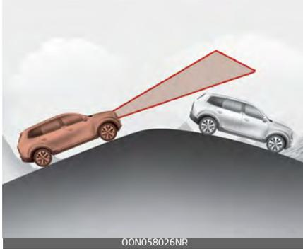
During uphill or downhill driving, the SCC may not immediately detect a moving vehicle in your lane, and may cause your vehicle to accelerate to the set speed.
