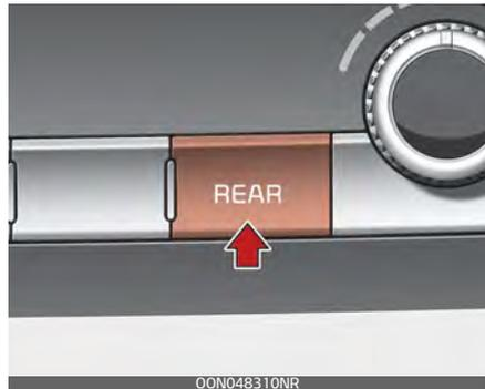
1. Press the REAR button located on the front climate control panel and press the rear fan speed control button on the audio or multi-media screen.
