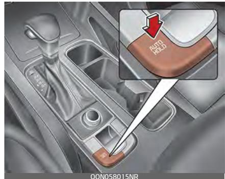
Before the Auto Hold will engage, the driver's door and engine hood must be closed and the liftgate must be closed.
