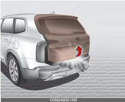
During power opening and closing if the power liftgate is blocked by an object or part of the body, the power liftgate will detect the resistance.
