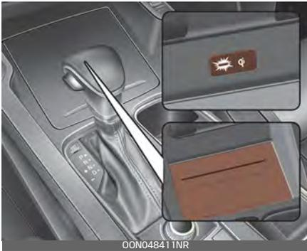
Firmly close all doors, and turn the vehicle on. To start wireless charging, place the smart phone capable of wireless charging on the wireless charging pad.
