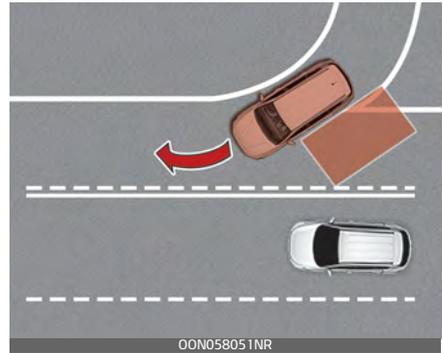
The BCW and BCA may not operate properly when driving where the road is merging/dividing. In certain instances the BCW/BCA may not detect the vehicle in the next lane. Always pay attention to road and driving conditions, while driving.
