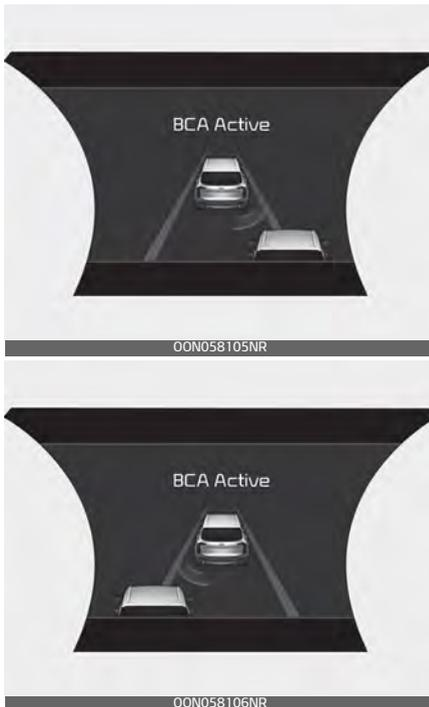
The BCA may apply braking power, when an approaching vehicle is detected within a certain distance next to/behind your vehicle.
