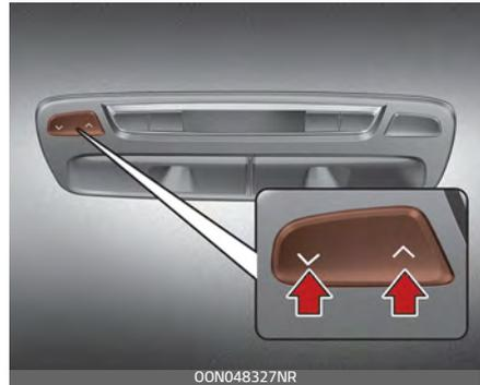
2. To change the temperature, press the button (∧) for warmer air or press the button (∨) for cooler air.
