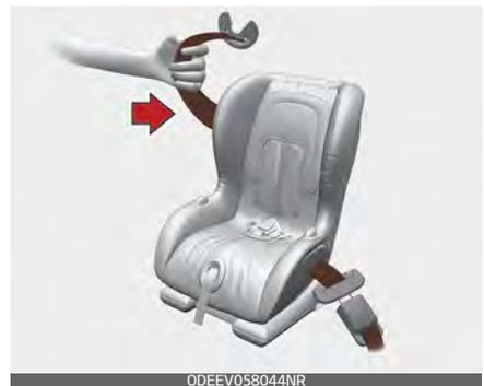
5. Remove as much slack from the belt as possible by pushing down on the CRS while feeding the shoulder belt back into the retractor.
