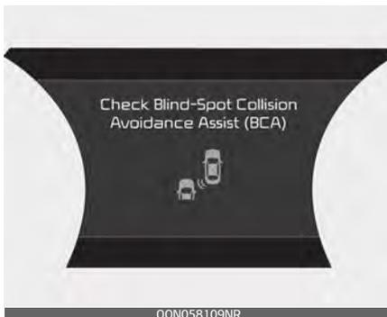
If there is a problem with the BCA, a warning message will appear. The BCA will turn off automatically. The BCW will still operate even if the BCA turns off due to malfunction. In this case, have your vehicle inspected by an authorized Kia dealer.
