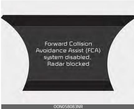
In this case, a warning message ("Forward Collision-Avoidance Assist (FCA) system disabled. Radar blocked") will appear to notify the driver.
