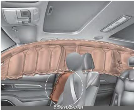
\* The actual air bags in the vehicle may differ from the illustration. Side and/or curtain air bags are designed to inflate when an impact is detected by side collision sensors depending on several factors, including the severity of impact resulting from a side impact collision.
