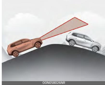
The FCA performance may be limited while driving upward or downward on a slope, and may not recognize the vehicle in front in the same lane. It may produce the warning message and the warning alarm prematurely, or it may not produce the warning message and the warning alarm at all.
