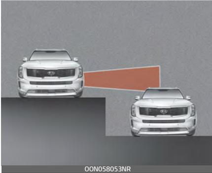
The BCW and BCA may not operate properly when driving where the heights of the lanes are different.
