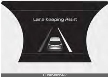
When the conditions below are met, the LKA will be enabled to assist steering.
