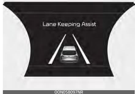
If the speed of the vehicle is over 40 mph (64 km/h) and the LKA detects lane markers, the color changes from gray to white.
