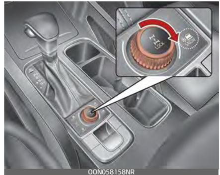
You can switch from DRIVE MODE to SNOW mode by turning the knob.
