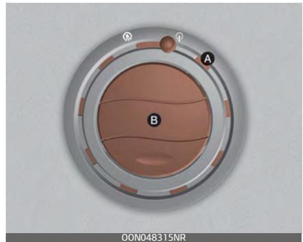
: Air discharged from [A] spreads over a wider area.
