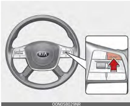
2. Accelerate to the desired speed. The SCC speed can be set as follows:
