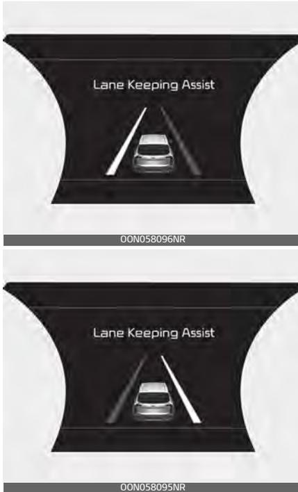
If the vehicle moves out its lane because steering torque for assistance is not enough, the line indicator of deviation direction will blink and the warning sound is provided.
