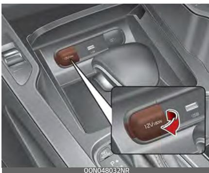
The devices should draw less than 10 amps with the vehicle on.
