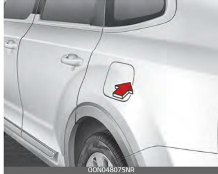
If the fuel filler lid does not open because ice has formed around it, tap lightly or push on the lid to break the ice and release the lid. Do not pry on the lid. If necessary, spray around the lid with an approved de-icer fluid (do not use radiator anti-freeze) or move the vehicle to a warm place and allow the ice to melt.
