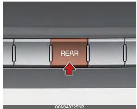
1. Press the REAR button located on the front climate control panel and press the rear fan speed control button on the audio or multimedia screen.
