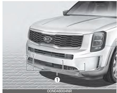
The sensing range and objects detectable by the sensors (1) are limited. Whenever moving while using the parking distance warning, pay as much attention to what is in
