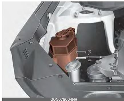
Do not remove the radiator cap when the engine and radiator are hot. Scalding hot coolant and steam may blow out under pressure which may result in serious injury.
