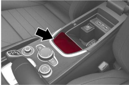
If the smartphone is removed from the charging pad, the charge will immediately be interrupted.
