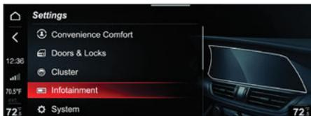
To access the “Infotainment” function, select it by turning and pressing the Rotary Pad or touching the display.
