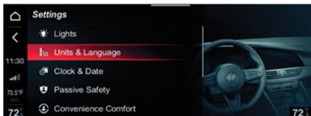
To access the "Units & Language" function and the respective sub-menus, select the option by turning and pressing the Rotary Pad or touching the screen.
