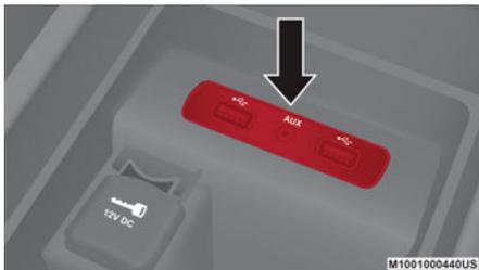
When a device is connected to the AUX port, the system will play the connected device's audio through the vehicle speakers.
