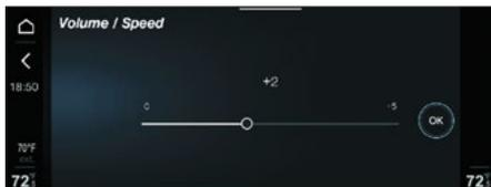
The adjustment can be set to six positions: "Off", system is turned off, and five sensitivity levels.
