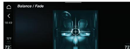
The adjustment can be set to 19 positions, from -9 to +9; 0 is the balance position.
