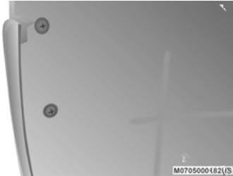
**Inner Wheel Liner Fasteners**
