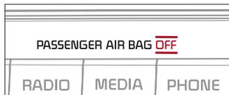
If the system determines that the airbag should not be deployed, the "PASSENGER AIR BAG OFF" light will illuminate.
