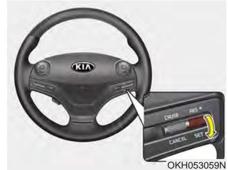
3. Lever must be moved down (to **SET-**) prior to setting any desired speed. The Set speed in the instrument cluster will illuminate. Release the accelerator at the same time. The desired speed will automatically be maintained.
