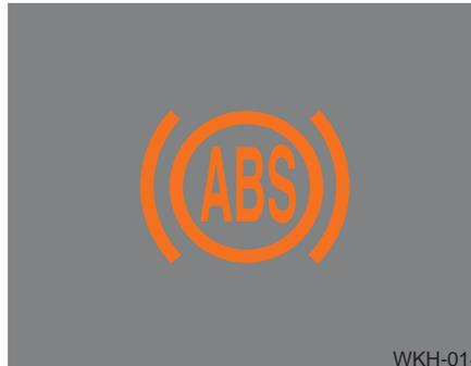
The ABS warning light will stay on for approximately 3 seconds after the Engine Start/Stop button is ON. During that time, the ABS will go through self-diagnosis and the light will go off if everything is normal. If the light stays on, you may have a problem with your ABS but your regular brakes will work normally. Contact an authorized K900 Kia dealer as soon as possible.
