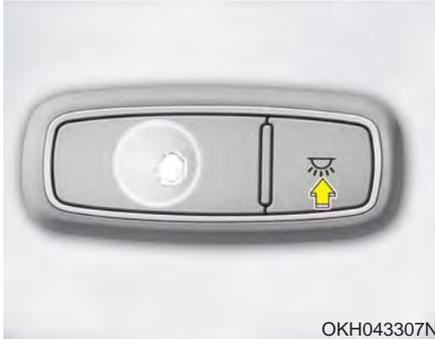
Press the button to turn the rear lamp on. To turn the lamp off, press the button again.
