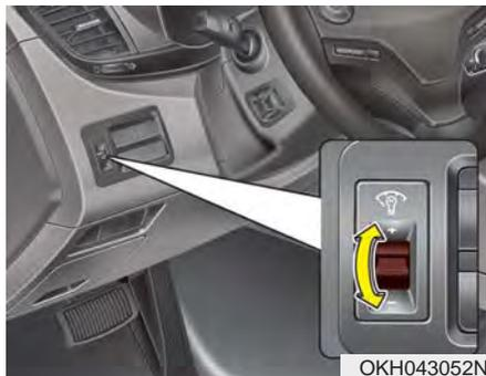
The brightness of the instrument panel illumination can be adjusted by pressing the illumination control buttons (“+” or “-”) when the Engine Start/Stop Button is ON or the tail lights are turned on.
