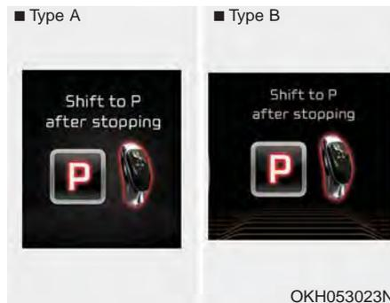
5.When you shift into [P], if the vehicle speed is high, warning will be illuminated. Stop the vehicle at safe area and shift into [P].
