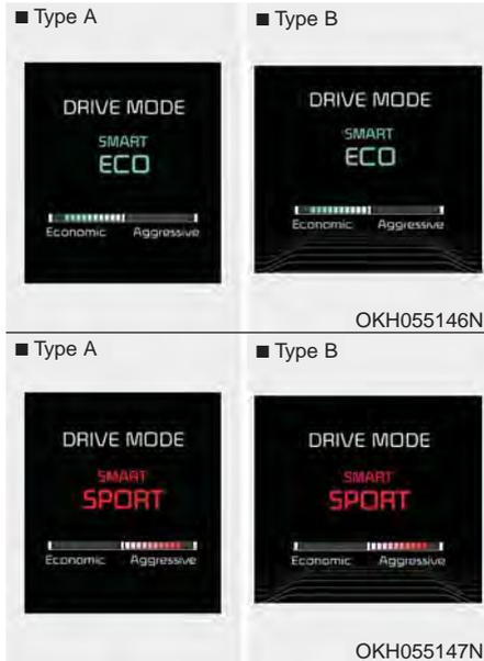
Once the SMART MODE is selected by pressing the DRIVE MODE button, and the DRIVE MODE indicator screen is selected by pressing the trip computer button on the steering wheel, the driving style gauge bar will show up at the bottom of screen and visualize current style of driving.
