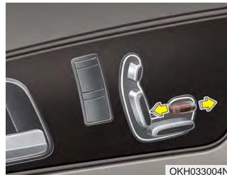
Push the control switch forward or backward to move the seat cushion to the desired length. Release the switch once the seat cushion reaches the desired length.
