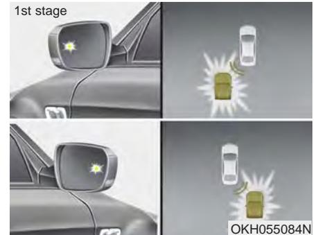
If a vehicle is detected within the boundary of the system, a warning light will illuminate on the outside rearview mirror and the head up display.
