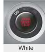
To turn off the engine (START/STOP position) or vehicle power (ON position), press the ENGINE START/STOP button with the shift lever in the P (Park) position. When you press the ENGINE START/STOP button without the shift lever in the P (Park) position, the ENGINE START/STOP button will not change to the OFF position but to the ACC position.
