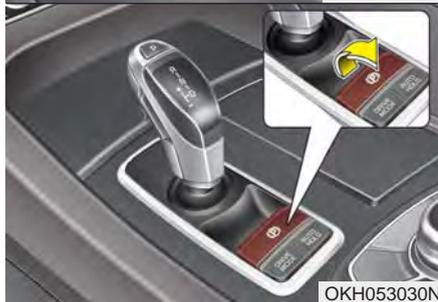
To apply the EPB (electric parking brake):
