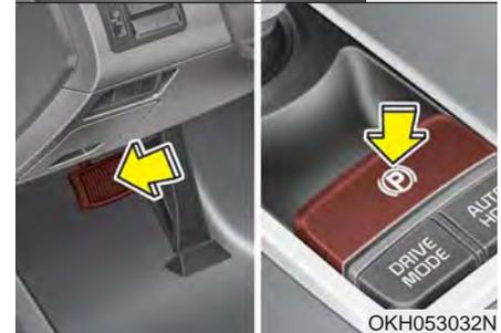
To release the EPB (electric parking brake), press the EPB switch in the following condition:
