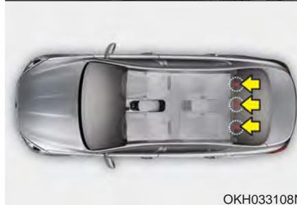
Child restraint hook holders are located on the package tray.
