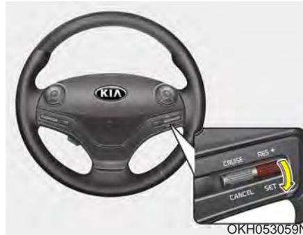
3. Lever must be moved down (to SET-) prior to setting any desired speed. The set speed and vehicle to vehicle distance on the LCD screen will illuminate.
