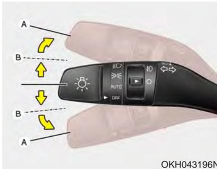
The Engine Start/Stop Button must be ON position for the turn signals to function. To turn on the turn signals, move the lever up or down (A). The green arrow indicators on the instrument panel indicate which turn signal is operating.
