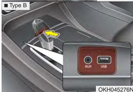
If your vehicle has an aux and/or USB(universal serial bus) port or iPod® port, you can use an aux port to connect audio devices and a USB port to plug in a USB, and an iPod® port to plug in an iPod®.
