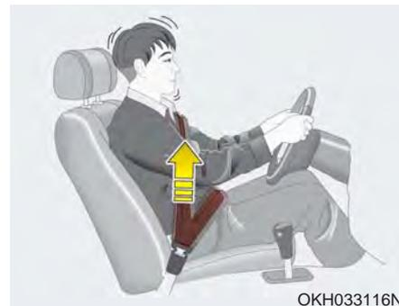
The pre-active seat belt activates only when the passenger is wearing his/her seatbelt. It will activate and pull the seat belt into tighter contact against the occupant's body if a collision is detected or during certain driving maneuvers.
