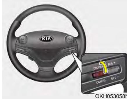
1. Move the lever up (to **CRUISE**), to turn the system on. The **CRUISE** indicator light will illuminate.
