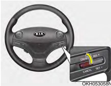
1. Move the lever up (to CRUISE), to turn the system on. The CRUISE indicator light in the instrument cluster will illuminate.
