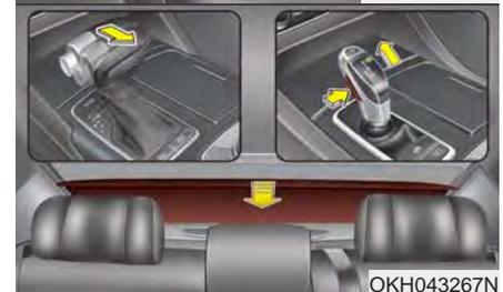
To raise the rear curtain, depress the button. To lower the rear curtain, depress the button again.
