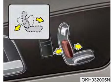
Push the control switch forward or backward to move the seatback to the desired angle. Release the switch once the seat reaches the desired position.
