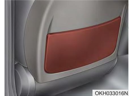
The seatback pocket is provided on the back of the front passenger's and driver's seatbacks.
