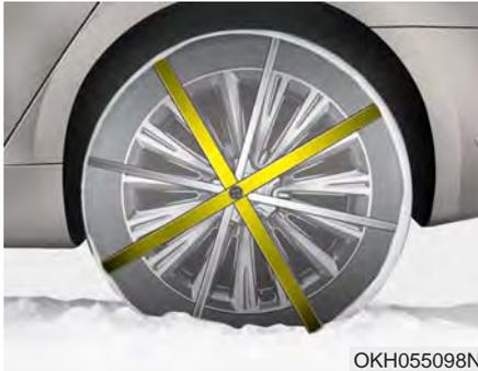
Since the sidewalls of radial tires are thinner, they can be damaged by mounting some types of snow chains on them. Therefore, the use of snow tires is recommended instead of snow chains. Do not mount tire chains on vehicles equipped with aluminum wheels; snow chains may cause damage to the wheels. If snow chains must be used, use the AutoSock® (fabric snow chain). Damage to your vehicle caused by improper snow chain use is not covered by your vehicle manufacturers warranty.
