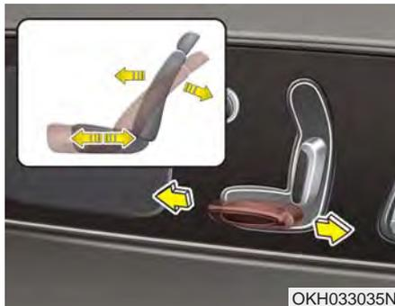
Push the control switch forward or backward to move the seat to the desired position. Release the switch once the seat reaches the desired position.
