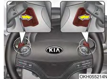
The paddle shifter is available when the shift lever is in the D (Drive) position or the sports mode.
