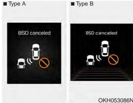
The message will appear to notify the driver if there are foreign substances on the rear bumper or it is hot near the rear bumper. The light on the switch and the system will turn off automatically.
