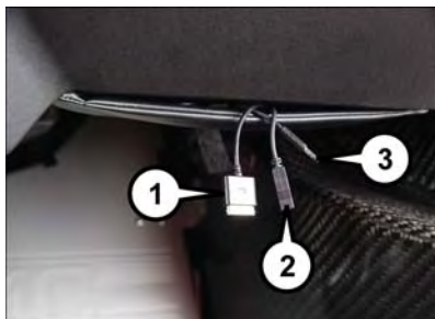
Source Media Cables
