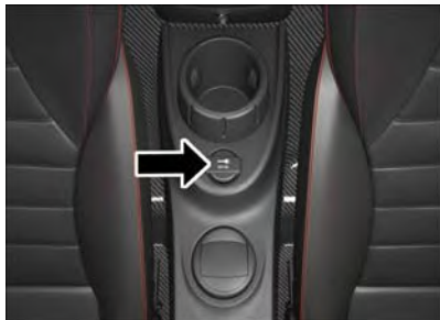
Rear Power Outlet
