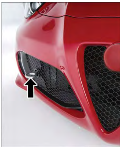
Front Tow Eye Installed
