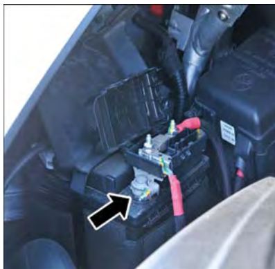
Positive (+) Battery Post
