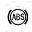
This light monitors the Anti-Lock Brake System (ABS). The light will turn on when the ignition is cycled to the ON/RUN position and may stay on for as long as four seconds.
