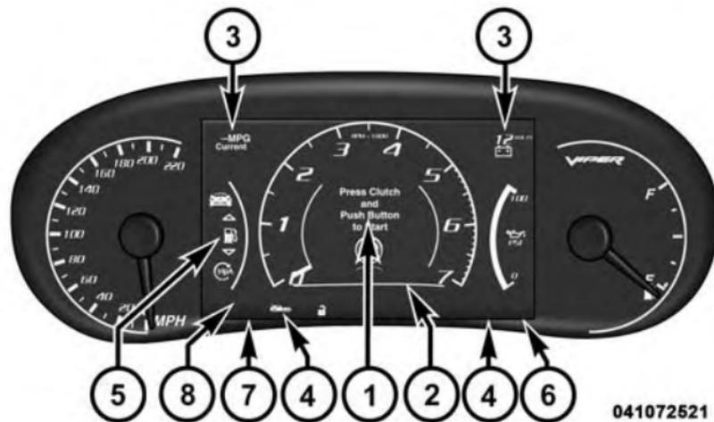
The EVIC displays are located in the center portion of the cluster and consists of the following sections:
