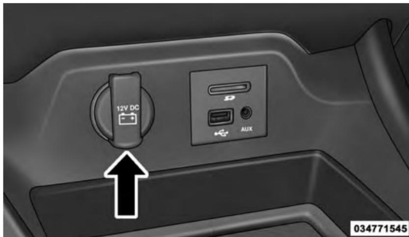
**NOTE:** Do not exceed the maximum power of 160 Watts (13 Amps) at 12 Volts. If the 160 Watt (13 Amp) power rating is exceeded the fuse protecting the system will need to be replaced.
