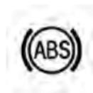
The “Anti-Lock Brake Warning Light” will turn on and stay on briefly as a bulb check when the ignition is first turned on. If the light does not turn on during starting, have it repaired promptly.
