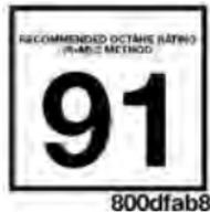
The 8.4L engine is designed to meet all emissions regulations and provide excellent fuel economy and performance when using high-quality premium unleaded gasoline with an octane rating of 91 or
