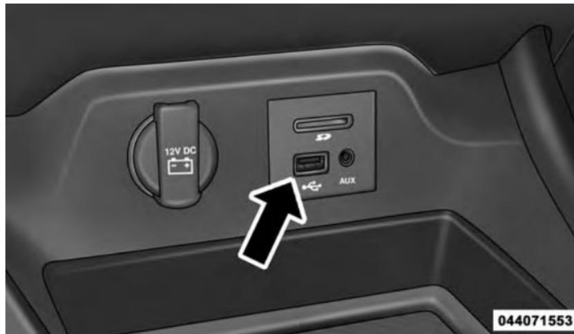
This feature allows an iPod® or external USB device to be plugged into the USB port.
