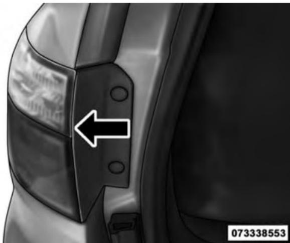
4. Twist socket counter clockwise and remove from lamp.
