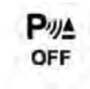
When the ParkSense switch is pressed to disable the system, the instrument cluster will display the “PARKSENSE OFF” message for approximately five seconds. Refer to “Electronic Vehicle Information Center (EVIC)” in “Understanding Your Instrument Panel” for further information. When the shift lever is moved to REVERSE and the system is disabled, the EVIC will display the “PARKSENSE OFF” message for as long as the vehicle is in REVERSE.
