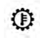
This light indicates that there is excessive transmission fluid temperature that might occur with severe usage such as trailer towing. It may also occur when operating the vehicle in a high torque converter slip condition, such as 4-wheel-drive operation (e.g., snow plowing, off-road operation). If this
