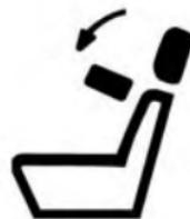
Press the power folding switch located on the instrument panel to fold the head restraints.
