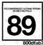
This engine is designed to meet all emissions regulations and provide satisfactory fuel economy and performance when using high-quality unleaded gasoline having an octane range of 87 to 89. The manufacturer recommends the use of 89 octane for optimum performance. The use of premium gasoline is not recommended, as it will not provide any benefit over regular gasoline in these engines.
