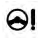
If the “POWER STEERING SYSTEM OVER TEMP” message and a icon are displayed on the EVIC screen, it indicates that extreme steering maneuvers may have occurred, which caused an over temperature condition in the power
