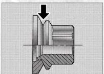
Dual wheel models require a special heavy-duty lug nut tightening adapter (included with the vehicle) to correctly tighten the lug nuts. Also, when it is necessary to remove and install dual rear wheels, use a proper vehicle lifting device.
