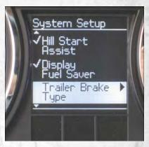
Press the SELECT button and then press the UP or DOWN buttons until the proper Trailer Brake Type appears on the screen.
