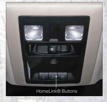
Erase all channels before you begin programming. To erase the channels, place the ignition switch into the ON/RUN position, then press and hold the two outside HomeLink® buttons (I and III) for up 20 seconds or until the red indicator flashes.
