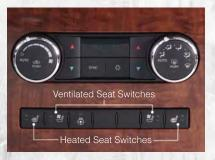
If the High-level setting is selected, the system will automatically switch to Low-level after approximately 60 minutes. The Low-level setting will turn Off automatically after approximately 45 minutes.
