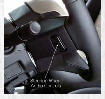
Press the button in the center to select the next preset station (radio) or to change CDs if equipped with a CD Changer.
