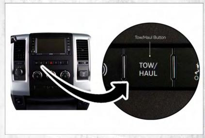
The "TOW/HAUL Indicator Light" will illuminate in the instrument cluster to indicate that TOW/HAUL mode has been activated. Pressing the switch a second time restores normal operation. If the TOW/HAUL mode is desired, the switch must be pressed each time the engine is started.
