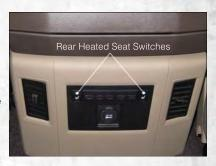
If the High-level setting is selected, the system will automatically switch to Low-level after approximately 60 minutes. The Low-level setting will turn Off automatically after approximately 45 minutes.
