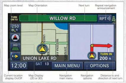
After starting route guidance, the system calculates the route and announces: "Follow the arrows on the display." You will receive navigation recommendations by voice messages and screen displays.
