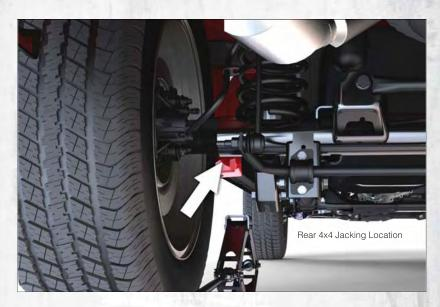
Connect the jack tube extension and wheel wrench.
