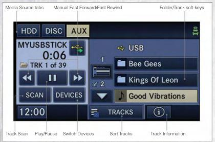
Press the "RADIO/MEDIA" hard key until the media source tabs are displayed at the top of the screen. Select the source by touching the "HDD," "DISC," or "AUX" media source soft-key tab.
