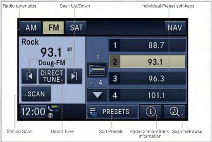
To access Radio Mode, touch the "RADIO" hard-key on the left side of the faceplate, then touch the "AM," "FM" or "SAT" soft-key at the top of the screen to select the band.
