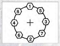
It is recommended that wheel stud nuts be kept torqued to specifications at all times. Torque wheel stud nuts to specifications at each lubrication interval.
