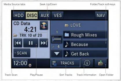
Press the "MEDIA" hard key to display the media source tabs at the top of the screen. Select the source by touching the "HDD," "DISC," or "AUX" media source soft-key tab.
