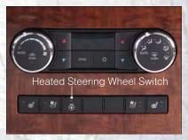
Once the heated steering wheel has been turned on, it will operate for approximately 58 to 70 minutes before automatically shutting off. The heated steering wheel can shut off early or may not turn on when the steering wheel is already warm.
