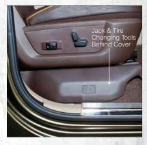
Remove the jack and tools by removing the wing bolt and sliding the assembly from under the seat.
