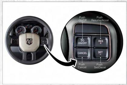
The speed control switches are located on the steering wheel.
