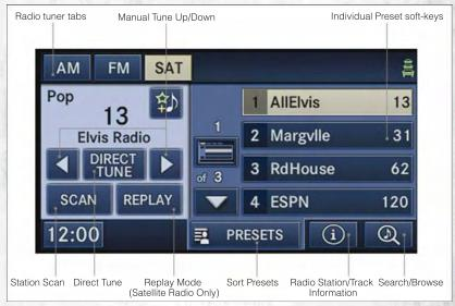
To access Radio Mode, touch the "RADIO/MEDIA" hard-key on the left side of the faceplate repeatedly until AM/FM/SAT appears at the top of the screen, then touch the "AM," "FM" or "SAT" soft-key to select the band.
