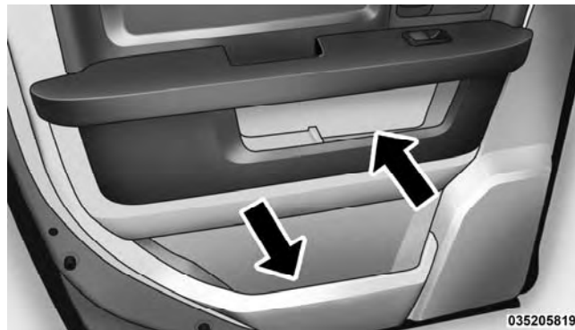
Rear Door Storage
