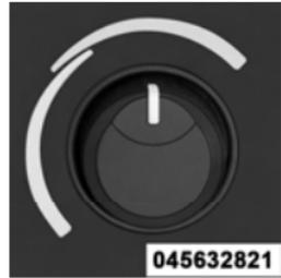
The rotary knob at the center of the control panel controls the temperature of the interior air. You can choose your degree of comfort by rotating the knob. The coldest temperature setting is to the extreme left (blue region) and the warmest setting is to the extreme right (red region) of the rotation.
