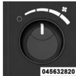
The rotary knob on the left of the control panel is the Blower Control. Turn the knob clockwise to one of the four positions to obtain the blower speed you desire. To turn the blower off, turn the knob to the far left position.
