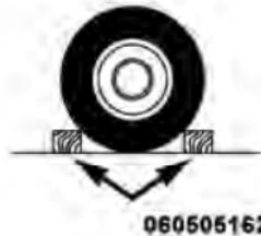
6. Block both the front and rear of the wheel diagonally opposite the jacking position. For example, if the right front wheel is being changed, block the left rear wheel.
