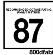
These engines are designed to meet all emissions regulations, and provide excellent fuel economy and performance when using high quality unleaded “regular” gasoline having an octane rating of 87. The use of premium gasoline is not recommended, as it will not provide any benefit over regular gasoline in these engines.
