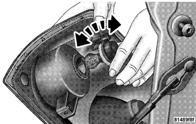
4. Pull bulb straight out of socket.
