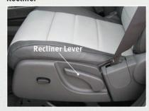
Lift the recliner lever located on the outboard side of the seat, lean back and release at the desired position.
