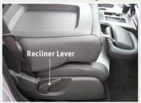
The front passenger seat can be folded flat to allow for extended cargo space. Pull up on the recliner lever to fold down the seatback.
