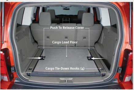
• The panel in the load floor is reversible for added utility. One side features a plastic lined tray which can hold a variety of items. The maximum load capacity of the load floor is 400 lbs (181 kg).
