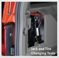
The scissor-type jack and tire changing tools are located in the left rear trim panel behind the second row seat.
