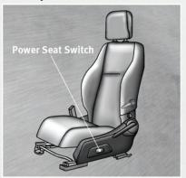
The power seat switch is located on the outboard side of the seat near the floor. Use the switch to move the seat up, down, forward, rearward, or to tilt the seat.
