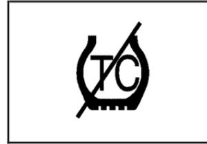
If your vehicle is equipped with the Enhanced Traction System (ETS), this warning light should come on briefly as you start the engine.
