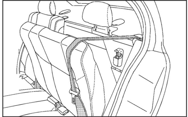
2. Once the handle is pulled, the seatback can be pushed open through the trunk, or pulled open from the inside of the vehicle.
