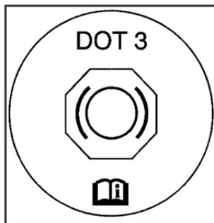
Your brake master cylinder and, on manual transaxle vehicles, the hydraulic clutch use the same reservoir. The reservoir is filled with DOT-3 brake fluid. See *Engine Compartment Overview* on page 5-12 for the location of the reservoir.
