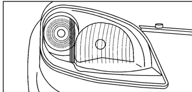
1. Find the aim dot on the lens of the low-beam lamp.
