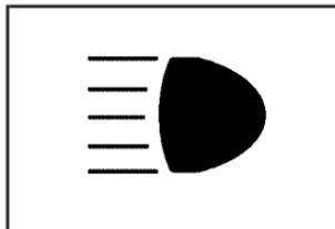
This light will come on when the high-beam headlamps are in use.
