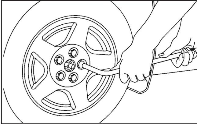
1. If your vehicle is equipped with plastic wheel covers, use the wheel wrench to loosen the plastic wheel nut caps.
