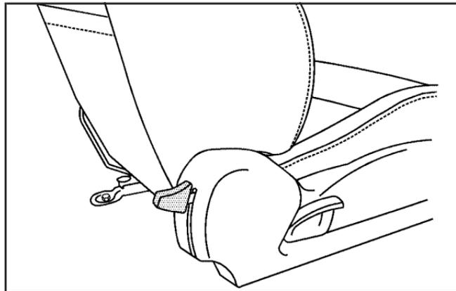
1. Push down the easy entry seat handle located on the rear of the seatback on the outboard side to release the seatback.
