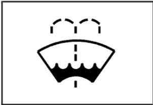
Open the cap with the washer symbol on it. Add washer fluid until the tank is full. See *Engine Compartment Overview* on page 5-12 for reservoir location.
