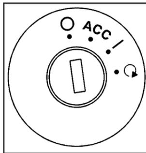
**Notice:** Using a tool to force the key from the ignition switch could cause damage or break the key. Use the correct key and turn the key only with your hand. Make sure the key is all the way in. If it is, turn the steering wheel left and right while you turn the key hard. If none of this works, then your vehicle needs service.
