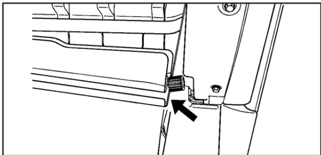
2. Tilt the glove box door down by squeezing on each side of the glove box until the door can be lowered from its track. Lower the glove box door.
