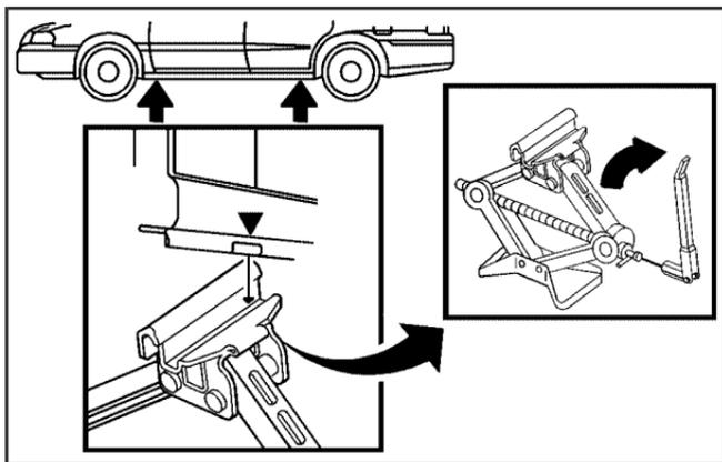
4. Position the jack lift head at the jack location nearest the flat tire. The front location is about 8 inches (20 cm) rearward from the front wheel opening. The rear location is about 4 inches (10 cm) forward of the rear wheel opening.
