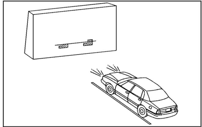
5. Turn the vertical aiming screw until the headlamp beam is aimed to the horizontal tape line. The top edge of the cut-off should be positioned at the bottom edge of the horizontal tape line.
