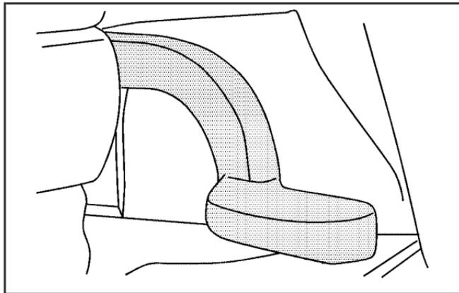
To tilt the wheel, pull down the lever. Then move the wheel to a comfortable position, pull up the lever to lock the wheel in place.
