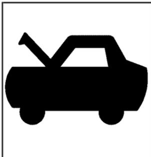
1. Pull the interior hood release lever with this symbol on it. It is located under the instrument panel on the driver's side of the vehicle.
