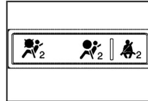
The passenger sensing system will turn off the right front passenger's frontal airbag under certain conditions. The driver's airbag and the side airbags (if equipped) are not part of the passenger sensing system.
