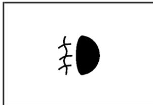
If equipped, the fog lamps light will come on when the fog lamps are in use.
