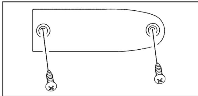
1. Remove the two screws from the face of the back-up lamp.
