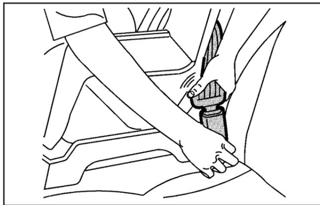
3. Buckle the belt. Make sure the release button is positioned so you would be able to unbuckle the safety belt quickly if you ever had to.
