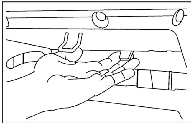
3. Open the passenger compartment air filter door by reaching through the opening in the back of the glove box and raising the tab until the door can be opened downward.
