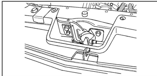
2. Then go to the front of the vehicle and push the secondary hood release lever to the left. It is located under the front center of the hood toward the driver's side of the vehicle.
