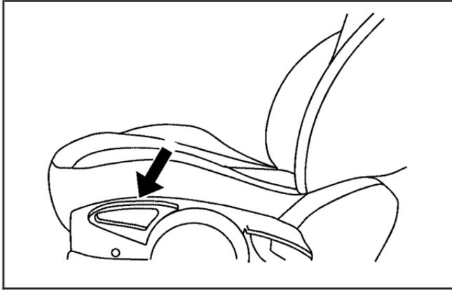
The driver's seat height adjuster is located on the outboard side of the seat.
