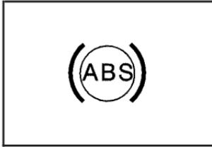
If your vehicle is equipped with the anti-lock brake system, the light will come on when your engine is started and may stay on for several seconds. That is normal.
