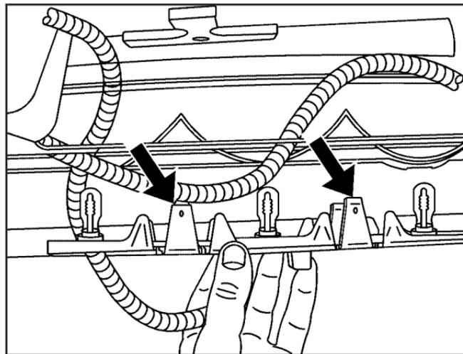
4. Pull the bulb assembly down to access the bulbs.
