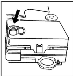
The remote positive terminal is located under a red tethered cap on the engine compartment fuse block. Lift the cap to access the terminal.
