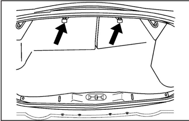
1. Open the trunk and pull one or both of the small handles located in the center of the trunk.
