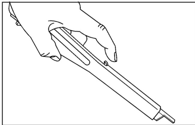
Press the button and then pull on the end of the wheel wrench to extend the handle.
