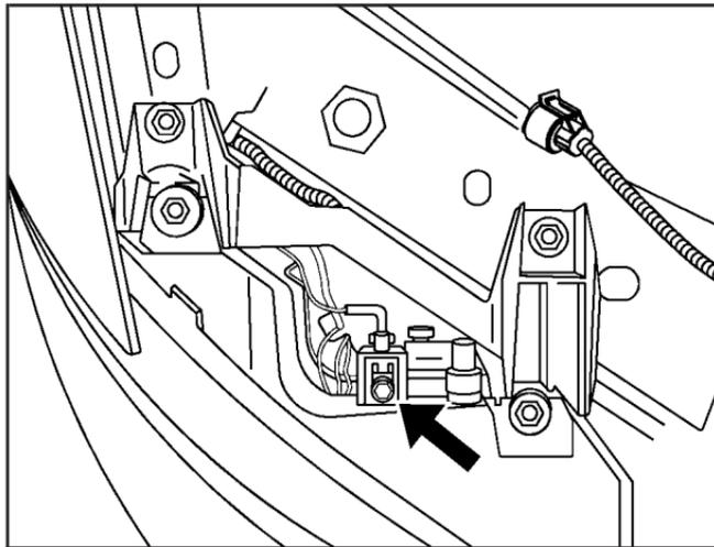
The adjustment screw can be turned with a 6 mm socket wrench.
