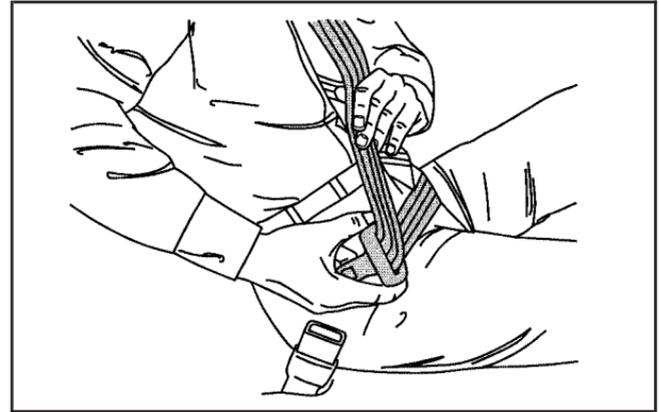
If the belt stops before it reaches the buckle, tilt the latch plate and keep pulling until you can buckle it. Pull up on the latch plate to make sure it is secure. If the belt is not long enough, see *Safety Belt Extender* on page 1-35.
