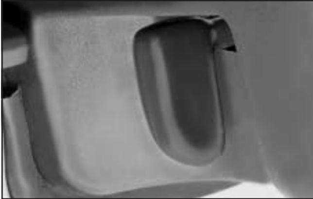
The lever that allows you to tilt the steering wheel is located on the left side of the steering column. To tilt the wheel, hold the wheel and pull the lever. Then move the wheel to a comfortable position and release the lever to lock the wheel in place.
