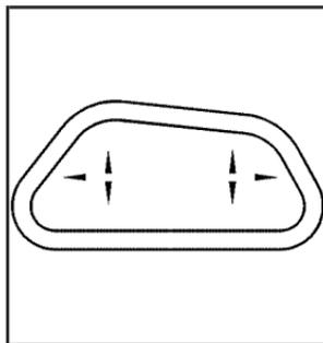
Your vehicle may have this feature. If it does, the six-way power seat control is located on the outboard sides of the driver's and front passenger's seats.
