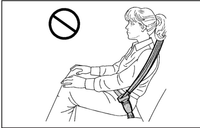
The lap portion of the belt should be worn low and snug on the hips, just touching the child's thighs. This applies belt force to the child's pelvic bones in a crash.
