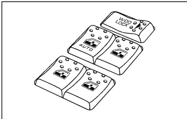
Switches on the driver's door armrest control each of the windows when the ignition is in ON, ACCESSORY, or when Retained Accessory Power (RAP) is active. See *Retained Accessory Power (RAP)* on page 2-20 for more information. In addition, each passenger's door has a window switch.
