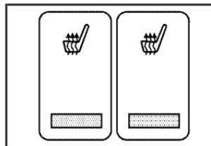
Your vehicle may have heated seats. If it does, the heated seat switches are located in the instrument panel switchbank.
