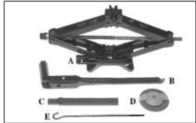
The tools you'll be using include the jack (A), folding wrench (B), extension tube (C), wing nut (D), and J-Hook (E).
