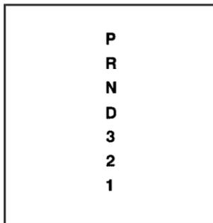
Maximum engine speed is limited when you are in PARK (P) or NEUTRAL (N), to protect driveline components from improper operation.
