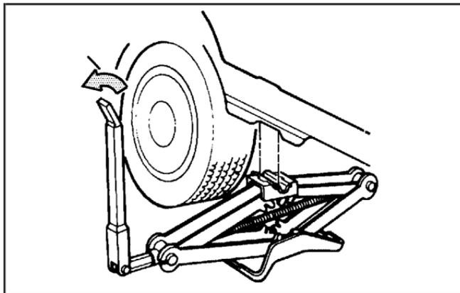
11. Lower the vehicle by attaching the folding wrench to the jack and turning the wrench counterclockwise. Lower the jack completely.
