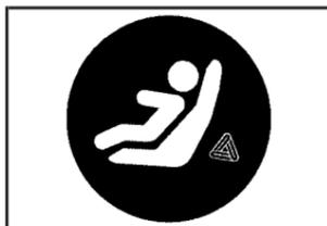
To assist you in locating the lower anchors for this child restraint system, each seating position with the LATCH system has a label on the seatback.
