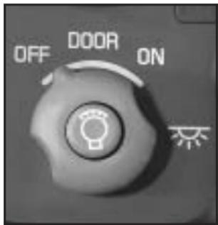
The interior lamp control is located to the left of the steering column, below the exterior lamp control.
