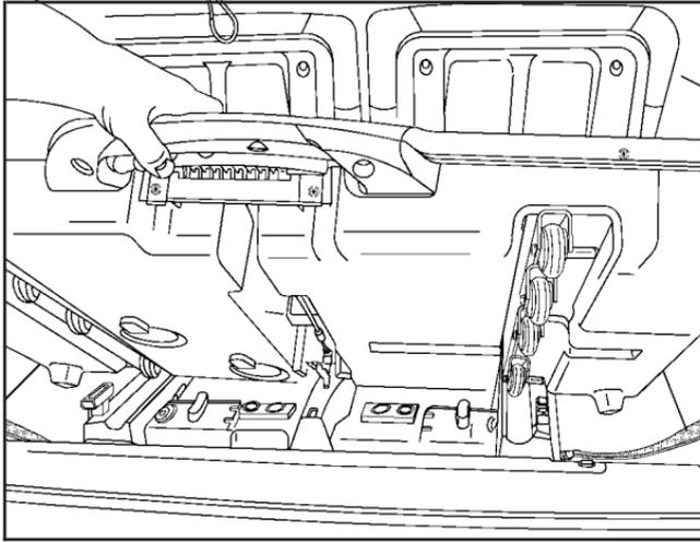
5. Use the handle to lift up on the tray while pulling it towards you. Use your other hand to support and lift the tray from the bottom. Remove the tray from the vehicle.
