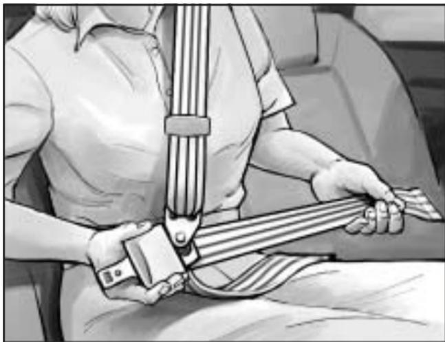
3. To make the lap belt longer, tilt the latch plate and pull it along the belt.
