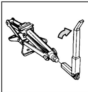
6. Attach the folding wrench to the jack, and turn the wrench clockwise to raise the jack head 3 inches (7.6 cm).
