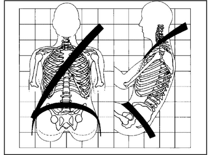
The lap part of the belt should be worn low and snug on the hips, just touching the thighs. In a crash, this applies force to the pelvic bones. And you would be less likely to slide under the lap belt. If you slid under it, the belt would apply force at your abdomen. This could cause serious or even fatal injuries. The shoulder belt should go over the shoulder and across the chest. These parts of the body are best able to take belt restraining forces.
