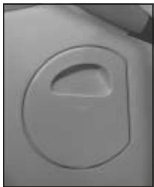
The floor console fuse block is located to the right of the shift lever.
