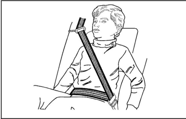
4. Buckle, position and release the safety belt as described in *Rear Seat Passengers* on page 1-25. Make sure that the shoulder belt crosses the shoulder.
