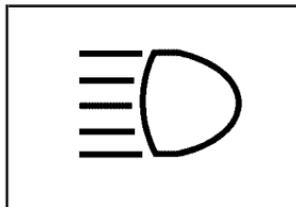
This light will appear on the instrument panel cluster when the high beams are on.
