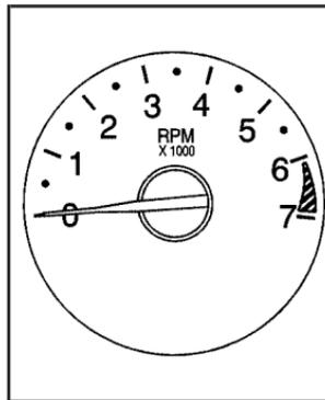
The tachometer located on your instrument panel displays the engine speed in revolutions per minute (rpm).
