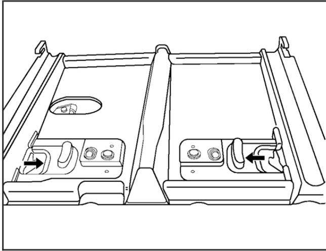
2. Unlock the slide locks from the two rear floor retainers by pushing the button down and pressing them inward.
