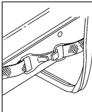
3. Disconnect the tethered ring from the hook and place the tethered ring on the outer edge of the tailgate on each side of the vehicle.
