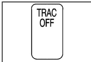
To turn the system off, press the TRAC OFF button located on the instrument panel switchbank.
