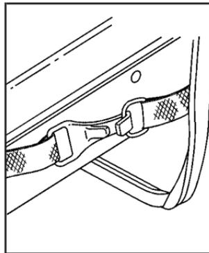
6. Connect the hook to the tethered ring located on each side of the sliding rear convenience tray.
