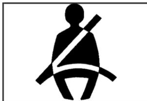
The safety belt light will also come on and stay on for several seconds. If the driver's belt is already buckled, neither the chime nor the light will come on.
