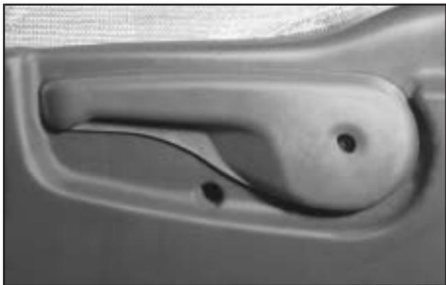
To adjust the seatback, pull up on the recliner lever located on the outboard sides of both the driver's and front passenger's seats. Release the lever to lock the seatback where you want it. Push and pull on the seat to make sure it's locked into position. Pull up on the lever, and the seat will go to its original upright position.
