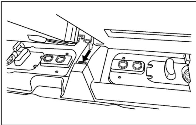
3. Make sure the pin on bottom of the convenience tray fits into the hole on the floor track assembly.
