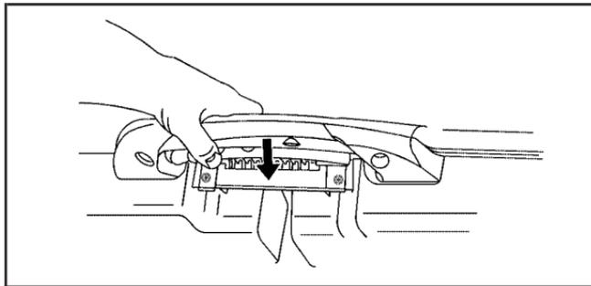
1. Push the release lever located in front of the handle of the tray to release the pin from the floor track assembly.
