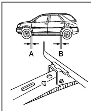
3. Locate the notch (A is 3.0 inches (7.5 cm) from the front tire or B is 5.5 inches (14.0 cm) from the rear tire) in the frame. The notch is located near each wheel in the vehicle's body.
