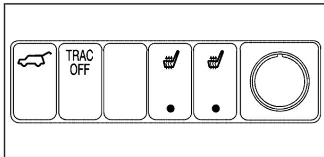
There is an instrument panel switchbank located below the comfort controls. It contains switches or blanks that will vary with the options that are on your vehicle and a cigarette lighter/accessory power outlet.
