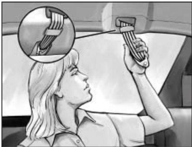
1. Remove the shoulder belt from its stowage location in the roof and pull it all the way down to the lap belt.
