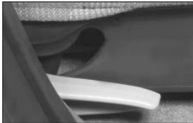
4. Pull the lever, located at the base on the outboard side of the seat, to release the rear latches from the floor pins and flip the seat forward.
