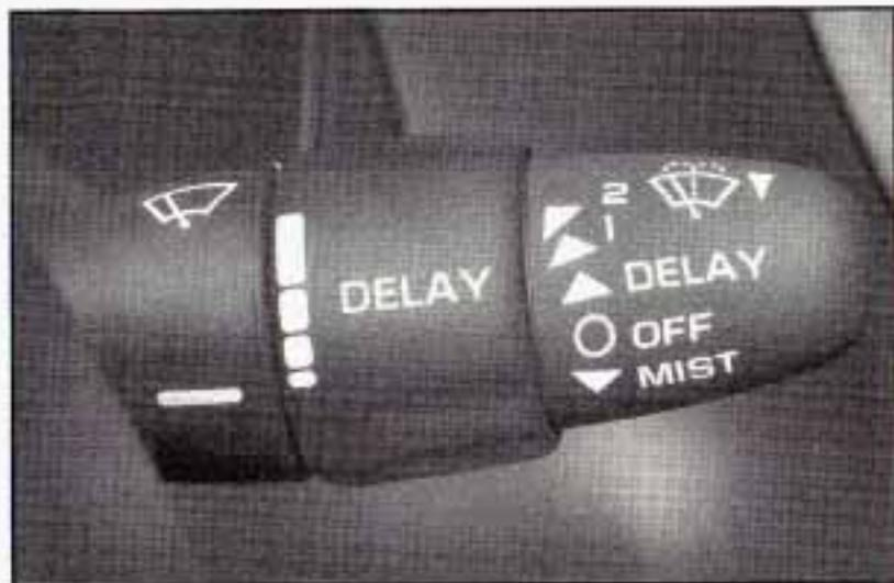
Use this lever located on the right side of the steering wheel to operate the windshield wipers.
