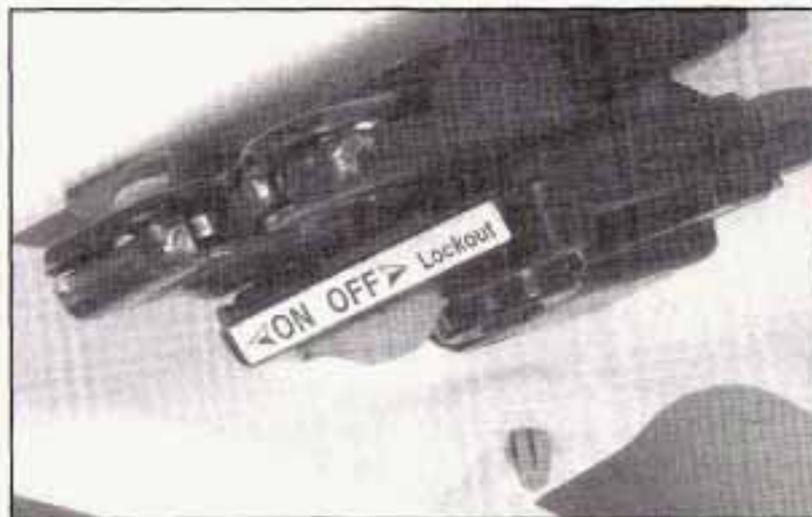
To turn the lockout on, slide the switch all the way to the left to ON. To turn the lockout off, slide the switch all the way to the right to OFF.
