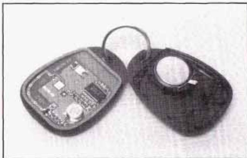
To replace the battery in the transmitter:
