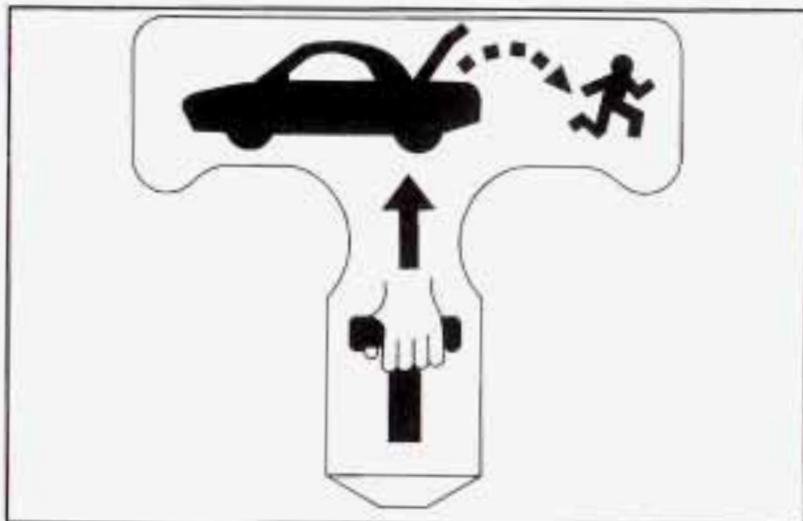
**Notice:** The emergency trunk release handle is not designed to be used to tie down the trunk lid or as an anchor point when securing items in the trunk. Improper use of the emergency trunk release handle could damage it.
