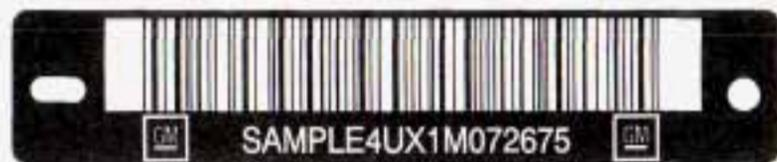
This is the legal identifier for your vehicle. It appears on a plate in the front corner of the instrument panel, on the driver's side. You can see it if you look through the windshield from outside your vehicle. The VIN also appears on the Vehicle Certification and Service Parts labels and the certificates of title and registration.
