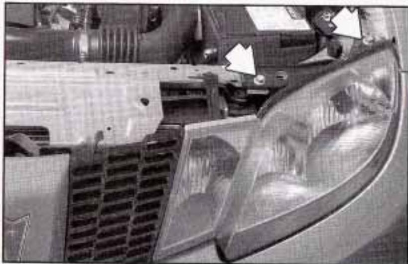
2. Remove the bolts that anchor the headlamp assembly. Pull the headlamp assembly toward the front of the vehicle to access the bulb assembly.
