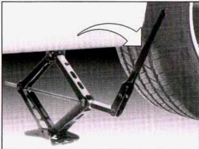
3. Raise the vehicle by turning the jack handle clockwise. Raise the vehicle far enough off the ground for the spare tire to fit underneath the wheel well. Remove all wheel nuts and take off the flat tire.
