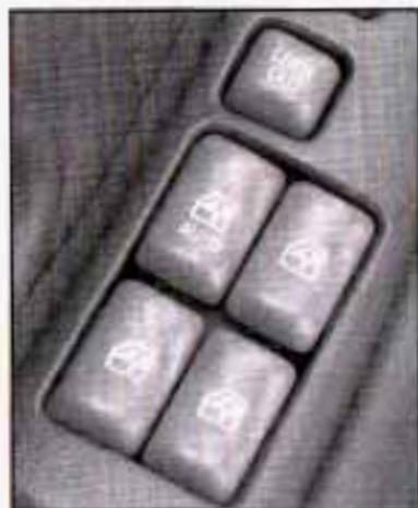
Use the switches on the driver's door armrest to operate each of the windows while the ignition is on or while Retained Accessory Power (RAP) is active. See "Retained Accessory Power (RAP)" under *Ignition Positions* on page 2-19 for more information.
