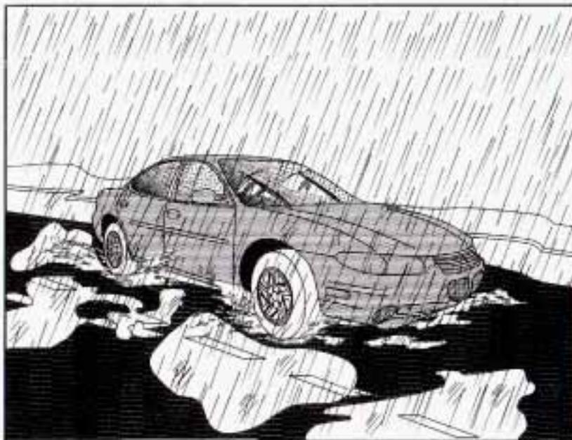
Rain and wet roads can mean driving trouble. On a wet road, you can't stop, accelerate or turn as well because your tire-to-road traction isn't as good as on dry roads. And, if your tires don't have much tread left, you'll get even less traction. It's always wise to go slower and be cautious if rain starts to fall while you are driving. The surface may get wet suddenly when your reflexes are tuned for driving on dry pavement.
