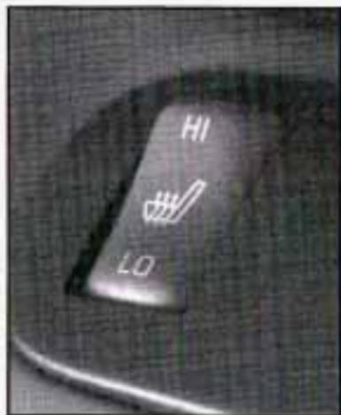
If your vehicle is equipped with this feature, the heated seat switch is located on the center console, behind the open storage bin.
