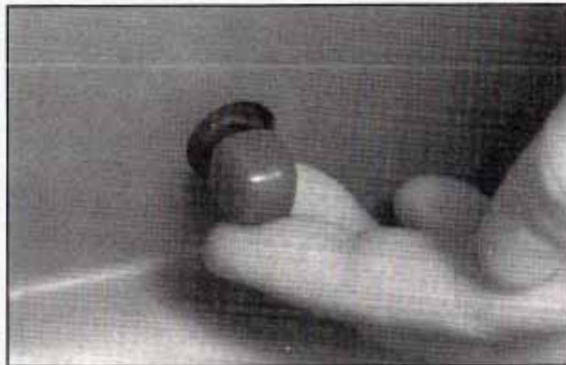
If your vehicle is equipped with this feature, there will be a control located on the outboard side of the driver's seat cushion, in front of the reclining seatback lever. To increase or decrease lumbar support, push the control forward or rearward. To adjust the lumbar support up or down, push the control up or down.
