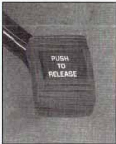
The parking brake is located to the left of the brake pedal near the driver's door. To set the parking brake, hold the regular brake pedal down with the right foot. Push down on the parking brake pedal, with the left foot.
