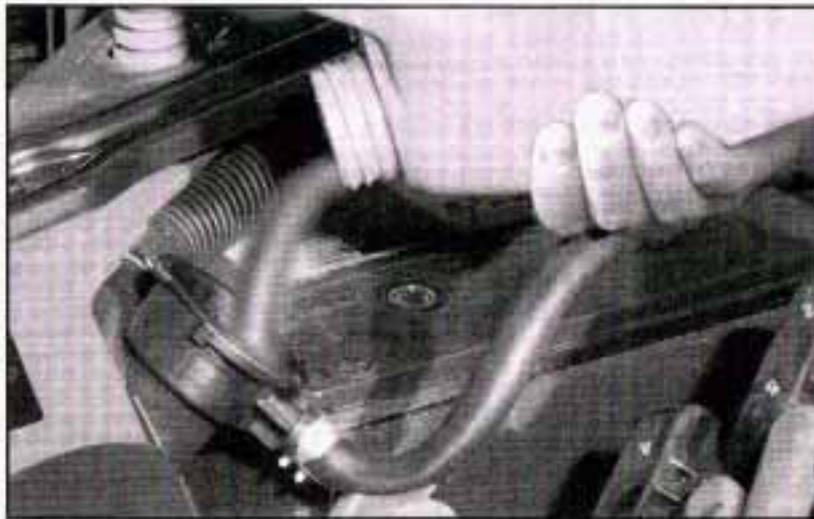
5. Fill the radiator with the proper DEX-COOL<sup>®</sup> coolant mixture, up to the base of the filler neck. See *Engine Coolant on page 5-30* for more information about the proper coolant mixture.
