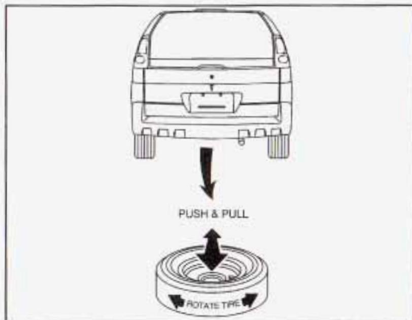
8. Make sure the tire is stored securely. Push, pull, and then try to rotate or turn the tire. If the tire moves, use the folding wrench to tighten the cable.
