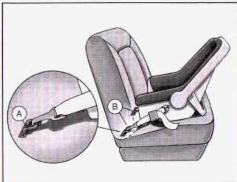
With this system, use the LATCH system instead of the vehicle's safety belts to secure a child restraint.
