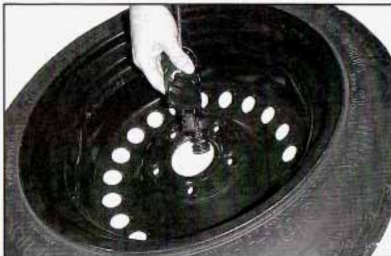
4. To remove the spare tire from the cable, tilt the retainer and slip it through the wheel opening.
