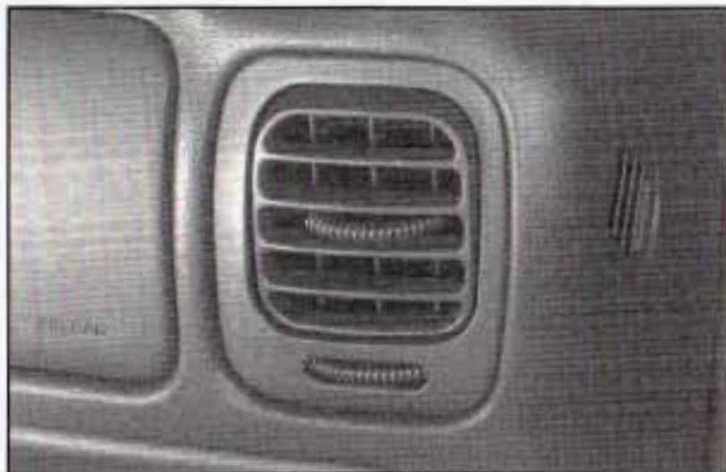
Use the thumbwheels located in the center and on the sides, to change the direction of the air flowing through the outlets.
