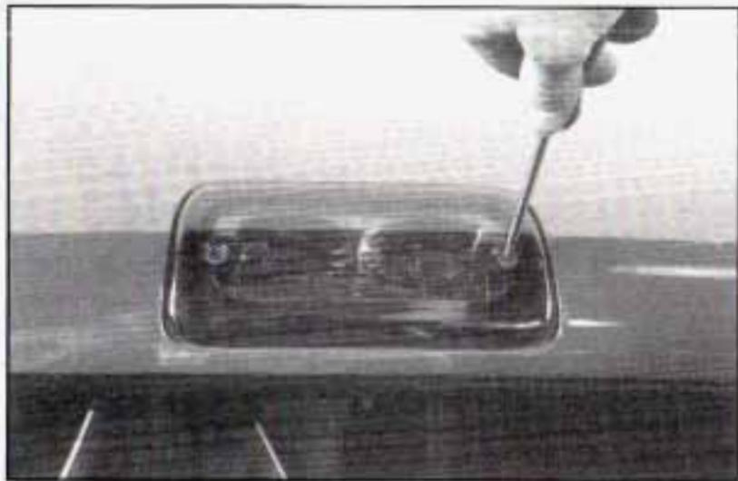
1. Remove the lens retaining screws.
