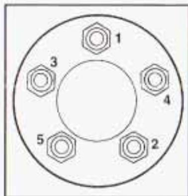
11. Use the wrench to tighten the wheel nuts firmly in a crisscross sequence as shown.
