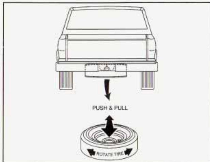
5. Make sure the tire is stored securely. Push, pull, and then try to rotate or turn the tire. If the tire moves, use the wheel wrench to tighten the cable. Return the jack, wheel wrench and wheel blocks to the proper location behind the seat. Secure the items.
