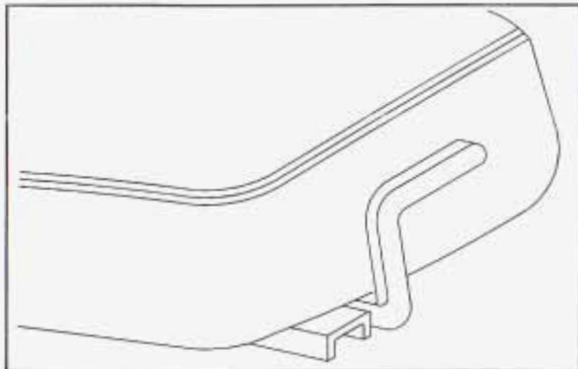
Move the lever under the front of a manual seat up to unlock it. Slide the seat to where you want it and release the lever. Try to move the seat with your body to make sure the seat is locked into place.
