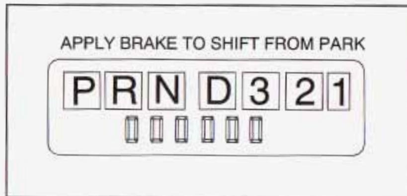
Your automatic transmission has a shift lever on the steering column.
