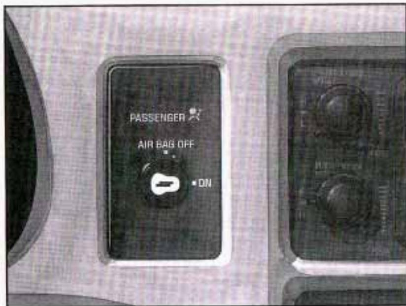
Unless your vehicle has the air bag off switch and the passenger's air bag has been turned off, never put a rear facing child restraint in the right front passenger's seat. Here's why:
