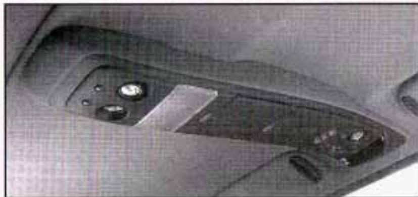
If your vehicle has this feature, the overhead console includes reading lamps, a compartment for a garage door opener, a temperature and compass display and a storage compartment for sunglasses.
