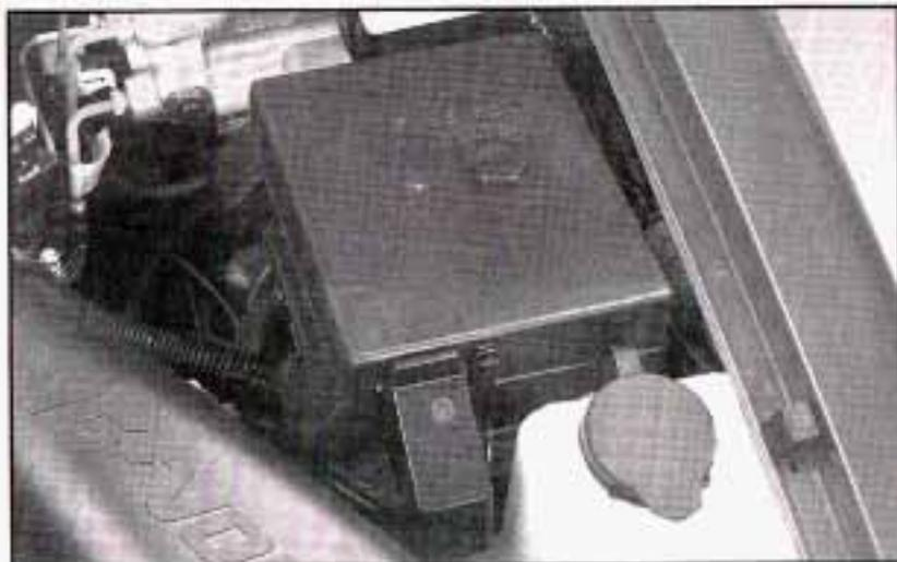
The engine compartment fuse block is located under the hood on the driver's side of the vehicle. See *Engine Compartment Overview* on page 5-12 for more information on location.
