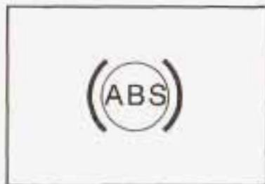
If there's a problem with the anti-lock brake system, this warning light will stay on. See *Anti-Lock Brake System Warning Light* on page 3-33.
