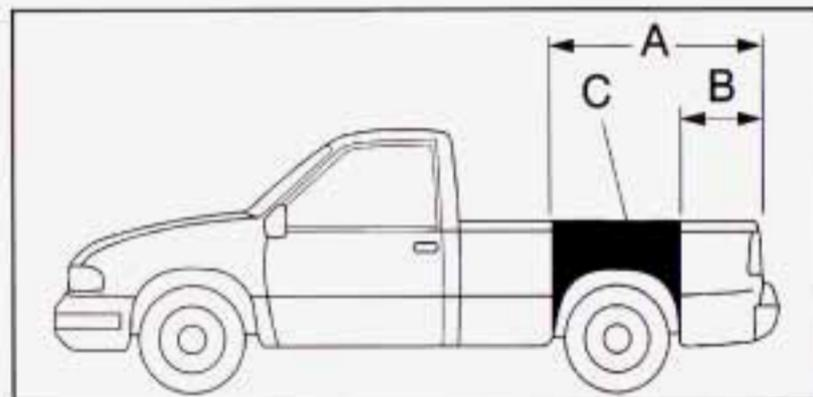
Use the rear edge of the load floor for measurement purposes. The recommended location for the cargo center of gravity for the Cargo Weight Rating (C) is the point where the mass of a body is concentrated and, if suspended at that point, would balance the front and rear.
