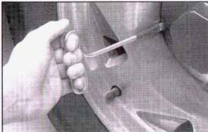
Position the bent end of your hub cap removal tool (shown), or the chisel end of your wheel wrench, in the notch of the hub cap and pry off the hub cap.
