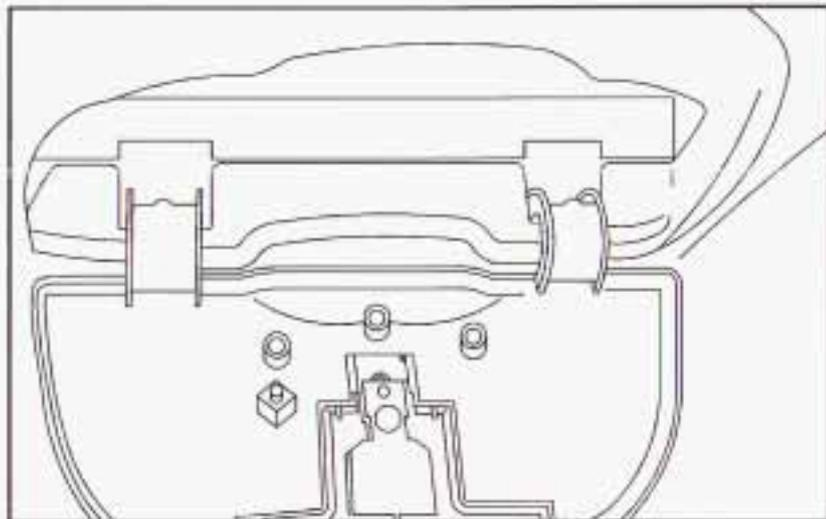
5. The pegs inside the compartment door are used to make sure the button on the compartment door will contact the control button on the garage door opener.
