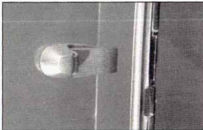
If your vehicle has this feature, squeeze the latch in the center of the window and slide the glass to open it.
