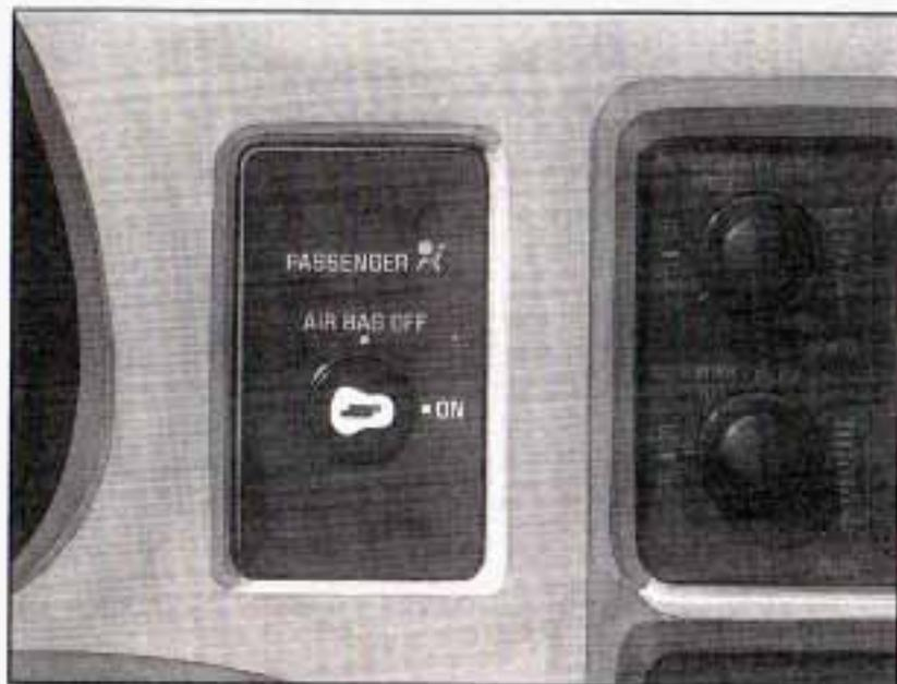
If your vehicle is a regular cab model or an extended cab model, it has a switch on the instrument panel that you can use to turn off the right front passenger's air bag.
