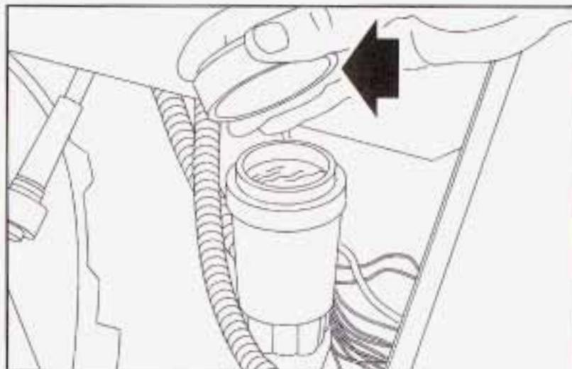
Refer to the Maintenance Schedule to determine how often you should check the fluid level in your clutch master cylinder reservoir and for the proper fluid. See *Part B: Owner Checks and Services* on page 6-25 and *Part D: Recommended Fluids and Lubricants* on page 6-32.
