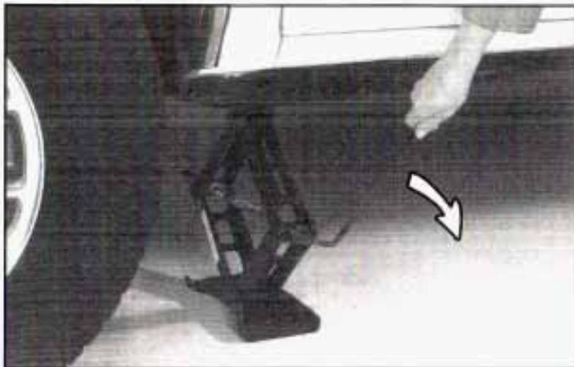
4. Raise the vehicle by turning the jack handle clockwise. Raise the vehicle far enough off the ground so there is enough room for the spare tire to fit underneath the wheel well.
