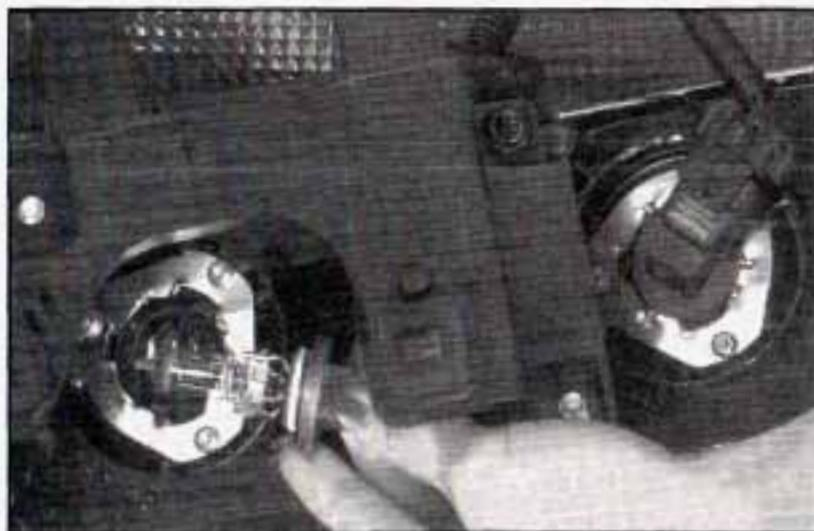
5. Turn the bulb assembly counterclockwise to remove it from the headlamp assembly.
