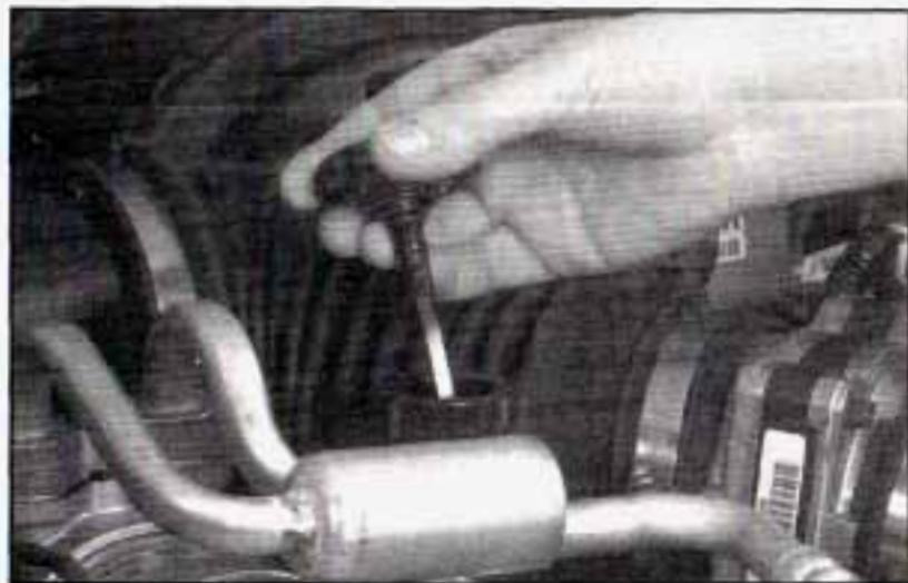
The power steering reservoir is located near the front of the engine compartment on the driver's side of the vehicle.
