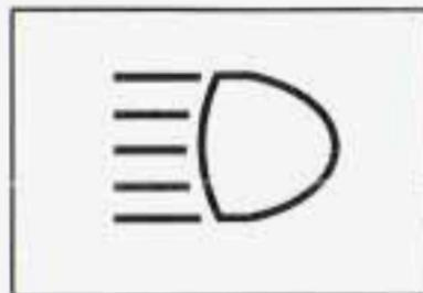
When the high-beam headlamps are on, this indicator light on the instrument panel cluster will also be on.
