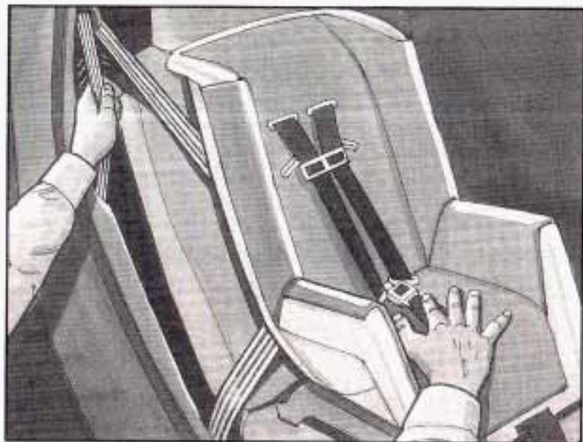
6. To tighten the belt, feed the shoulder belt back into the retractor while you push down on the child restraint. If you are using a forward-facing child restraint, you may find it helpful to use your knee to push down on the child restraint as you tighten the belt.
