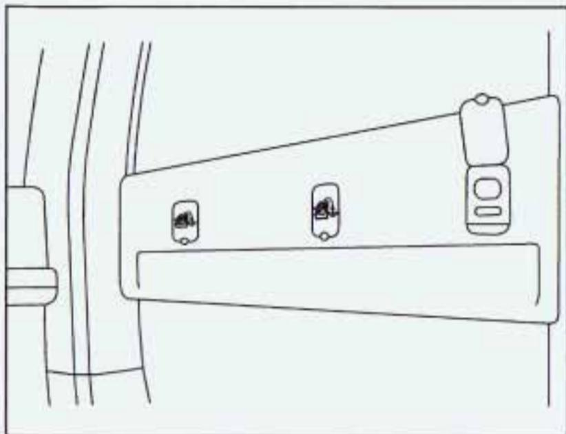
The anchor points for the rear seat child restraint positions in the Crew Cab<sup>®</sup> are located on the back wall behind the rear seat.
