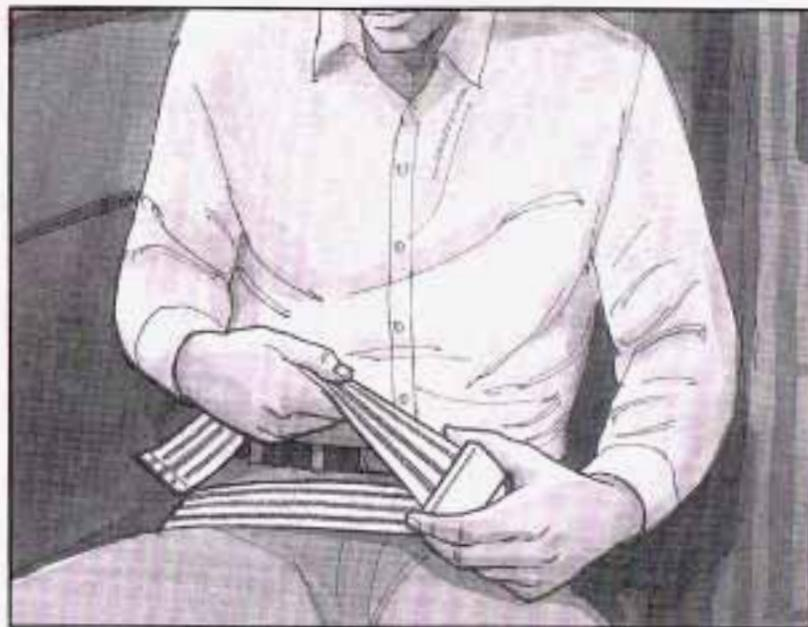
The jump seat has a lap belt with no retractor. To make the belt longer, tilt the latch plate and pull it along the belt.
