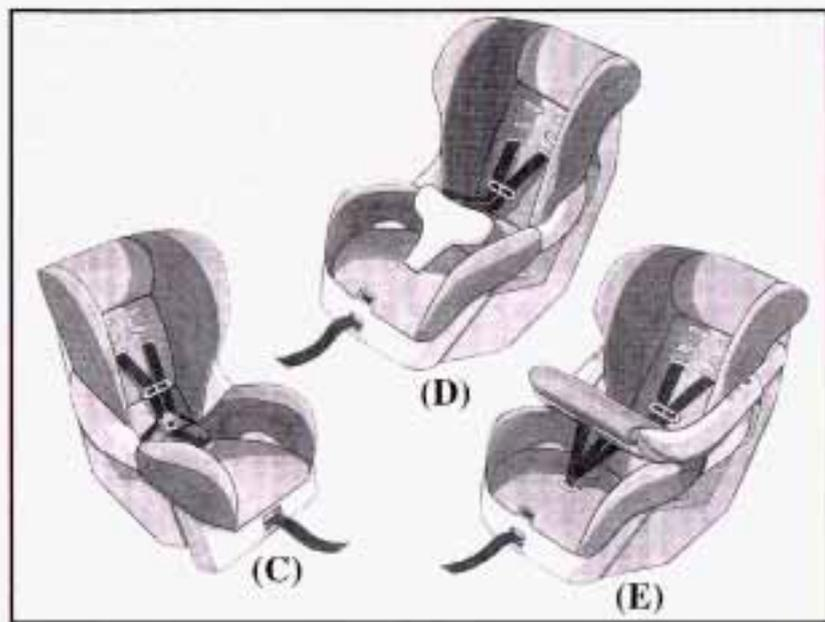
A forward-facing child seat (C-E) provides restraint for the child's body with the harness and also sometimes with surfaces such as T-shaped or shelf-like shields.
