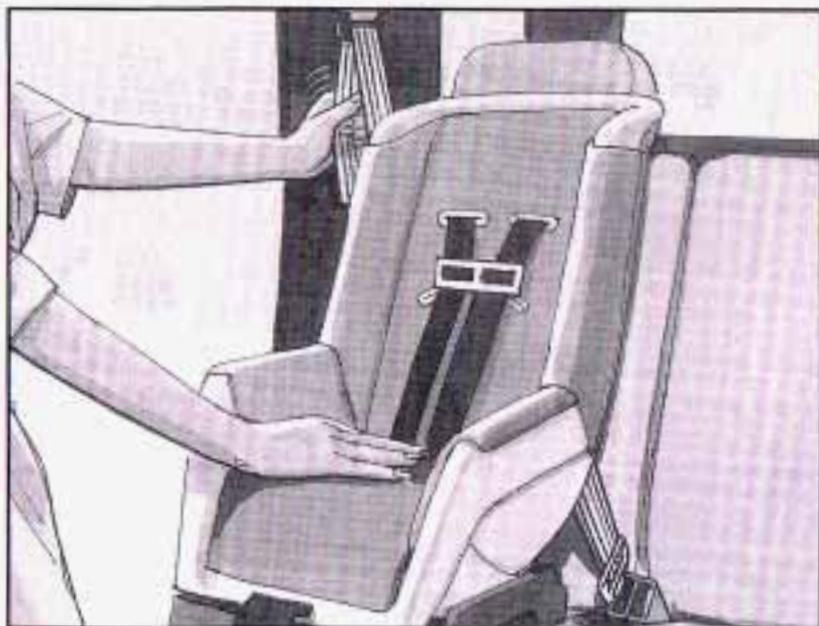
To remove the child restraint, just unbuckle the vehicle's safety belt and let it go back all the way. The safety belt will move freely again and be ready to work for an adult or larger child passenger.
