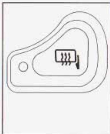
The heated mirror button is located to the lower right of the mode knob on the climate control system. The button has an indicator light to indicate if the heated mirror feature is on or off.
