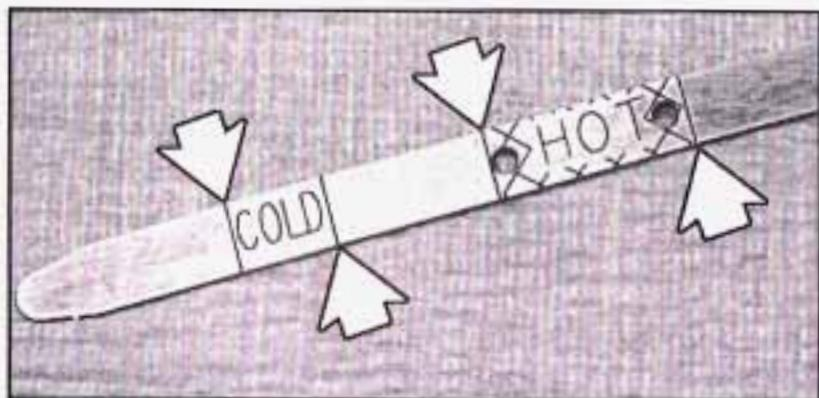
3. Check both sides of the dipstick, and read the lower level. The fluid level must be in the COLD area, below the cross-hatched area, for a cold check or in the HOT area or cross-hatched area for a hot check.
