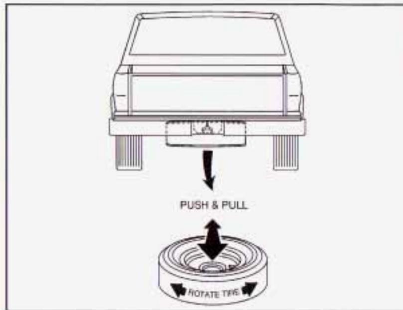
5. Make sure the tire is stored securely. Push, pull, and then try to rotate or turn the tire. If the tire moves, use the wheel wrench to tighten the cable.
