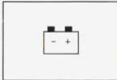
The charging system light will come on briefly when you turn on the ignition, but the engine is not running, as a check to show you it is working.
