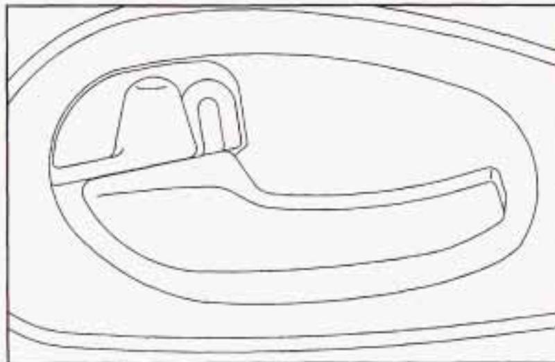
You can lock or unlock the door from the inside by sliding the manual lever forward or rearward. When the door is unlocked, you can see a red area on the lever.
