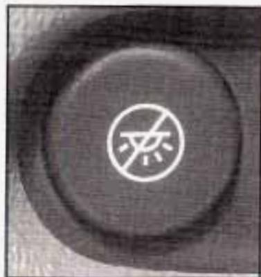
The dome override button is located below the exterior lamps knob.
