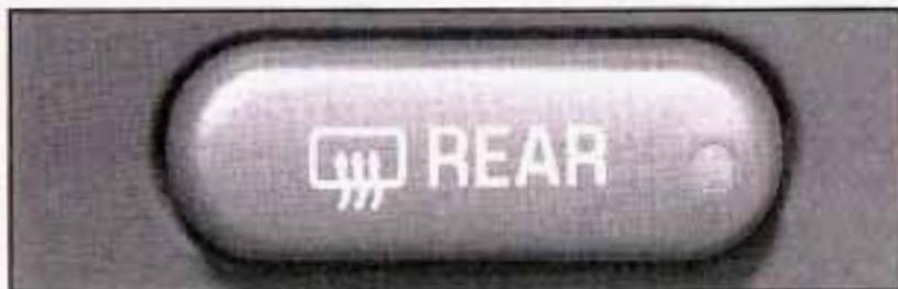
Press this button to turn the rear window defogger on or off. An indicator light in the button will come on to let you know that the rear window defogger is active. The rear window defogger will automatically turn off approximately ten minutes after the button is pressed.
