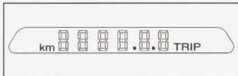
The trip odometer can tell you how far your vehicle has been driven since you last set the trip odometer to zero.
