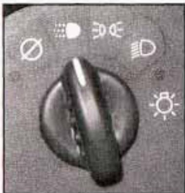
Your exterior lamps knob is located on your instrument panel to the left of the steering wheel.
