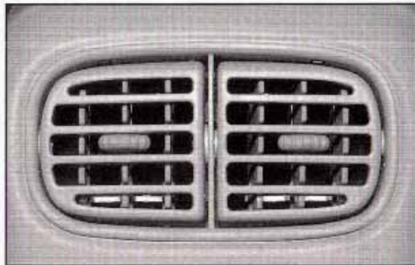
Your vehicle may have rear seat outlets that can be used to adjust the airflow toward either seating area, the floor or upward. Move the control in the center of each outlet in any direction to direct airflow.
