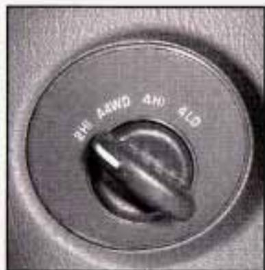
If your vehicle is equipped with the automatic transfer case, the transfer case knob is located to the right of the steering wheel on the instrument panel. Use this knob to shift into and out of four-wheel drive.
