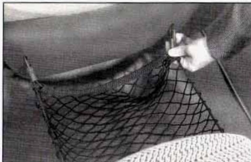
There may be a storage net that stretches between the front seats. Pull the hooks towards the passenger's seat and insert them into the holes.
