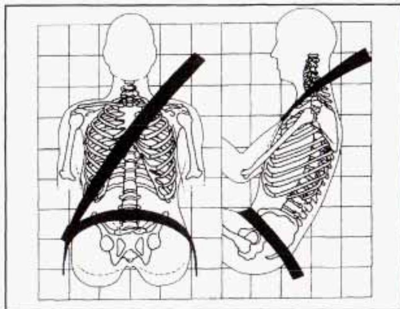
The lap part of the belt should be worn low and snug on the hips, just touching the thighs. In a crash, this applies force to the strong pelvic bones. And you'd be less likely to slide under the lap belt. If you slide under it, the belt would apply force at your abdomen. This could cause serious or even fatal injuries. The shoulder belt should go over the shoulder and across the chest. These parts of the body are best able to take belt restraining forces.
