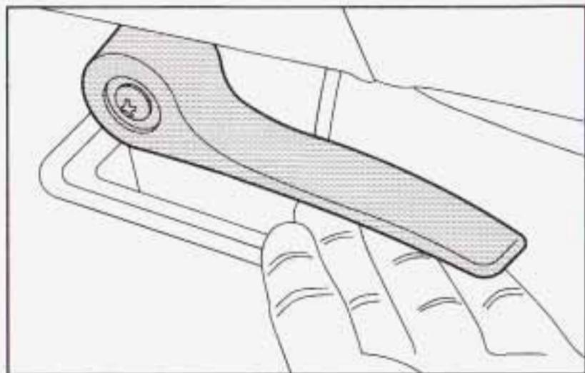
You can also lift the lever on the side of the seat to release the rear latches from the floor pins.
