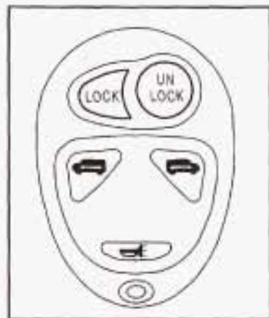
You can lock and unlock your doors and the liftgate from about 3 feet (1 m) up to 30 feet (9 m) away using the remote keyless entry transmitter supplied with your vehicle.
