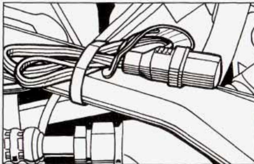
Your vehicle may have an engine coolant heater. In very cold weather, 0°F (-18°C) or colder, the engine coolant heater can help. You'll get easier starting and better fuel economy during engine warm-up. Usually, the coolant heater should be plugged in a minimum of four hours prior to starting your vehicle. At temperatures above 32°F (0°C), use of the coolant heater is not required.
