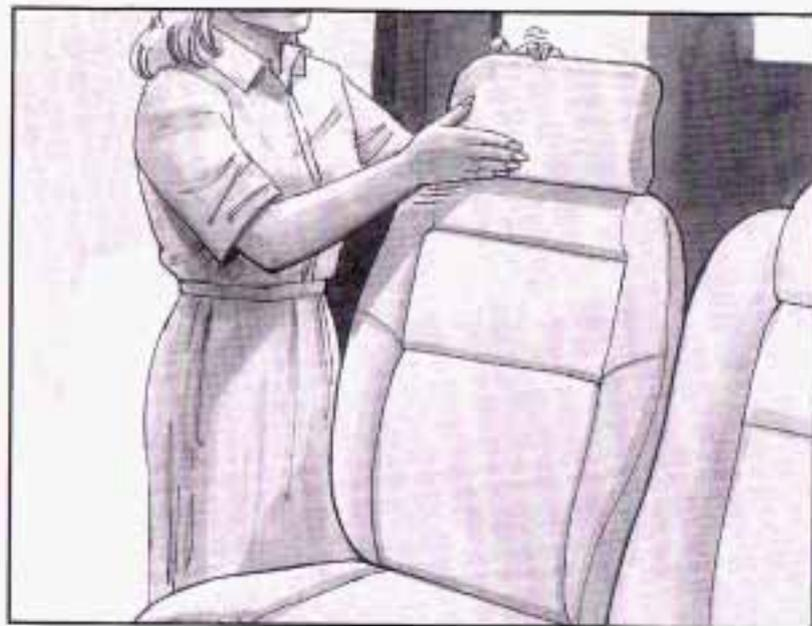
2. Rotate the head restraint rearward until it touches the top of the seatback. Make sure there is no gap between the lower edge of the head restraint and the top of the seatback.
