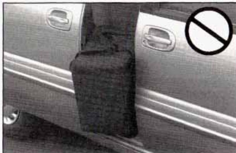
If an object obstructs the power sliding door(s) while it is closing, the door will automatically reverse to the open position, provided it meets sufficient resistance. Resistance must be as strong as the force of the closing door, or stronger. The force of the closing door increases significantly as the door approaches the latched position.
