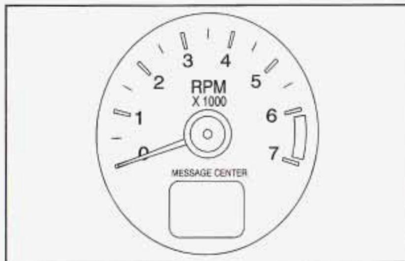
Your vehicle may have a tachometer that displays the engine speed in revolutions per minute (rpm).
