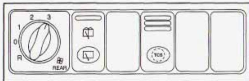
This switchbank is located in the instrument panel below the comfort controls. The switchbank may include the rear fan knob, the rear window wiper/washer and the traction control switches. If your vehicle does not have some of these options, there will be a blank.
