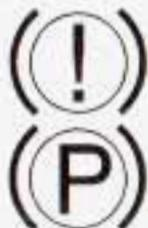
When your brake fluid falls to a low level, your brake warning light will come on. See *Brake System Warning Light* on page 3-41.
