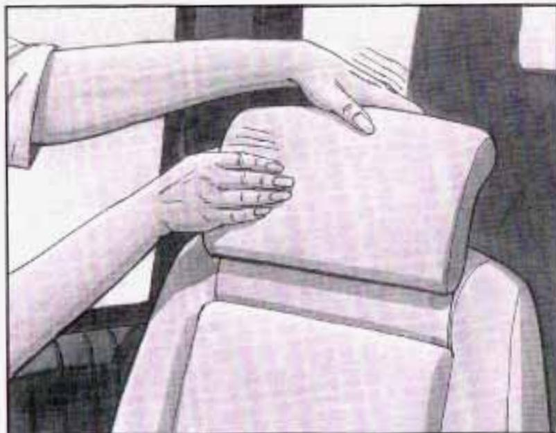
5. Rotate the head restraint forward and push it all the way down.
