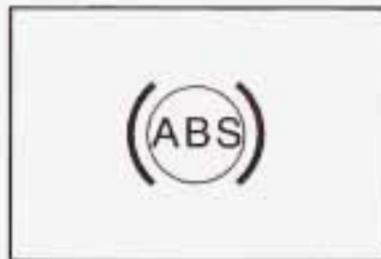
Your vehicle may have this light. If it does, the anti-lock brake system warning light should come on for a few seconds when you turn the ignition key to RUN.
