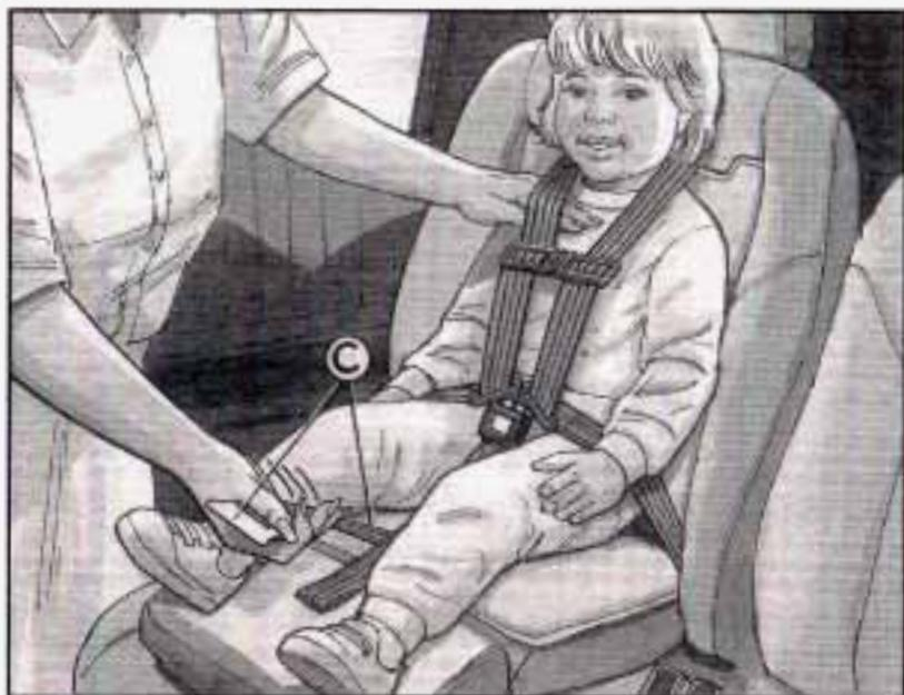
12. Pull the shoulder harness adjustment strap (C) firmly until the harness is snugly adjusted around the child. You should not be able to put more than two fingers between the harness and the child's chest. Make sure the harness and buckle strap are not twisted.
