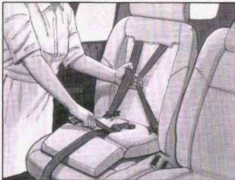
4. Before placing the child in the child restraint, add slack to the shoulder harness. Pull the black shoulder harness release strap firmly. At the same time pull both shoulder harness straps through the slots in the seatback as shown.
