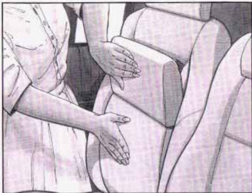
4. Then press the leg rest firmly into the seatback, and secure it by pressing the upper corners against the fastener strips on the seatback.
