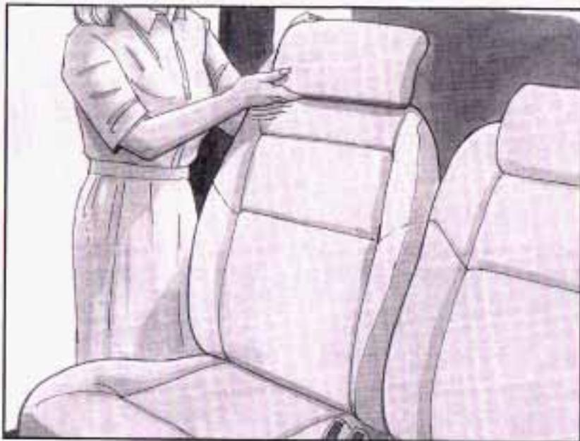
1. Raise the head restraint until the lower edge of the head restraint is even with the top of the seatback.
