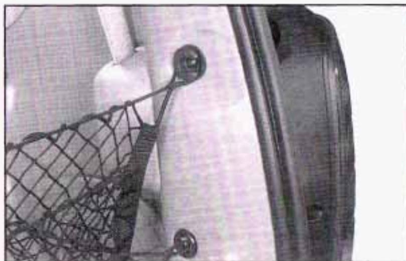
1. Attach the upper loops to the posts on either side of the liftgate opening. The label on the net should be in the upper left-hand corner.
