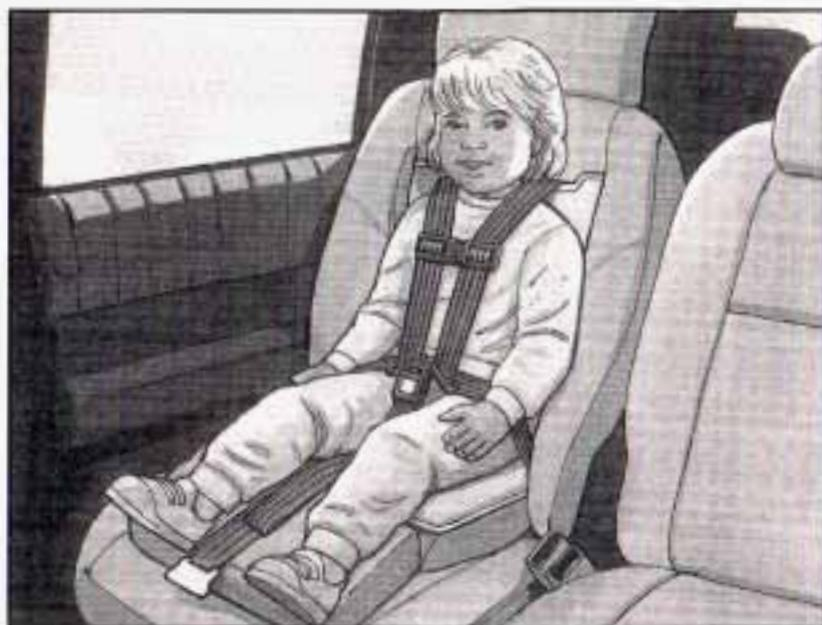
13. Adjust the position of the harness on the child's shoulder by moving the clip along the harness until it is level with the child's armpits. On each side of the harness, the shoulder part should be centered on the child's shoulder. The harness should be away from the child's face and neck, but not falling from the child's shoulders.
