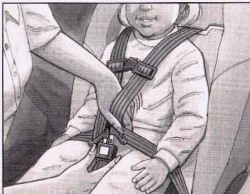
10. Pull up on the latch plates to make sure they are secure.
