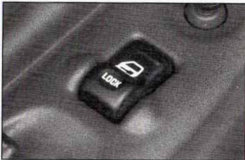
From the inside, press the front of the power door lock switch (on either front door) to unlock all doors and the liftgate. With the content theft-deterrent system, the power door lock switch will not unlock the doors until the system is disarmed. See *Content Theft-Deterrent on page 2-27* for more details.
