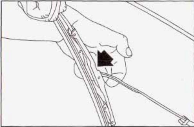
5. Push the release clip at the connecting point of the blade and the arm up. Then pull the blade assembly down toward the glass to remove it from the wiper arm.
