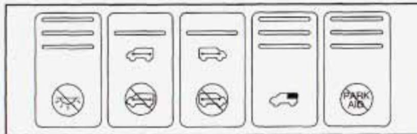
This switchbank is located in the overhead console. The switchbank may include the interior lamps override, the power sliding door(s)/override, the power rear quarter windows and the Ultrasonic Rear Parking Aid (URPA) disable switches. If your vehicle does not have some of these options, there will be a blank.
