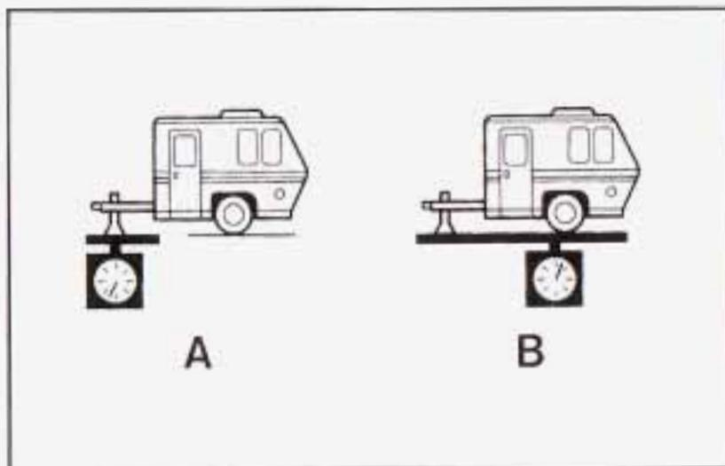
If you're using a weight-carrying or a weight-distributing hitch, the trailer tongue weight (A) should be 10 percent to 15 percent of the total loaded trailer weight (B). Do not exceed the maximum allowable tongue weight for your vehicle.
