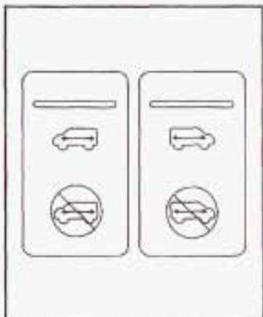
If you have the dual sliding doors, your vehicle has these switches. The left switch is for the driver's side power sliding door and the right switch is for the passenger's side sliding door. The power sliding door and the power sliding door override is one switch.
