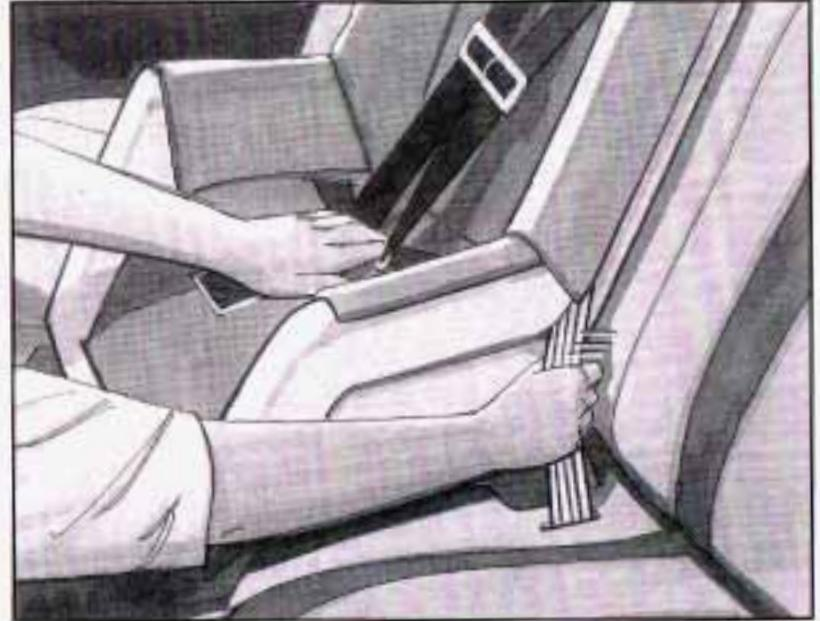
5. To tighten the belt, feed it back into the retractor while you push down on the child restraint. If you're using a forward-facing child restraint, you may find it helpful to use your knee to push down on the child restraint as you tighten the belt.
