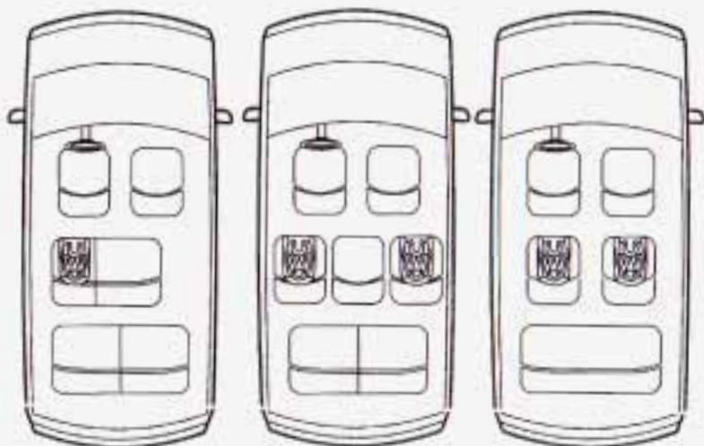
To assist you in locating the lower anchors for this child restraint system, each seating position with the LATCH system will have latches between the seatback and cushion.
