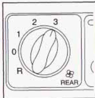
This knob is located below the main climate-control system on the instrument panel switchbank. Use this knob to adjust the fan speed for the rear-seat passengers, from the front-seating area.
