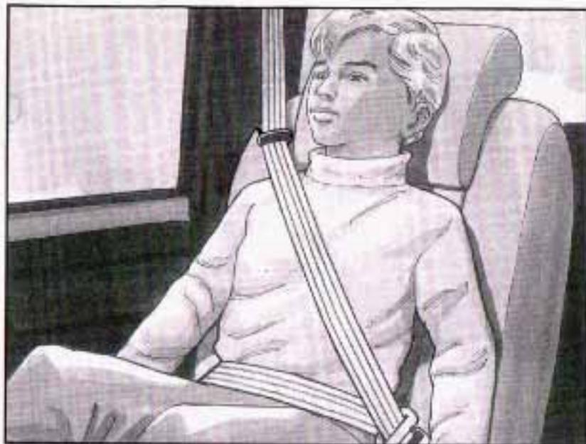
4. Buckle, position and release the safety belt as described in *Rear Seat Passengers* on page 1-48. Make sure that the shoulder belt crosses the shoulder.
