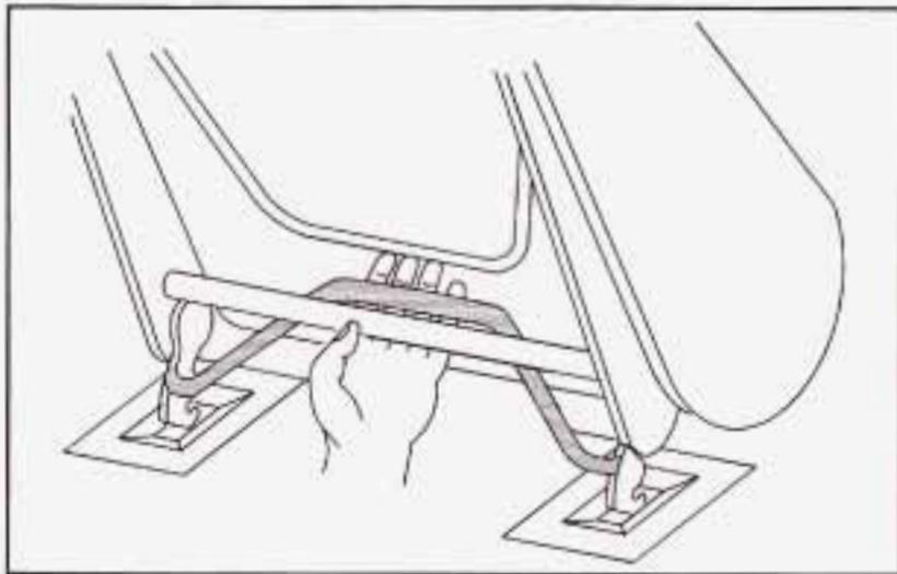
6. To unlatch the front latches, squeeze the angled bar toward the straight crossbar.
