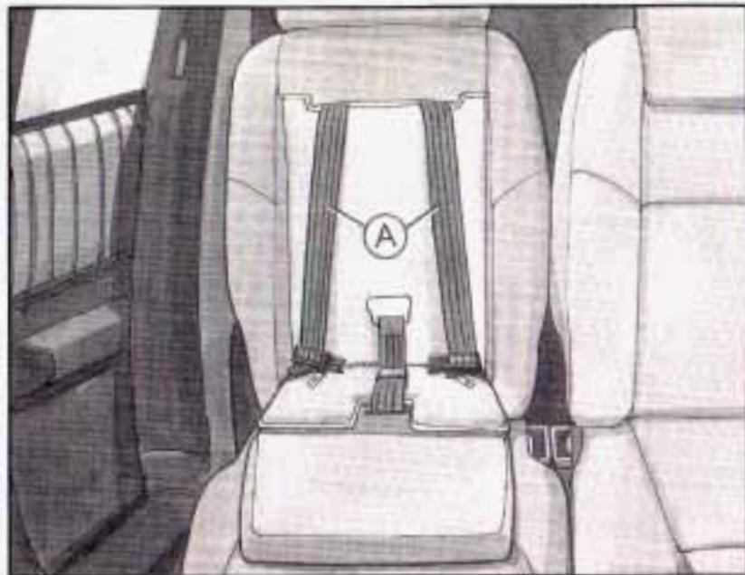
You'll be using the child restraint's harness (A) to secure your child. Don't use the vehicle's safety belts.
