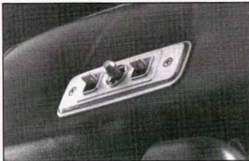
If your vehicle has a power seat on the driver's or passenger's side, you can adjust it with these controls located at the front center of the seat cushion.
