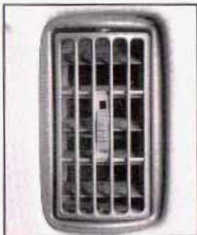
Use the outlets located near the center and on the sides of the instrument panel to change the direction of airflow.
