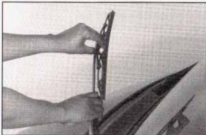
Replacement blades come in different types and are removed in different ways. To remove the type with a release clip, do the following:
