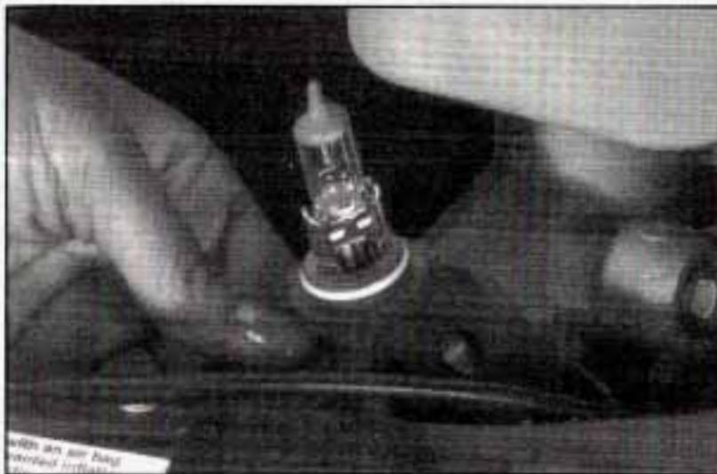
8. Without removing the headlamp assembly itself, remove the bulb socket from the back of the headlamp on the driver's side.
