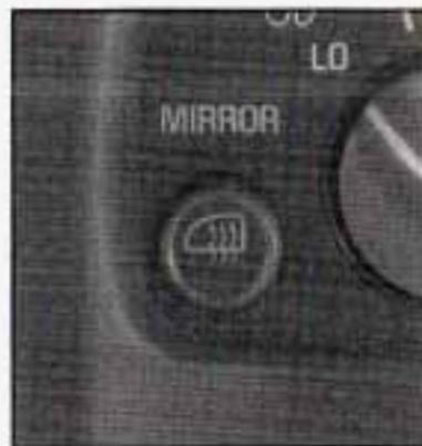
Your outside mirrors can be defrosted by pressing the button located near the fan control.
