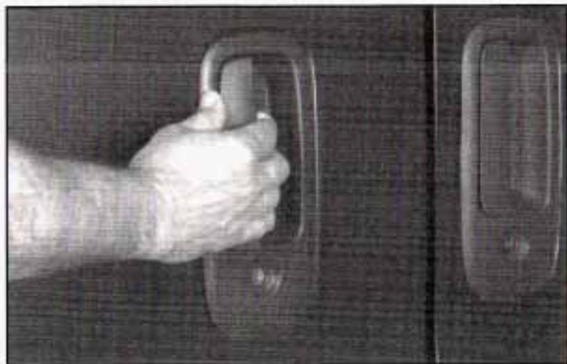
To open the sliding side door from outside, pull the handle toward the rear of the vehicle. Then, slide the door open.
