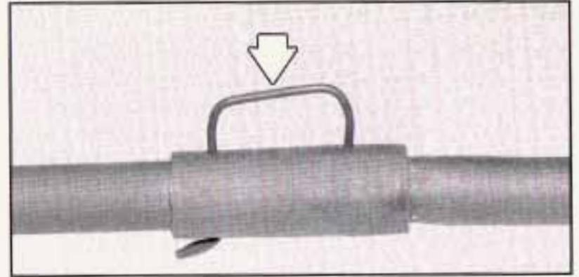
4. Connect the jack handle (C) and jack handle extension (B) together and press the retention clip (arrow) so it engages.
