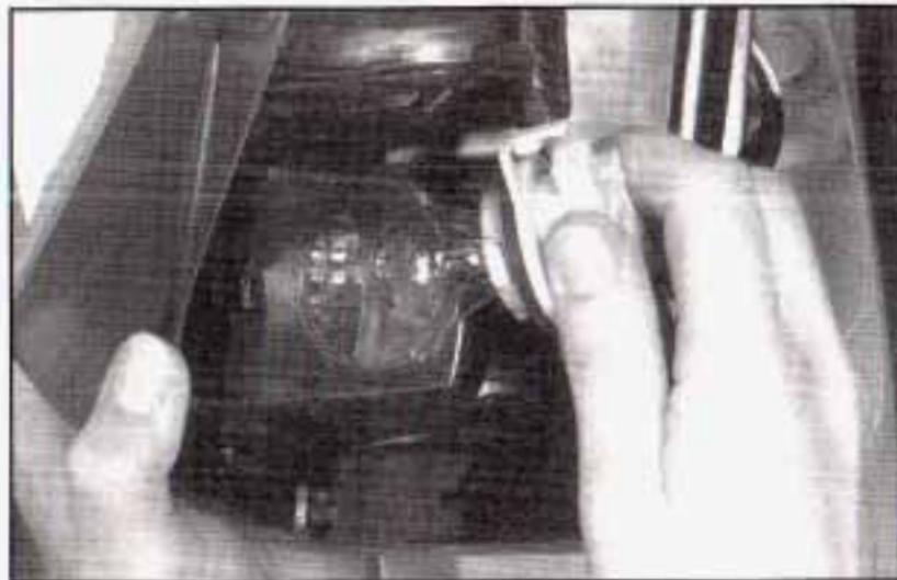
9. Turn the bulb counterclockwise to remove it. Install the new bulb.
