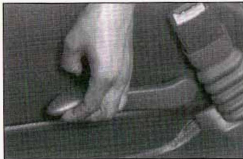
To adjust the seatback, lift the front of the lever, which is located on the inboard side of the seat cushion.
