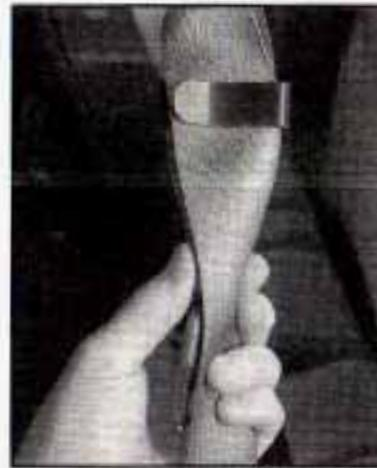
7. For the first rear seat, stow the safety belt latch by attaching the clip on the safety belt latch to the trim just inside the side door. For the remaining rear seats, stow the safety belt latch plate on the clip at the window trim.
