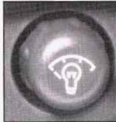
Press this knob located next to the exterior lamps knob to extend and turn it to make your instrument panel brighter. Turn the knob all the way up to turn on the interior lamps. Press the knob back into its stored position.
