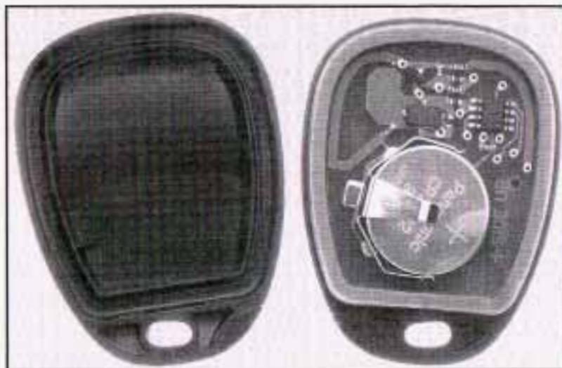
1. Use an object like a coin to pry open the transmitter.
