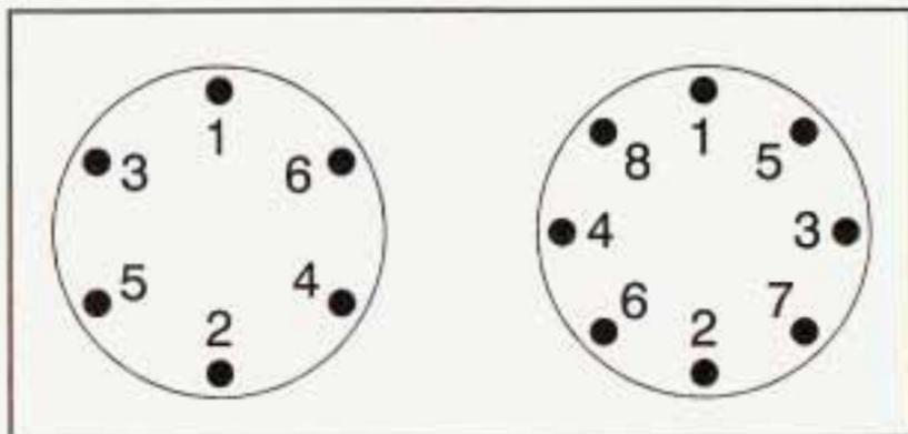
9. Tighten the nuts firmly in a crisscross sequence as shown. Turn the wheel wrench clockwise.
