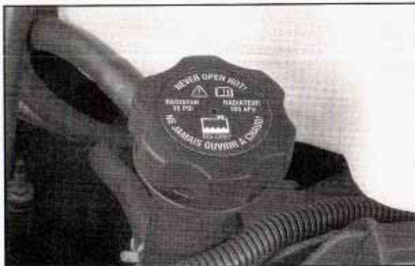
The radiator pressure cap is located near the center of the engine compartment.
