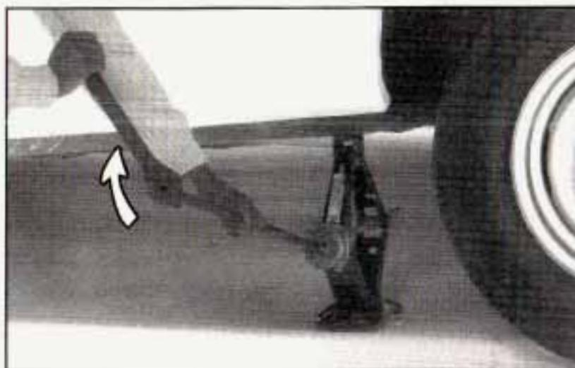
4. Raise the vehicle by turning the ratchet clockwise. Make sure the UP mark faces you. Raise the vehicle far enough off the ground so there is enough room for the spare tire to fit.
