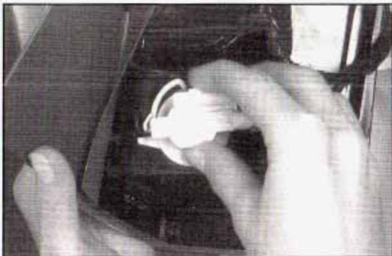
8. To remove, squeeze the tab on the side of the sockets while turning them counterclockwise.
