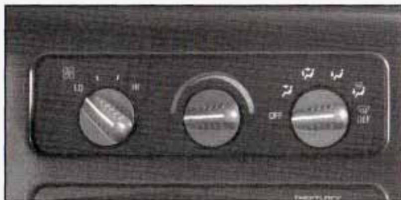
Turn the right knob clockwise or counterclockwise to direct the airflow inside of your vehicle.
