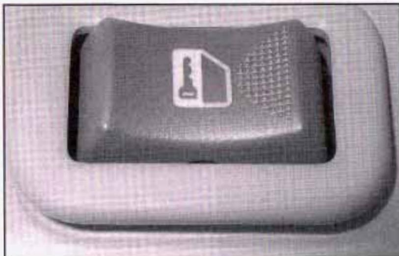
Press the bottom side of the power door lock switch to lock all the doors at once. Press the top side of the power door lock switch to unlock all the doors at once.
