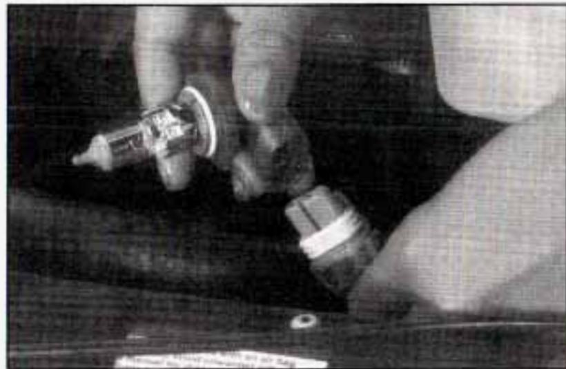
11. Install the new bulb into the socket and return it to the headlamp assembly.
