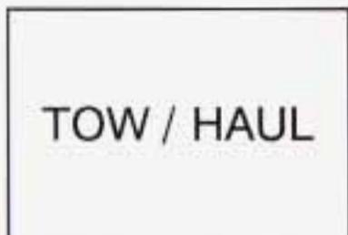
When the button is pressed, this light on the instrument panel will illuminate to indicate that tow/haul has been selected.
