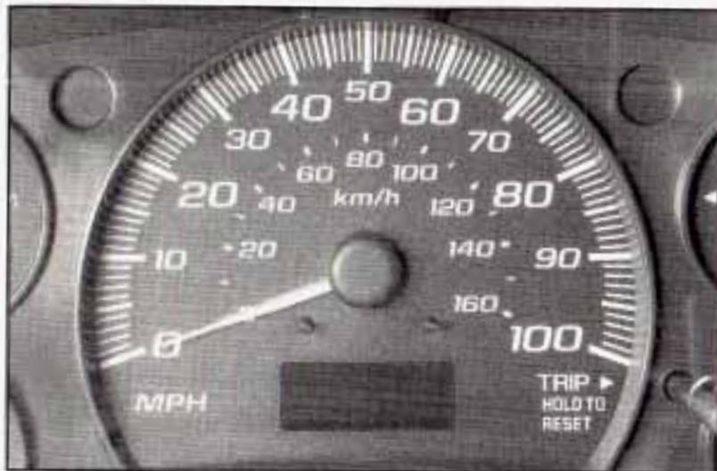
Your speedometer lets you see your speed in both miles per hour (mph) and kilometers per hour (km/h). Your odometer shows how far your vehicle has been driven, in either miles (used in the United States) or kilometers (used in Canada).
