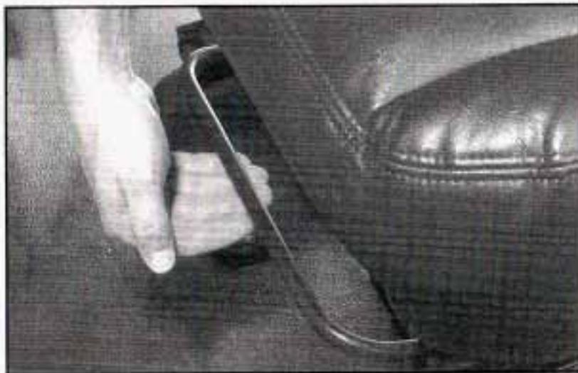
The bucket seats can be adjusted forward or rearward with the lever located at the front of the seat.
