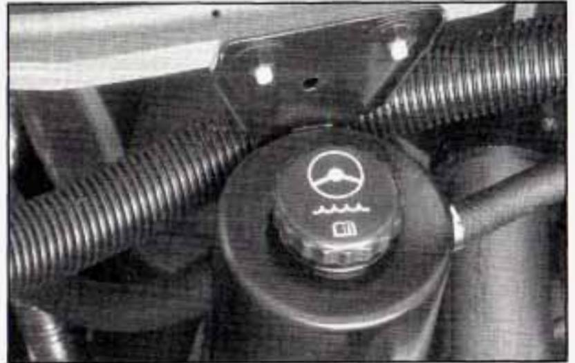
The power steering fluid reservoir is located in the engine compartment on the driver's side of the vehicle.
