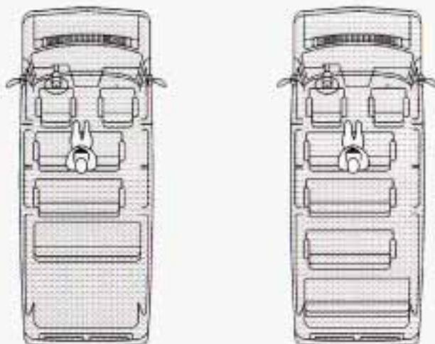
If your vehicle has a second row bench seat, someone can sit in the center position. When you sit in the center position in the second row bench seat, you have a lap-shoulder belt which works the same way as the rear seat outside passengers' belts. To learn how to wear a lap-shoulder belt see, "Lap-Shoulder Belt" under *Rear Seat Passengers on page 1-27*.
