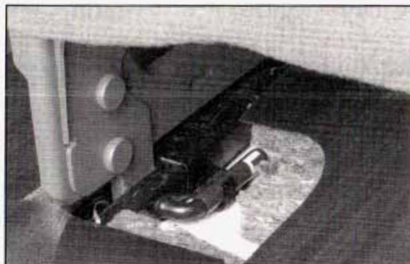
4. Push the pin with the white handle marked "R" down until it is in the retaining clip.
