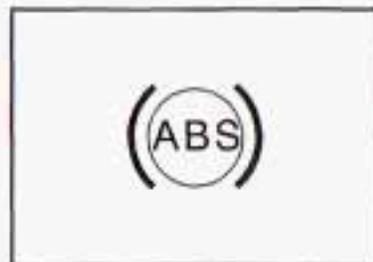
If there's a problem with the anti-lock brake system, this warning light will stay on. See *Anti-Lock Brake System Warning Light* on page 3-32.
