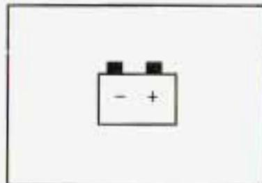
This light should come on briefly when you turn on the ignition, before starting the engine, as a check to show you it is working.
