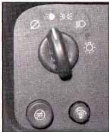
The control on the driver's side of your instrument panel operates the exterior lamps. Turn the control clockwise to operate the lamps.
