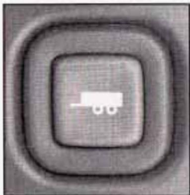
Your vehicle is equipped with a button on the instrument panel, to the right of the steering wheel, which when pressed enables tow/haul.
