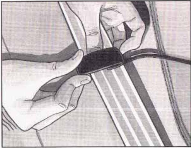
3. Be sure the belt is not twisted and it lies flat. The elastic cord must be under the belt and the guide on top.
