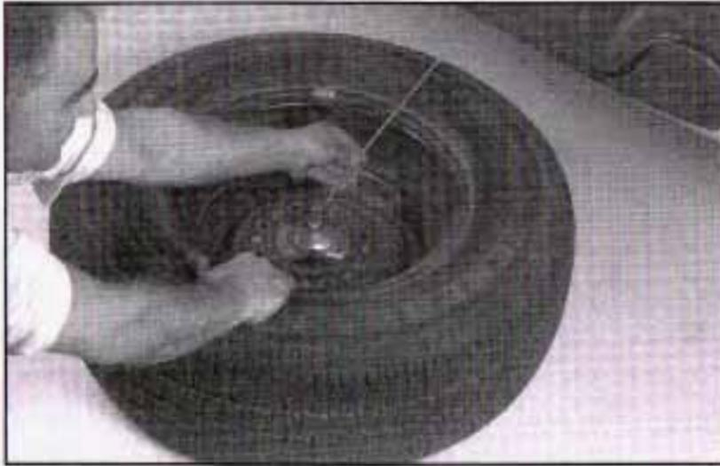
3. Pull the wheel toward the rear of the vehicle, keeping the cable tight.
