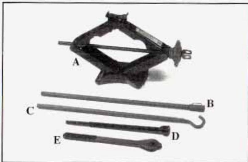
The tools you'll be using include the jack (A), jack handle extension (B), jack handle (C), wheel wrench (D) and the ratchet (E).
