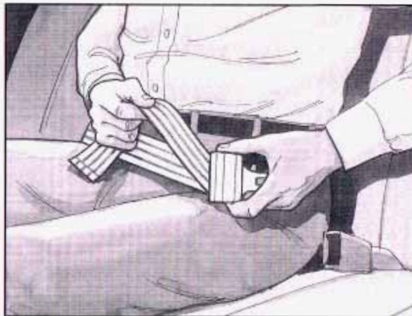
When you sit in a center seating position in the third, fourth or fifth row, you have a lap safety belt, which has no retractor. To make the belt longer, tilt the latch plate and pull it along the belt.
