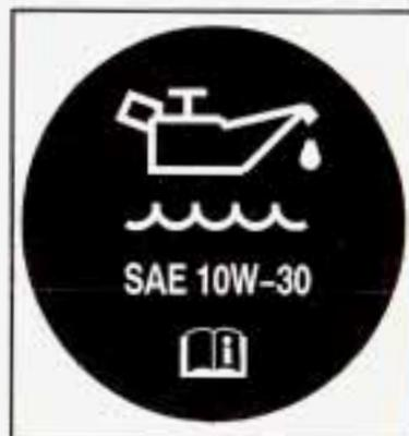
Add engine oil at the engine oil fill cap next to the oil dipstick. See *Engine Compartment Overview on page 5-12* for more information on location.
