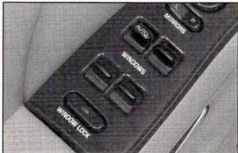
Use the switches on the driver's door armrest to control each of the windows while the ignition is on or while Retained Accessory Power (RAP) is active. See "Retained Accessory Power (RAP)" under *Ignition Positions* on page 2-25 for more information. In addition, each passenger door has a window switch.
