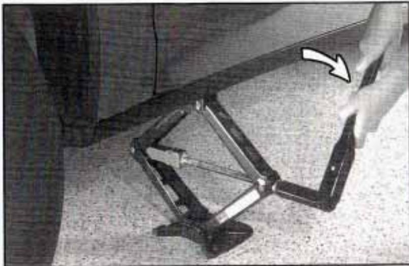
5. Raise the vehicle by turning the wheel wrench clockwise in the jack. Raise the vehicle far enough off the ground so there is enough room for the compact spare tire to fit underneath the wheel well.
