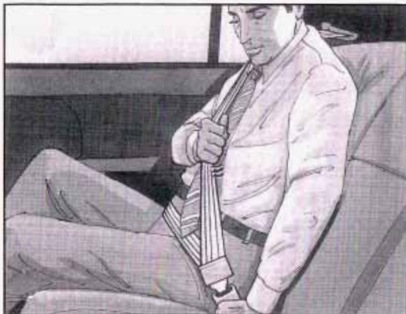
3. To make the lap part tight, pull down on the buckle end of the belt as you pull up on the shoulder belt.
