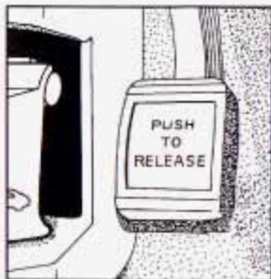
This vehicle has a PUSH TO RELEASE parking brake pedal. To set the parking brake, hold the regular brake pedal down with your right foot. Push down the parking brake pedal with your left foot.
