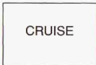
The CRUISE light comes on when you set the vehicle's cruise control. See "Cruise Control" under *Turn Signal/Multifunction Lever* on page 3-5.
