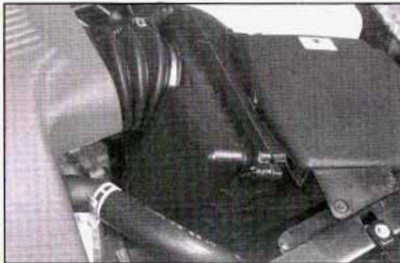
The engine air cleaner/filter is in the engine compartment on the driver's side of the vehicle. See *Engine Compartment Overview* on page 5-12 for more information on location.
