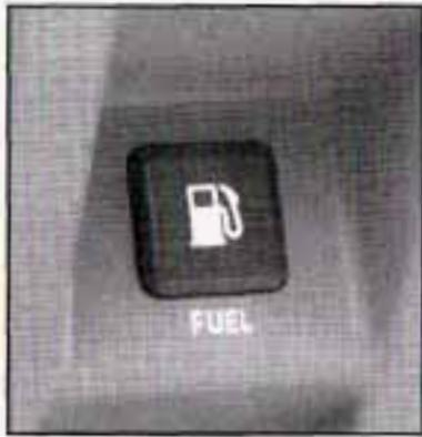
The release button for the fuel door is located to the left of the steering column.
