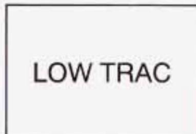
If your vehicle has the Enhanced Traction System, this light will come on when the system is limiting wheel spin.
