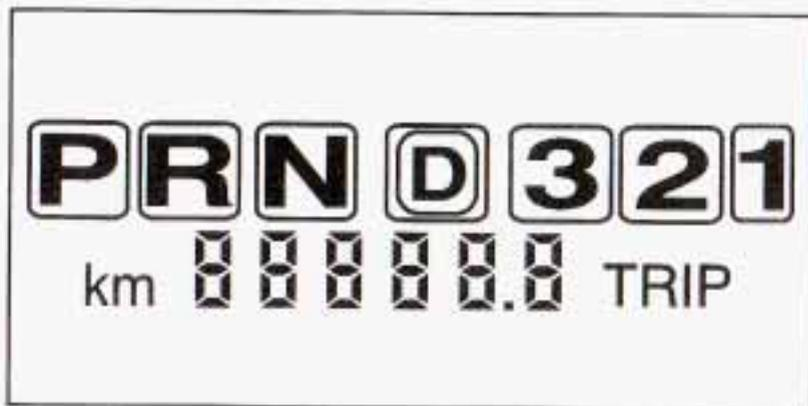
The graphic shown above is displayed on your instrument panel cluster and will indicate the gear your vehicle is in when you move.
