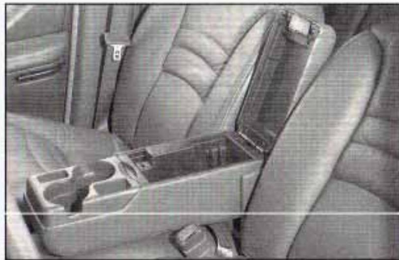
To use the storage area, fold down the armrest located in the center front seat. Press the latch on the front edge and pull up to access the storage area.
