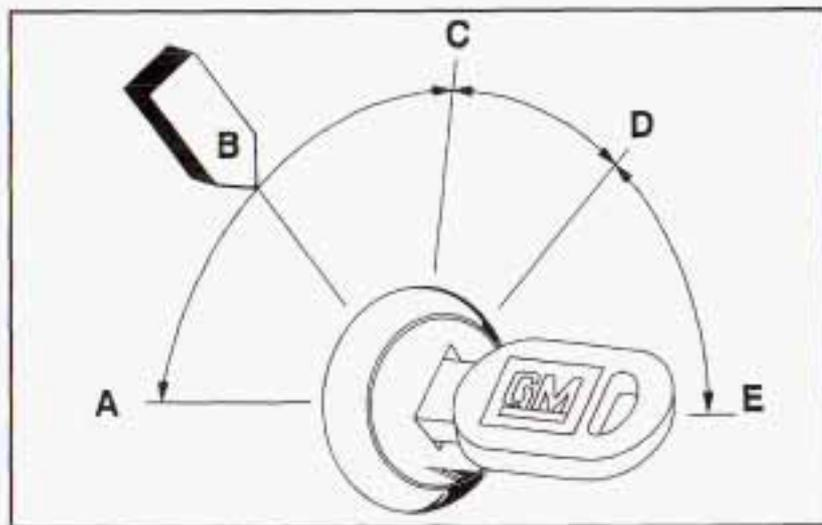
**A (ACCESSORY):** This position lets you use the radio and windshield wipers when the engine is off. To use ACCESSORY, push in the key and turn it toward you. Your steering wheel will stay locked.
