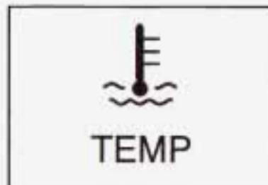
This light tells you that your engine coolant has overheated or your radiator cooling fan is not working.
