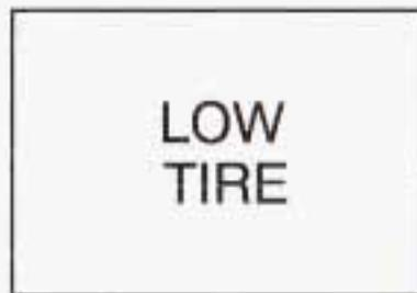
Your vehicle may have a tire pressure monitor that can alert you to a large change in the pressure in one tire.
