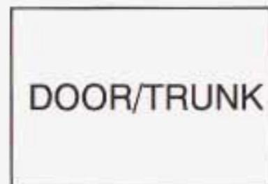
The DOOR/TRUNK light will come on if your trunk or any door is not completely closed.
