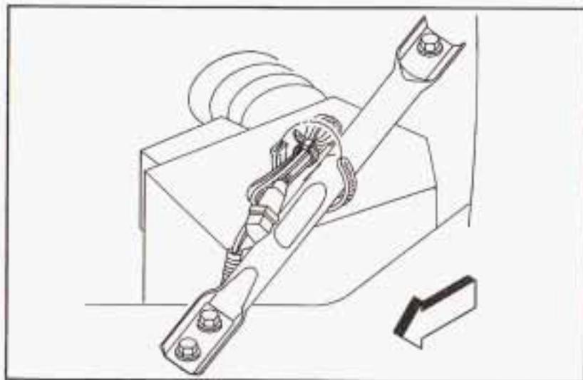
Your vehicle may be equipped with this feature. In very cold weather, 0°F (-18°C) or colder, the engine coolant heater can help. You'll get easier starting and better fuel economy during engine warm-up. Usually, the coolant heater should be plugged in a minimum of four hours prior to starting your vehicle. At temperatures above 32°F (0°C), use of the coolant heater is not required.
