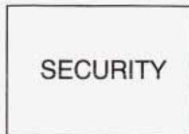
The SECURITY light will come on when you turn the key to START and stay on until the vehicle starts.
