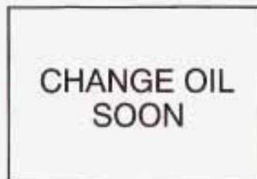
The CHANGE OIL SOON light should come on briefly as a bulb check when you start the engine. If the light doesn't come on, have it serviced.
