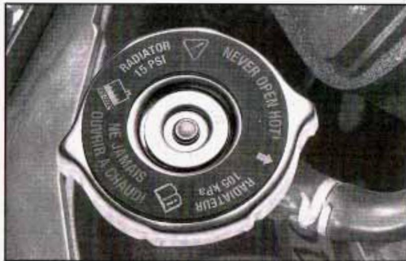
Turn the pressure cap slowly counterclockwise until it first stops. (Don't press down while turning the pressure cap.)
