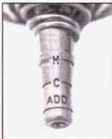
When the engine compartment is hot, the level should be at the H (hot) mark. When it's cold, the level should be at the C (cold) mark. If the fluid is at the ADD mark, you should add fluid.
