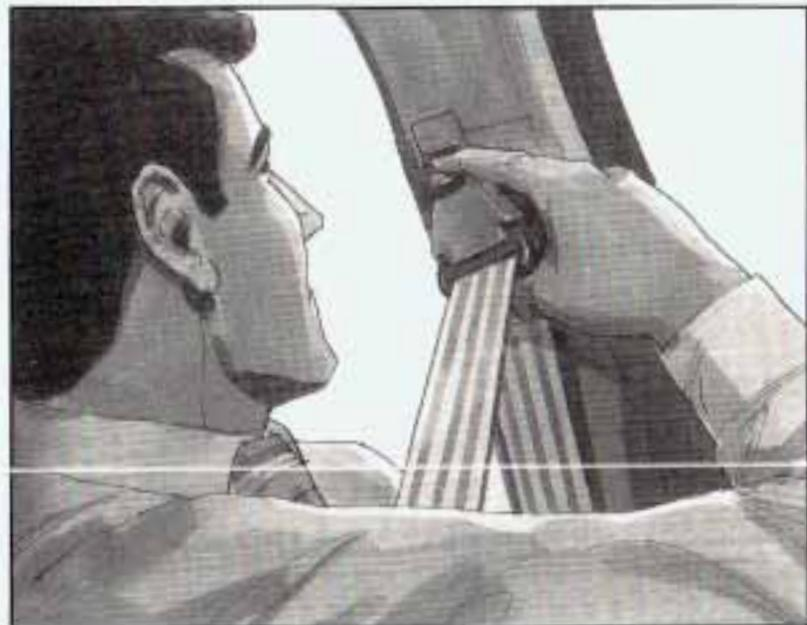
To move it down, squeeze the release lever and the shoulder belt guide as shown and move the height adjuster to the desired position. You can move the adjuster up just by pushing up on the shoulder belt guide. After you move the adjuster to where you want it, try to move it down without squeezing the release lever to make sure it has locked into position.
