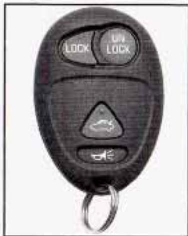
Using the remote keyless entry transmitter, you can lock and unlock your doors, or release the trunk from about 3 feet 1 (m) and up to 30 feet 9 (m) away.
