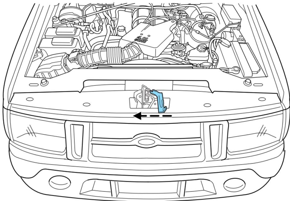
3. Lift the hood until the lift cylinders hold it open.
