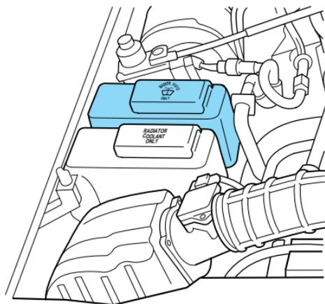
Only use a washer fluid that meets Ford specifications. Refer to *Lubricant specifications* in the *Capacities and specifications* chapter. State or local regulations on volatile organic compounds may restrict the use of methanol, a common windshield washer antifreeze additive. Washer fluids containing non-methanol antifreeze agents should be used only if they provide cold weather protection without damaging the vehicle's paint finish, wiper blades or washer system.
