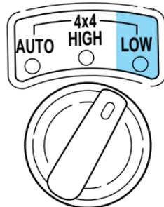
**The vehicle should not be operated in 4WD HIGH and 4WD LOW on dry or merely wet pavement. Doing so will produce excessive noise, increase tire wear and may damage driveline components. These modes are intended for use only on consistently slippery or loose surfaces.**
