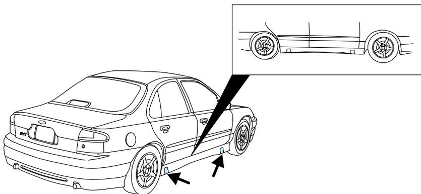
The SVT Contour has two jacking points on each side of the car to be utilized if it is necessary to change to your spare tire.
