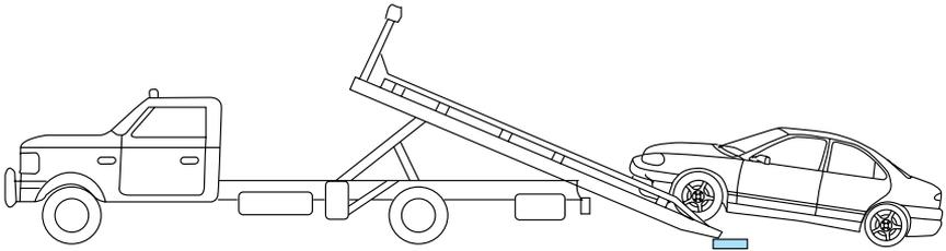
When towing your SVT Contour with flatbed equipment, you must place a block under the tongue of the inclined flatbed to decrease the angle of ascent and descent.
