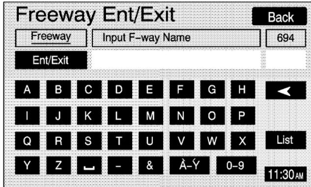
Enter Freeway names using the alpha keypad. See “Alpha-Numeric Keypad” listed previously in this section for more information. After entering the freeway name, enter the name of the entrance or exit that you wish to set as the destination using the alpha keypad.
