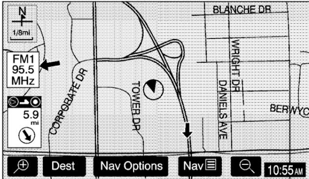
The main navigation menu allows you to choose from a list of options and to use the available touch screen buttons to make system adjustments and plan routes.
