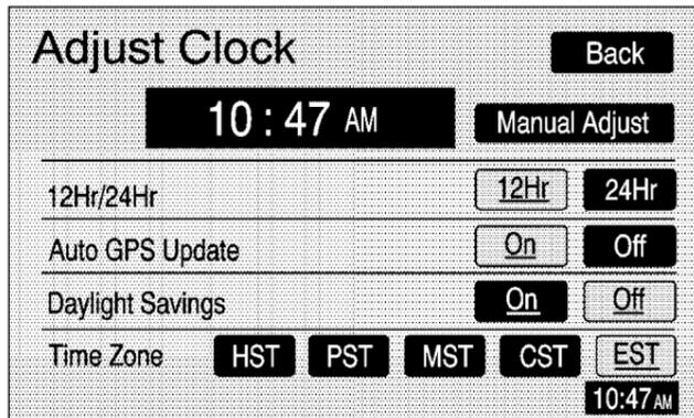
To adjust the time displayed at the lower right corner of the navigation screen, as well as other time options, touch the Clock screen button. This will take you to the Adjust Clock screen.
