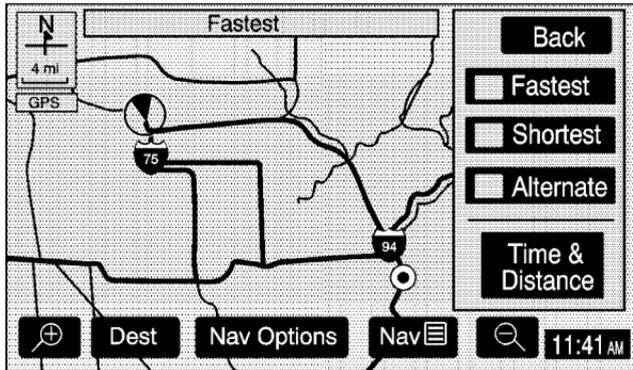
After selecting one of the three routes, the road distance and estimated travel time will be displayed. The Fastest route means you will be routed along main roads and highways, but does not necessarily mean it is the shortest route. You may also touch the Time & Distance screen button to view the road distance and estimated travel time for each of the three routes.
