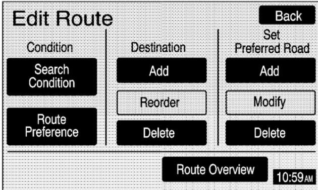
**Condition:** The Search Condition screen allows you to select your route preference by choosing from Fastest, Shortest, or Alternative route. By selecting the Fastest route, you will be routed along main roads and highways, which does not necessarily mean it will be the shortest route.
