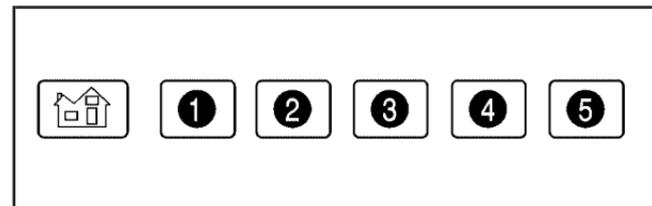
These presets, along with the home symbol preset, are located at the bottom of each page of the Destination menu. Besides the home preset destination and Emergency destination entry method, these are the only presets available for selection while the vehicle is moving.
