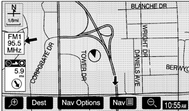
The following touch-sensitive screen buttons will appear frequently at the bottom of a map screen.
