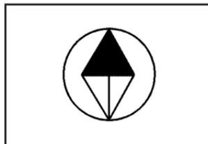
This symbol indicates that the map is shown with the vehicle travel direction up, known as Heading Up mode.
