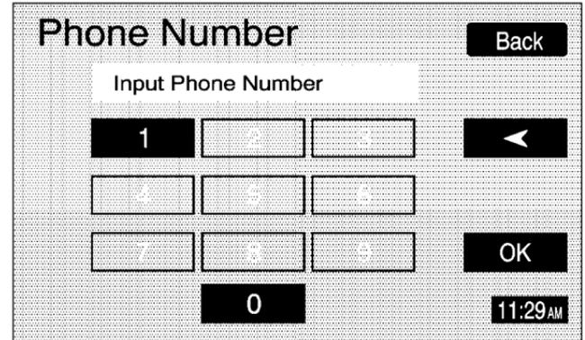
Enter the POI phone number on the numeric keypad and touch the OK screen button. The destination location will then be displayed. Most phone numbers for POIs included in the DVD database can be entered to locate a destination. Cellular phone numbers and internal company phone numbers cannot be entered to locate a destination.
