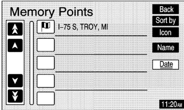
Memory points include up to 30 saved points, five preset destinations, and a home location. Selecting the Memory Points screen button from the Destination screen allows you to select any one of the marked points as the active destination. Marked points can also be sorted by icon, date saved, or alphabetically.
