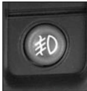
The fog lamp button is located on the left side of your instrument panel.
