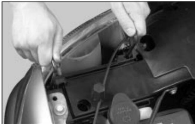
1. Remove the two pins on the top of the headlamp assembly. To remove the pins, turn the outer pin outward and pull it straight up. To remove the inner pin, turn it inward and pull it straight up.
