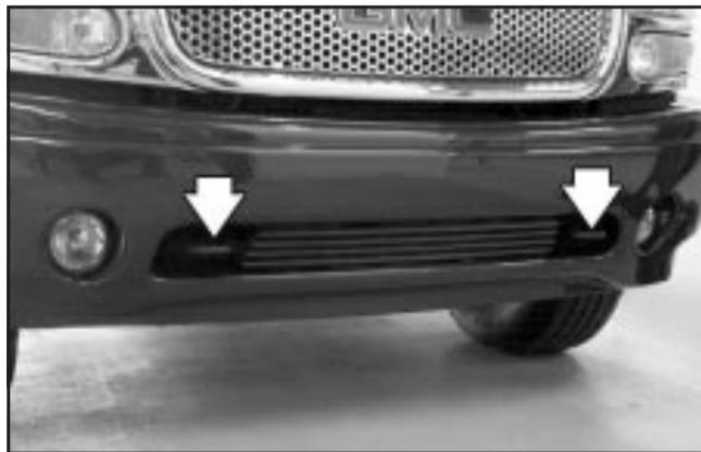
Your vehicle is equipped with recovery hooks. The hooks are provided at the front of your vehicle. You may need to use them if you are stuck off-road and need to be pulled to some place where you can continue driving.
