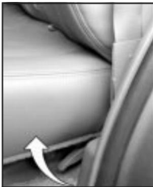
2. Pull the seatback release lever upward and pull the seatback up and fold it down until it is flat.
