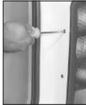
1. Remove the two screws from the rear lamp assembly.
