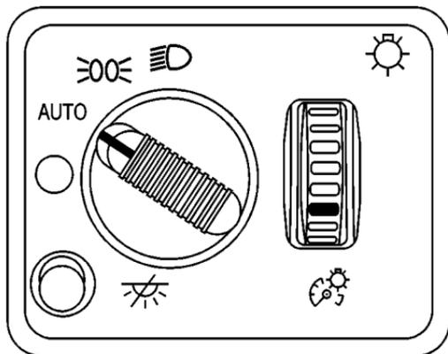
The control on the driver's side of your instrument panel operates the exterior lamps.
