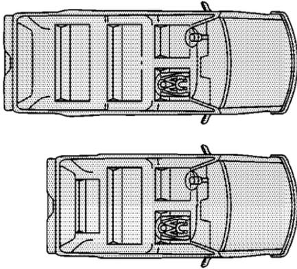
Your vehicle has a right front passenger air bag. A rear seat is a safer place to secure a forward-facing child restraint. See *Where to Put the Restraint* on page 1-56.
