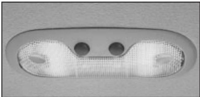
Your vehicle may also have reading lamps in other locations. To turn on or off, press the button located next to the lamp. The lamps are fixed and cannot be adjusted.
