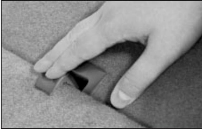
1. Release the panels from the seatbacks by pushing forward on the latches.
