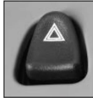
The hazard warning flasher button is located at the top of the steering column.
