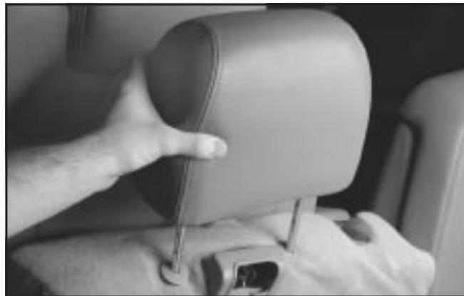
Pull the headrest out from the seatback and slide the pins into the holes provided in the top of the seat cushion.
