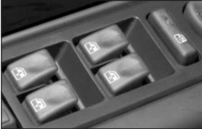
The driver's door has a switch for the passenger's windows as well. Your power windows will work when the ignition has been turned to ACCESSORY or RUN or when Retained Accessory Power (RAP) is active. See *Ignition Positions on page 2-19*.
