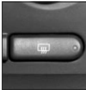
When you press this button, a defogger warms the heated driver's and passenger's outside rearview mirrors to help clear them of ice, snow and condensation.
