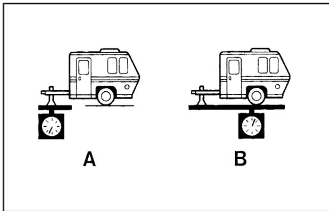
The trailer tongue weight (A) should be 10 percent to 15 percent of the total loaded trailer weight (B), up to a maximum of 600 lbs. (272 kg) with a weight carrying hitch. The trailer tongue weight (A) should be 10 to 15 percent of the total loaded trailer weight, up to a maximum of 1,000 lbs. (453 kg) with a weight distributing hitch.
