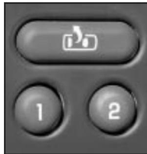
If your vehicle has this feature, then the controls for the memory function are located on the driver's door.
