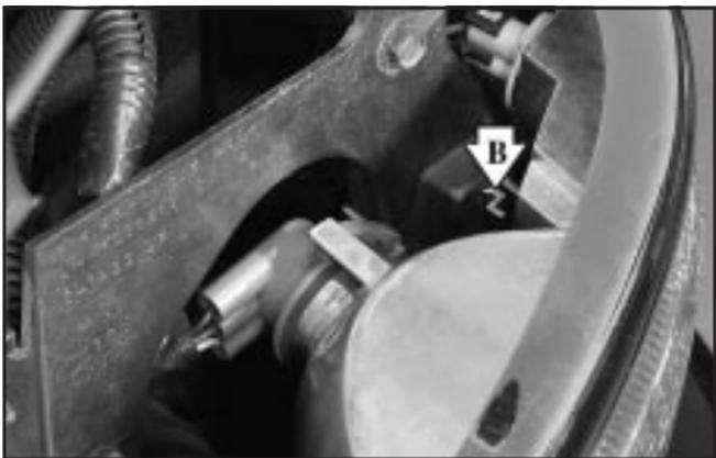
2. Press the retainer clip (B), located behind the turn signal housing, towards the outside of the vehicle.
