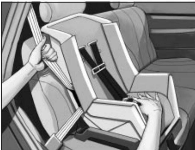
5. To tighten the belt, feed the shoulder belt back into the retractor while you push down on the child restraint. If you're using a forward-facing child restraint, you may find it helpful to use your knee to push down on the child restraint as you tighten the belt.
