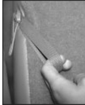
1. Pull up on the release lever labeled 1 and then pull up on the seatback or the assist strap located on the outboard side of the seat until the seatback locks into the upright position.
