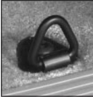
Your vehicle may be equipped with cargo tie downs in the rear cargo area that allow you to strap cargo in and keep it from moving inside the vehicle.
