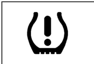
If your vehicle is equipped with the Tire Pressure Monitor system, this light will come on if the system detects low tire pressure.
