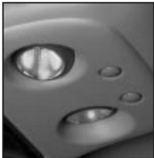
If your vehicle has reading lamps, press the button located next to the lamp to turn it on or off. The lamps can be adjusted to point in the direction you want.
