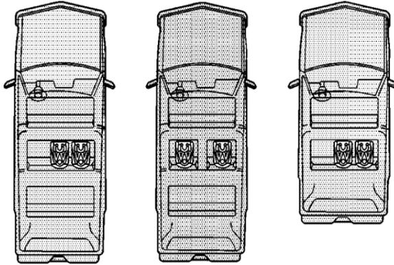
Your vehicle has the LATCH system. You will find anchors (A) in the center and right side passenger second row seating positions for bench seats, and the outboard passenger positions for bucket seats.
