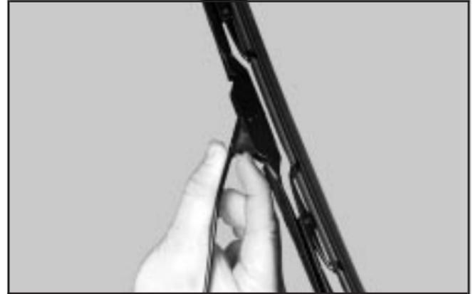
2. Push the release lever and slide the wiper assembly toward the driver's side of the vehicle.
