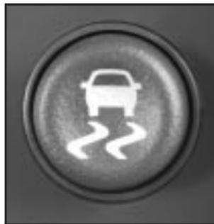
Stabilitrak<sup>®</sup> and part of the traction control system can be turned off or back on by pressing the Stabilitrak<sup>®</sup> button located on the instrument panel.
