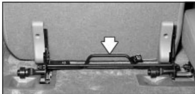
4. Squeeze the release handle while pulling the seat out.
