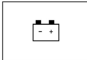
The charging system light will come on briefly when you turn on the ignition, but the engine is not running, as a check to show you it is working.
