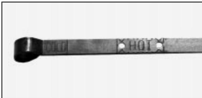
3. Check both sides of the dipstick, and read the lower level. The fluid level must be in the COLD area, below the cross-hatched area, for a cold check or in the HOT area or cross-hatched area for a hot check. Be sure to keep the dipstick pointed down to get an accurate reading.
