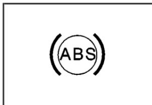
If there is a problem with the anti-lock brake system, this warning light will stay on. See *Anti-Lock Brake System Warning Light* on page 3-37.
