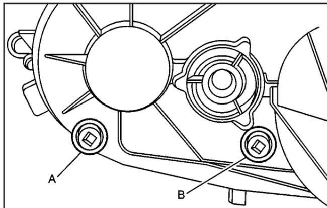
(A) Drain Plug (B) Filler Plug
