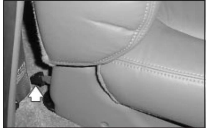
1. Lift the release lever on the back of the seat.
