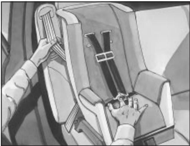
6. To tighten the belt, push down on the child restraint, pull the shoulder portion of the belt to tighten the lap portion of the belt and feed the shoulder belt back into the retractor. If you are using a forward-facing child restraint, you may find it helpful to use your knee to push down on the child restraint as you tighten the belt. You should not be able to pull more of the belt from the retractor once the lock has been set.
