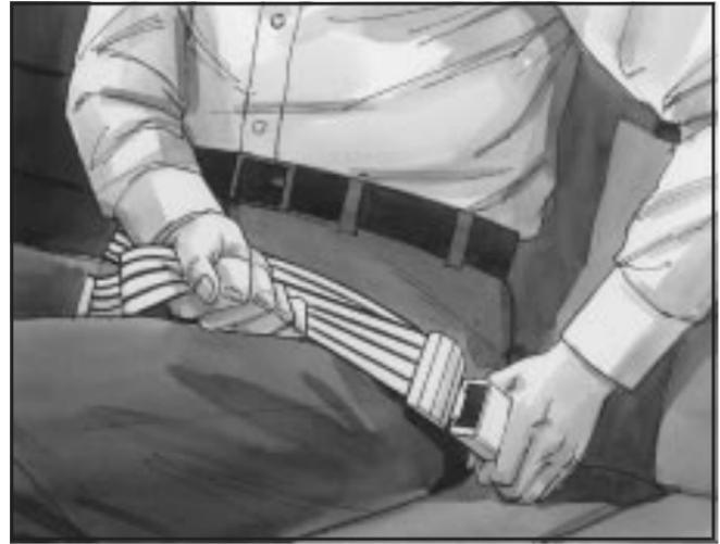
To make the belt shorter, pull its free end as shown until the belt is snug. Buckle, position and release it the same way as the lap part of a lap-shoulder belt. If the belt is not long enough, see *Safety Belt Extender* on page 1-47.
