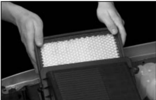
1. Loosen the screws on the cover of the housing and lift up the cover.
