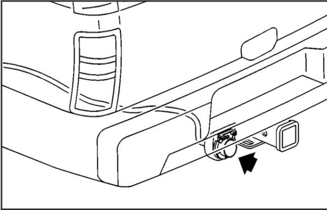
Your vehicle is equipped with the seven-wire trailer towing harness. This harness with a seven-pin universal heavy-duty trailer connector is attached to a bracket on the hitch platform.
