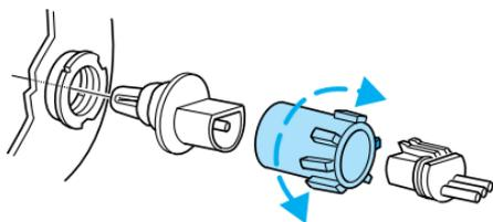
7. Remove the old bulb from its socket by gently pulling it straight back out of the socket. Do not turn the bulb while removing it.
