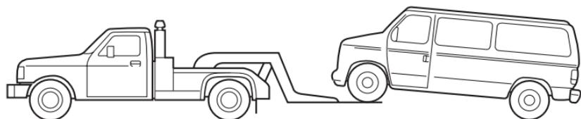
If you need to have your vehicle towed, contact a professional towing service or, if you are a member, your roadside assistance center. It is recommended that your vehicle be towed with a wheel lift or flatbed equipment.
