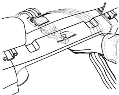
Do not clip the tether strap to the seat pedestal as shown.
