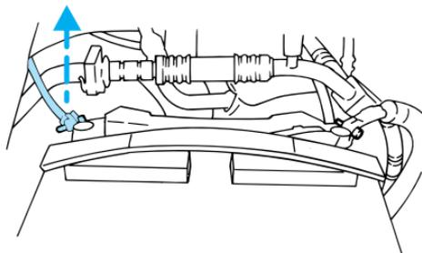
2. Disconnect the auxiliary battery frame ground.
