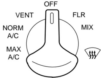
The air conditioning compressor will operate in all modes except VENT and FLR. However, the air conditioning will only function if the outside temperature is about 10°C (50°F) or above.
