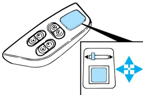
3. Return to the center position to lock mirrors in place.
