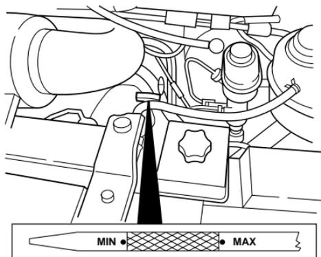
6. Wipe the indicator clean. Insert the indicator fully, then remove it again.
