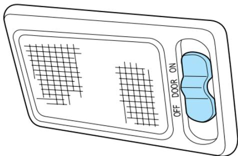
When the cargo lamp switch is in the OFF position, it will not illuminate when you open the doors or turn the headlamp control.
