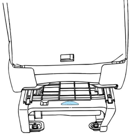
3. Route the child safety seat tether strap over the back of the front right-hand passenger seat as shown.
