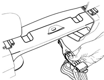
5. Rotate the tether strap as shown.
