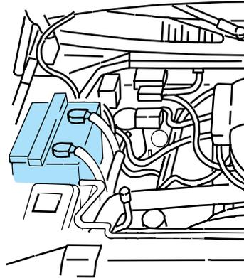
Keep the electrolyte level in each cell up to the level indicator. Do not overfill.
