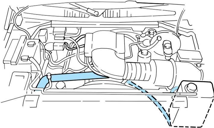
Inspect all engine and heater system hoses and hose connections for:
