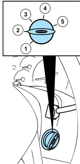
**1 (Accessory)** - allows electrical accessories such as the audio system and wiper/washer to operate when the engine is not running.
