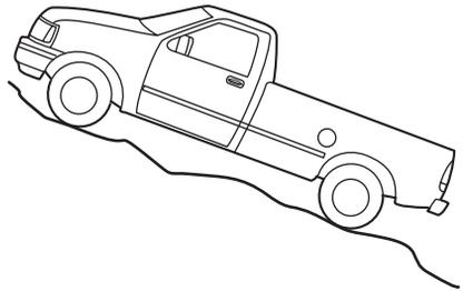
When climbing a steep hill, start in a lower gear rather than downshifting to a lower gear from a higher gear once the ascent has started. This reduces strain on the engine and the possibility of stalling.
