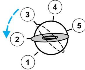
3. Turn ignition key to Lock and remove the key.
