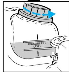
Check the coolant level in the coolant recovery reservoir the next few times you drive the vehicle. If necessary, add enough of a 50/50 mixture of coolant and water to bring the liquid level to the fill line on the reservoir.
