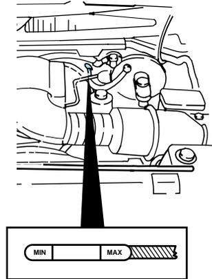
5. Wipe the dipstick clean. Insert the dipstick fully, then remove it again. The oil level should be in the range shown on the dipstick.
