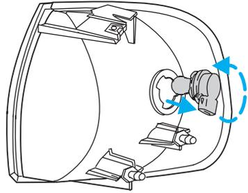
3. Remove the electrical connector from the bulb by grasping the wire and pulling it rearward.
