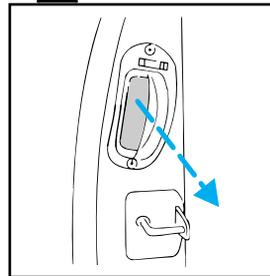
To open the third door (the passenger door must be open) pull either the handle located in the
