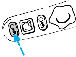
Press switch to tilt the rear of the seat up or down.
