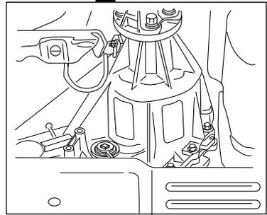
3. Add only enough fluid through the filler opening so that the fluid level is at the bottom of the opening.
