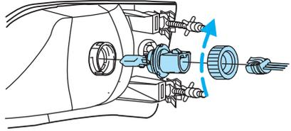
5. Remove the electrical connector from the bulb by grasping the wire and pulling it rearward.
