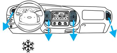
The A/C mode directs outside air conditioned air to flow through the instrument panel vents. The A/C mode can be used for heating, ventilating and defogging the windows or air conditioning. The A/C mode only functions if the outside temperature is above 10°C (50°F).
