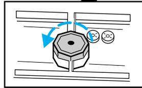
3. Fluid level should be at bottom of the opening.
