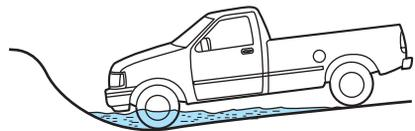
When driving through water, determine the depth; avoid water higher than the bottom of the hubs (if possible) and proceed slowly. If the ignition system gets wet, the vehicle may stall.
