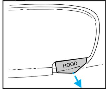
2. While applying downward pressure on the hood, push the hood latch handle located just left of the center of the hood.
