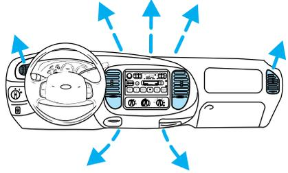
The FLR & DEF position directs outside air to flow through the floor vents and the windshield defroster vents. The air conditioning will function to defog the windows provided the outside temperature is above 10°C (50°F).
