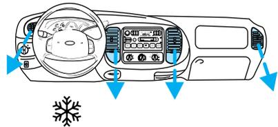
The MAX A/C mode recirculates the cabin air and directs it to flow through the instrument panel vents. The MAX A/C mode can be used for air conditioning or heating. This mode is noisier but more economical than the A/C mode. The MAX A/C mode only functions if the outside temperature is above 10°C (50°F).
