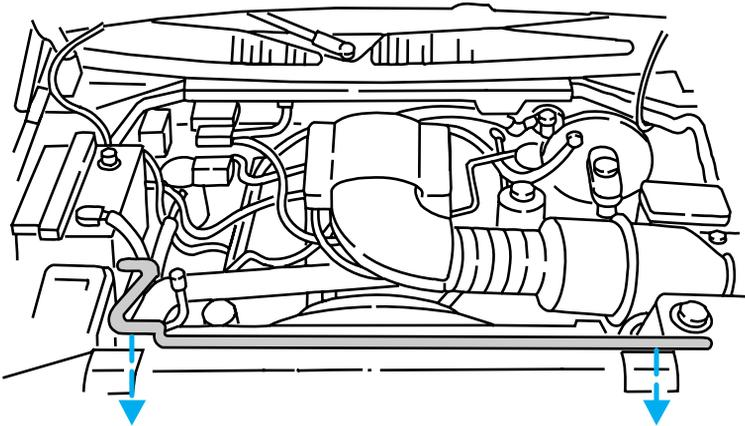
1. Carefully remove the jack handle from the retaining clips (above radiator in engine compartment).
