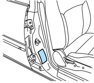
The cold pressure amount is listed on the Safety Compliance Certification Label located on the inside driver door latch pillar.
