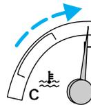
If you are driving more than 24 km (15 miles) at temperatures above freezing, angle the plow blade either full left or full right to provide maximum airflow to the radiator.
