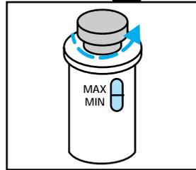
3. Visually inspect the fluid level in the power steering fluid reservoir.
