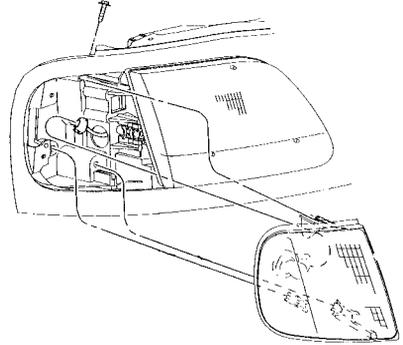
9. Align top and bottom ribs of parking lamp assembly with corresponding slots on front of vehicle.
