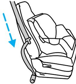
3. While holding the shoulder and lap belt portions together, route the tongue through the child seat according to the child seat manufacturer's instructions. Be
