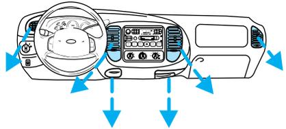
The PANEL & FLOOR position directs outside air to flow between the panel and floor vents. The air conditioning will function to provide cooling and dehumidification when the outside temperature is above 10°C (50°F).
