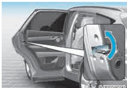
In case of an emergency such as when the battery is discharged, the only way to lock the door(s) is with the mechanical key from the outside key hole.
