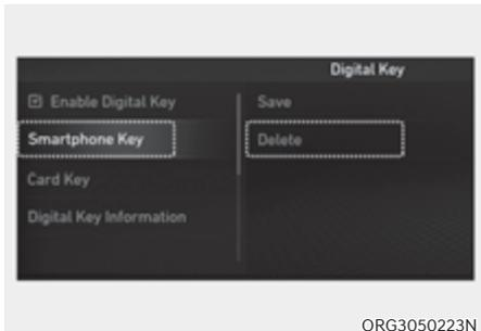
2. From the infotainment system settings menu, select 'Setup → Vehicle → Digital Key → Smartphone key → Delete'. The 'Delete' menu will be disabled if there is no digital key (smart phone) saved.
