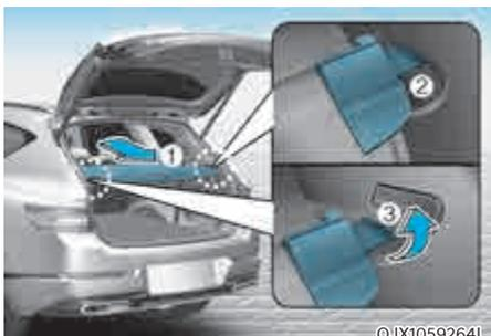
1. Pull the cargo security screen towards the rear of the vehicle by the handle (1).
