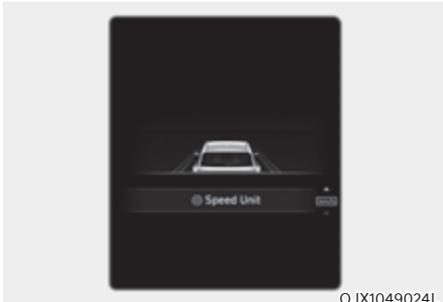
When the Speed Unit menu is selected, press the OK switch on the steering wheel. You can change the speed unit setting between MPH and km/h for the cluster.
