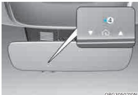
4. Press the Original Transmitter button until the indicator (4) is turned continuously ON or flashes in Green for approximately 10 seconds and it indicates the programming is completed.
