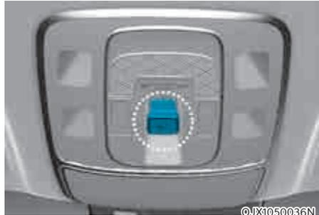
The sunroof can only be opened, closed, or tilted when the Engine Start/Stop button is in the ON position.
