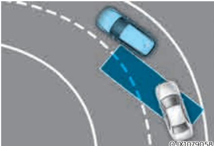
Blind-Spot Safety system may not operate properly when driving on a curved road. The system may recognize a vehicle in the same lane.
