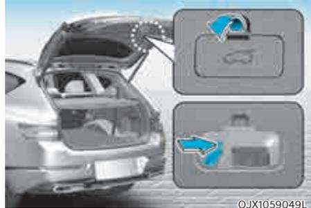
To unlock and open the liftgate manually from inside the luggage compartment, perform the following procedure:
