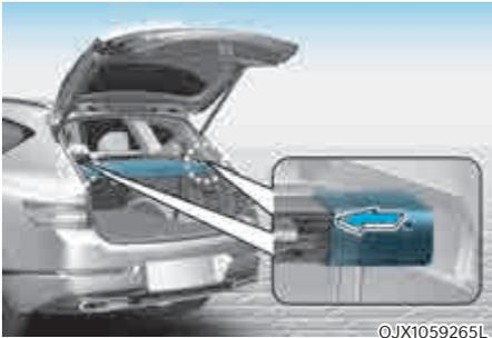
1. Push one side of the cargo screen inward to compress the spring and release the screen from the vehicle.
