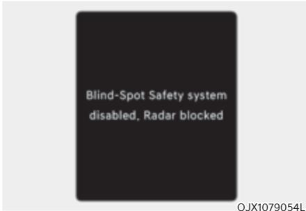
When the rear bumper around the rear corner radar or sensor is covered with foreign material, such as snow or rain, or installing a trailer or carrier, it can reduce the detecting performance and temporarily limit or disable Blind-Spot Safety system.
