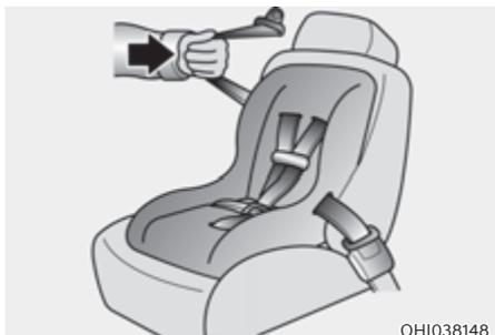
4. Slowly allow the shoulder portion of the seat belt to retract and listen for an audible "clicking" or "ratcheting" sound. This indicates that the retractor is in the "Automatic Locking" mode. If no distinct sound is heard, repeat steps 3 and 4.
