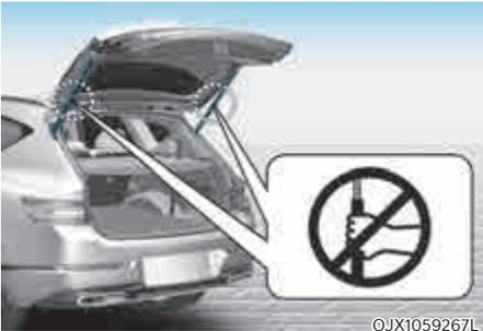
Do not hold on to or try to pull on the liftgate strut. Be aware that the deformation of the liftgate strut may cause vehicle damage and risk of injury.
