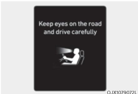
Forward Attention Warning helps determine whether the driver is focused on the road depending on information, such as the amount of time the driver is looking elsewhere, the amount of time the eyes are closed, how frequently the driver yawns, etc. If the system judges the driver is not focused, the 'Keep eyes on the road and drive careful' warning message will appear on the cluster, and an audible warning will sound.
