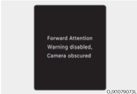
When there is an object right in front of the camera or between the driver and the camera for a certain period of time, Forward Attention Warning will not operate properly, and the 'Forward Attention Warning disabled. Camera obscured' warning message will appear on the cluster.
