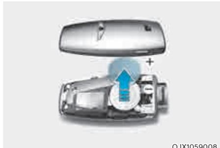
2. Remove battery cover using a phillips screwdriver.
