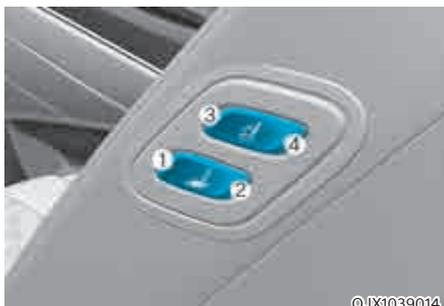
The rear seat passenger may use the switches to control the front passenger seat.
