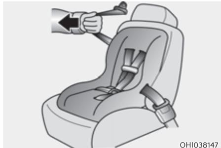
3. Pull the shoulder portion of the seat belt all the way out. When the shoulder portion of the seat belt is fully extended, it will shift the retractor to the "Automatic Locking" (child restraint) mode.
