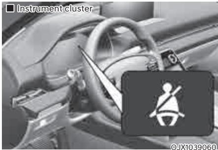
As a reminder to the driver, the seat belt warning light will illuminate for approximately 6 seconds each time the Engine Start/Stop button is in the ON or START position regardless of belt fastening.
