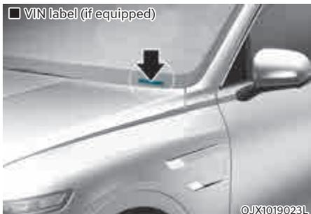
The VIN is also on a plate attached to the top of the left side dashboard. The number on the plate can easily be seen through the windshield from outside.
