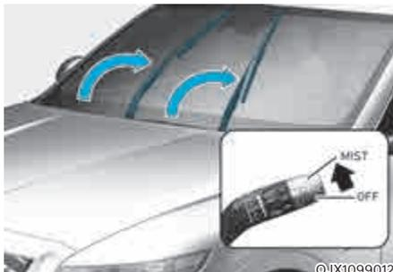
1. Within 20 seconds of turning off the engine, lift up and hold the wiper lever to the MIST position for about 2 seconds until the wipers move to the top wipe position.
