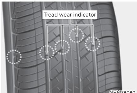
If the tire is worn evenly, a tread wear indicator will appear as a solid band across the tread. This shows there is less than 1/16 inch (1.6 mm) of tread left on the tire. Replace the tire when this happens.
