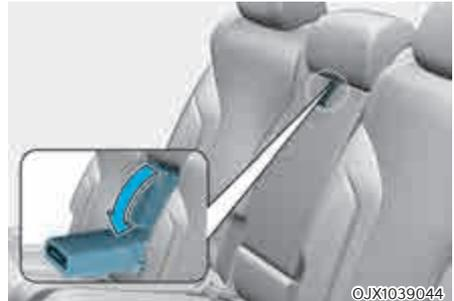
The armrest is located in the center of the rear seat. Pull the armrest down by using the strap from the seatback to use it.
