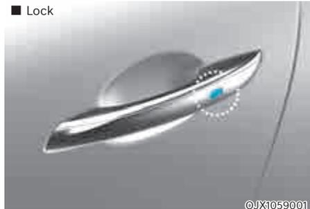
Touch the touch sensor on the front outside door handle (the engraved part) while carrying the Smart Key with you or press the Door Lock button on the Smart Key, all doors will lock.
