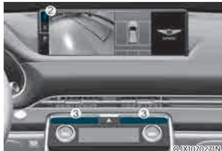
Surround View Monitor will assist in parking by allowing the driver to see around the vehicle.
