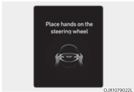
If the driver takes their hands off the steering wheel for several seconds, the 'Place hands on the steering wheel' warning message will appear and an audible warning will sound in stages.
