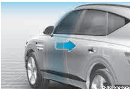
If a door isn't closed completely but is closed to the first detent position, the door will close automatically.
