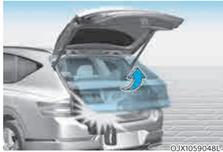
During power opening or closing if the power liftgate senses any obstacle, the power liftgate will stop and move in the opposite direction.
