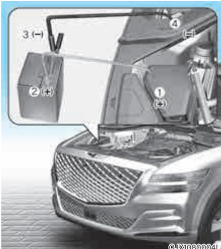
7. Connect the jumper cables in the exact sequence shown in the illustration. First connect one jumper cable to the red, positive (+) jumper terminal of your vehicle (1).
