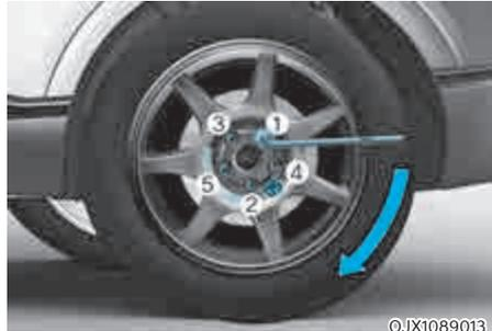
16. Use the wheel lug wrench to tighten the wheel bolts in the order shown. Double-check each wheel bolts until they are tight. After changing tires, have an authorized retailer of Genesis Branded products tighten the wheel bolts to their proper torque as soon as possible. **The wheel bolt should be tightened to 101–116 lbf.ft (14–16 kgf.m).**
