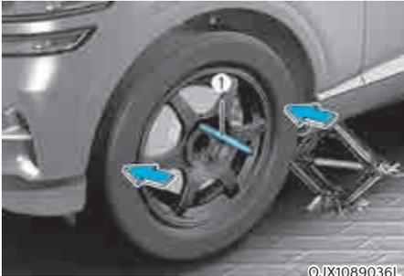
12. Install the spare tire over the centering pin (1) and then push in the spare tire.
