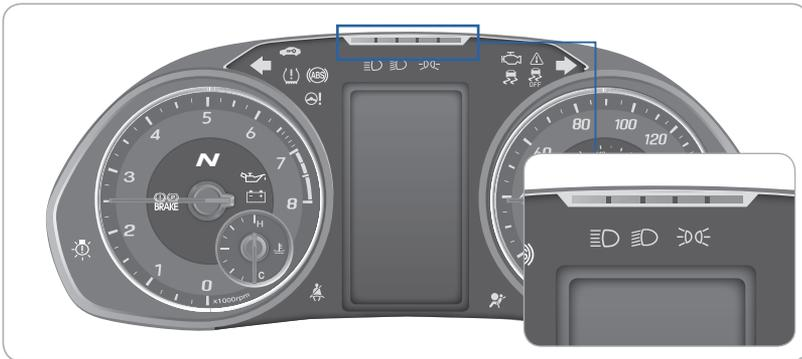
The number of LEDs illuminated indicates the relevant engine speed. Different colored LEDs will be illuminated as engine speed nears the maximum allowed speed. When all 5 LEDs start blinking, it indicates the best time to initiate upshift operation.
