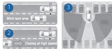
The BCA (Blind-Spot Collision-Avoidance Assist) system uses a radar sensor to alert the driver while driving. It monitors the rear area of the vehicle and provides information to the driver.
