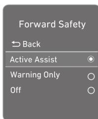
Forward Collision-Avoidance Assist (FCA) system is designed to help detect and monitor the vehicle ahead in the roadway through camera recognition to warn the driver that a collision is imminent, and if necessary, apply emergency braking.
