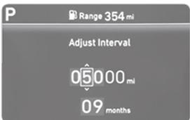
This system is designed to notify you of your next vehicle maintenance interval.
