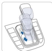
Shift the lever from D into the manual gate to activate manual shift mode. Manual shift mode is a recalibrated automatic mode that will hold gears longer and downshift at higher RPM for a more dynamic driving style.
