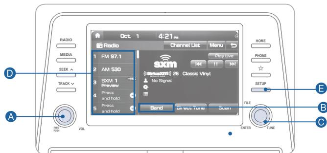
Press POWER button **A** to turn radio on.
