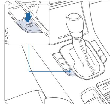
The drive mode may be selected according to the driver's preference or road condition. The system resets to NORMAL mode every time the engine is restarted. Each time you press the button, the drive mode changes as following :
