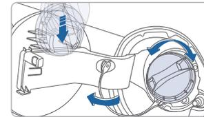
2. Remove the fuel tank cap.
