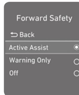
The Forward Collision Avoidance (FCA) system is designed to detect and monitor the vehicle ahead and warn the driver if a collision is imminent. On vehicles equipped with both camera and radar sensor, pedestrian detection is also available.
