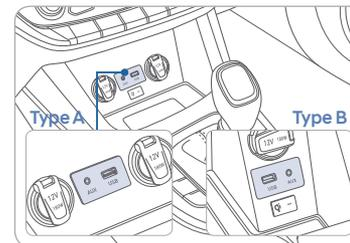
Use the AUX or USB ports to connect an external audio device and listen to it through the audio system in your vehicle.
