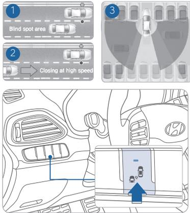
The Blind Spot Detection system uses radar sensors to monitor and warn the driver of an approaching vehicle in the driver's blind spot area.
