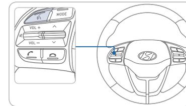
Press button on the steering wheel control to activate voice recognition.
