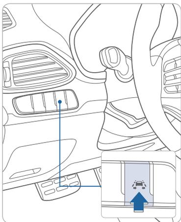
The Lane Keeping Assist System detects lane markers on the road, and assist the driver's steering to help keep the vehicle between lanes.
