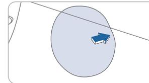
1. Push the center edge of the fuel filler door when the driver's door is unlocked.
