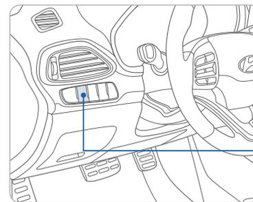
Press the illumination control button to adjust the instrument cluster illumination brightness.
