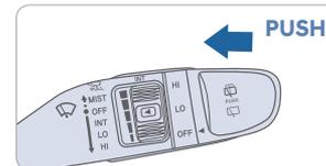
**Rear:** Push the lever away from you to spray washer fluid on the rear window and run the wiper briefly.
