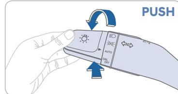
**NOTE:** To turn off the high beam, pull the lever towards you.
