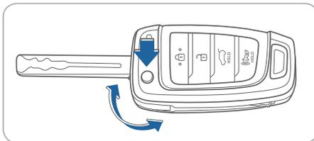
To unfold the mechanical key, press the release button on the remote.
