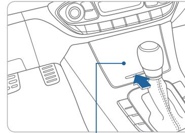
There is a wireless cellular phone charging system inside the front console. The system operates with all doors closed, and the ignition switch is in the ACC/ON position.
