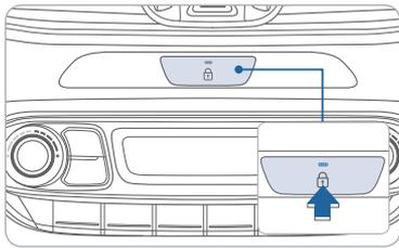
Press the central door lock/unlock switch to lock/unlock all vehicle doors. All doors must be closed to use the central door lock switch.
