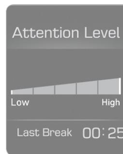
The Driver Attention Warning System (DAW) system displays the condition of the driver's fatigue level and inattentive driving practices. The DAA system monitors the lane markers and driver's inputs to the steering wheel, accelerator pedal and brake pedal.
