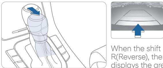
When the shift lever is moved to R(Reverse), the rear view camera displays the area behind the vehicle.
