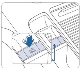
The Auto Hold feature assists in hilly areas. It applies the brake until the accelerator pedal is pressed.
