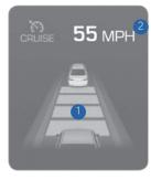
The system assists you in setting the distance from the vehicle ahead and will maintain the selected distance without having to press on the accelerator or the brake pedal.
