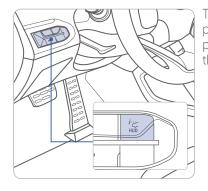
To activate the Heads-Up Display, press the HUD button on the dash panel located on the left-hand side of the driver.
