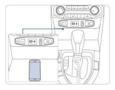
There is a wireless cellular phone charging system inside the front console. The system operates with all doors closed, and the ignition switch is in the ACC/ON position.
