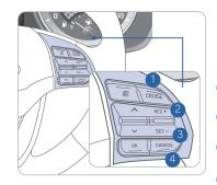
The Cruise Control system allows you to program the vehicle to maintain a constant speed without pressing the accelerator pedal.
