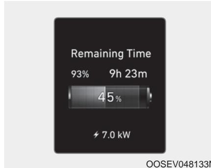
9. After charging has started, the estimated charging time is displayed on the instrument cluster for about 1 minute.
