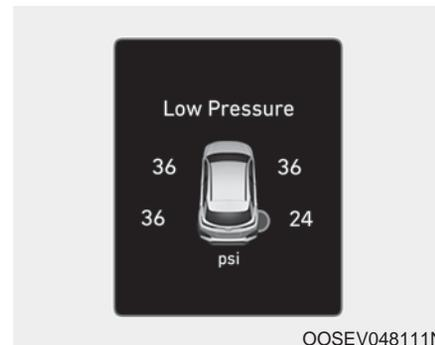
This warning message is displayed if the tire pressure is low. The display will indicate which of the tires has low tire pressure and what is the approximate tire pressure value.
