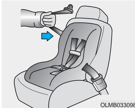
5. Slowly allow the shoulder portion of the seat belt to retract and listen for an audible "clicking" or "ratcheting" sound. This indicates that the retractor is in the "Automatic Locking" mode. If no distinct sound is heard, repeat steps 3 and 4.
