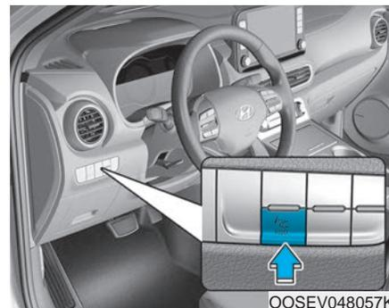
Use the button on the left hand side of the dash panel to activate/deactivate the Head-up display when the the POWER button is in the ON position or when the vehicle is in the ready (
