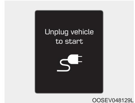
This message is displayed when you start the vehicle without unplugging the charging cable. Unplug the charging cable, and then turn on the vehicle.
