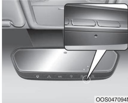
1. Press and release the Control Button within 1 second to turn the display feature OFF.
