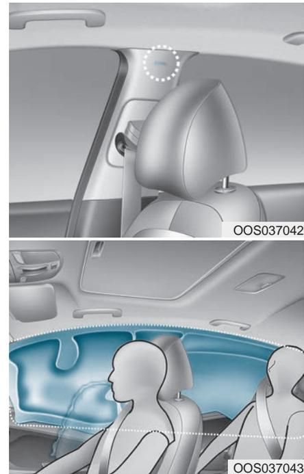
Curtain air bags are located along both sides of the roof rails above the front and rear doors.
