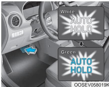
2. When you stop the vehicle completely by depressing the brake pedal, Auto Hold maintains the brake pressure to hold the vehicle stationary. The indicator changes from white to green.
