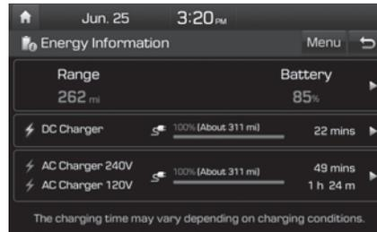
You can check the vehicle expected range, total battery power remaining, and expected charging time for each charge type.
