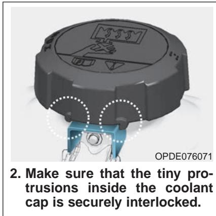
**2. Make sure that the tiny protrusions inside the coolant cap is securely interlocked.**
