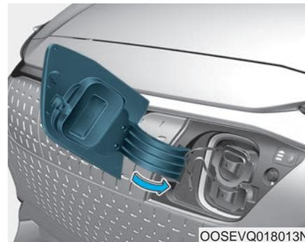
1. After recharging, make sure to install the charging port dust cover(s) before closing the charging door.
