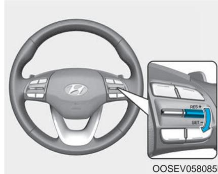
3. Push the toggle switch down (SET-). The Set Speed and Vehicle-to-Vehicle Distance on the LCD display will illuminate.
