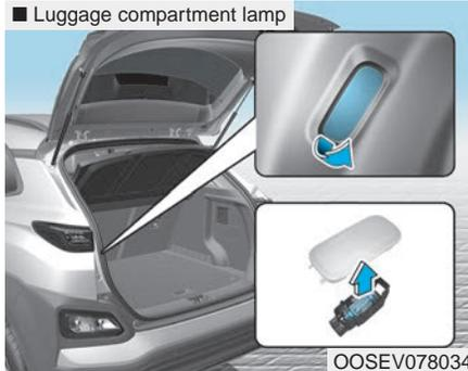
1. Using a flat-blade screwdriver, gently pry the lens from the interior lamp housing.
