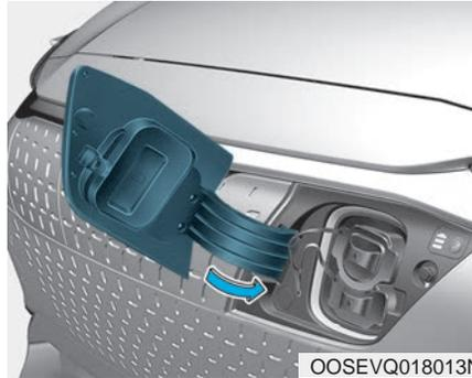
2. Make sure to re-install the charging port dust cover(s) before closing the charging door.
