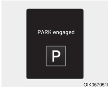
The message appears on the LCD display when the P (Park) position is engaged.
