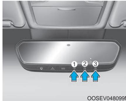
3. Press and release the programmed HomeLink button to activate the garage door.
