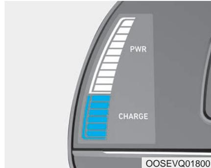
The Power/Charge gauge shows the energy consumption rate of the vehicle and the charge/discharge status of the regenerative brakes.
