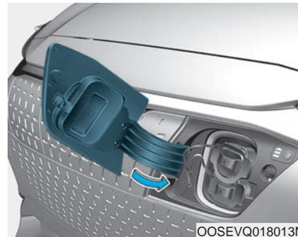
2. Make sure to re-install the charging port dust cover(s) before closing the charging door.
