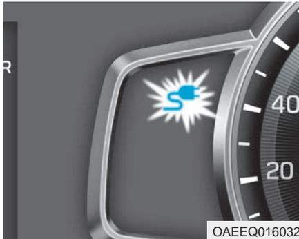
10. Check to see that the charging indicator light in the instrument cluster is illuminated. Charging has not been initiated if the charging indicator light is OFF.
