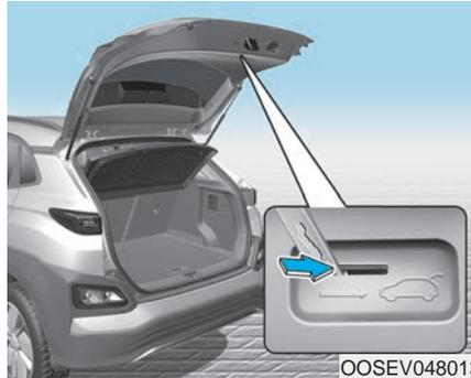
To unlock and open the liftgate manually from inside the luggage compartment, perform the following steps:
