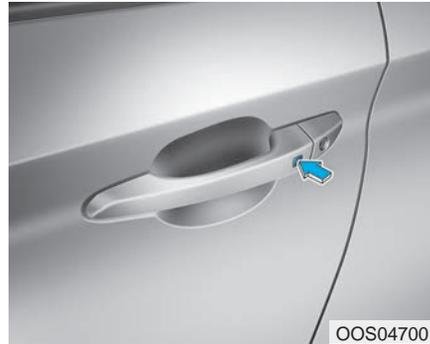
To lock your vehicle using the door handle button or the Smart Key:
