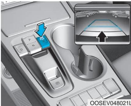
The Rear View Monitor will activate when the vehicle is in the ready (🚗) mode and the gear is in the R (Reverse) position.
