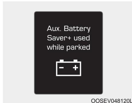
This message is displayed when the Aux. Battery Saver+ function has been operating while the vehicle was turned off.
