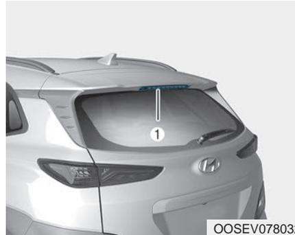
If the LED lamp (1) does not operate, have the system checked by an authorized HYUNDAI dealer.
