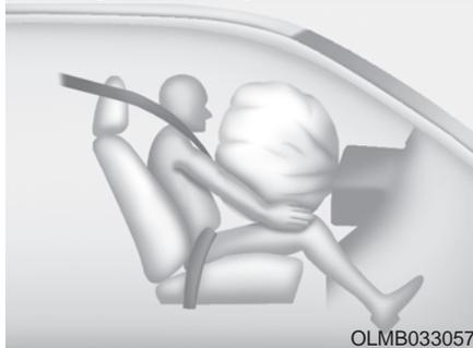
After complete inflation, the air bag immediately starts deflating, enabling the driver to maintain forward visibility and the ability to steer or operate other controls.
