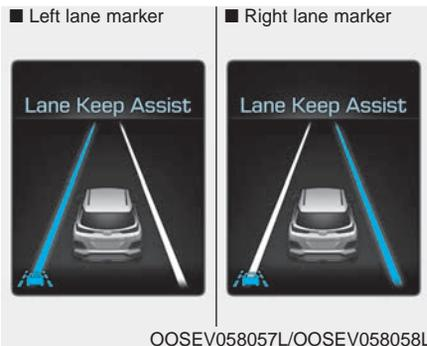
1. A visual warning appears on the cluster LCD display. Either the left lane marker or the right lane marker in the cluster LCD display will blink depending on which direction the vehicle is veering. Also, a warning sound will be heard.
