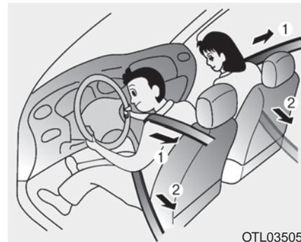
Your vehicle is equipped with driver's and front passenger's Pre-tensioner Seat Belts (Retractor Pretensioner and Emergency Fastening Device System). The purpose of the pre-tensioner is to make sure the seat belts fit tightly against the occupant's body in certain frontal or side collision(s). The Emergency Fastening Device System may be activated in certain crashes where the frontal or side collision(s) is severe enough, together with the air bags.
