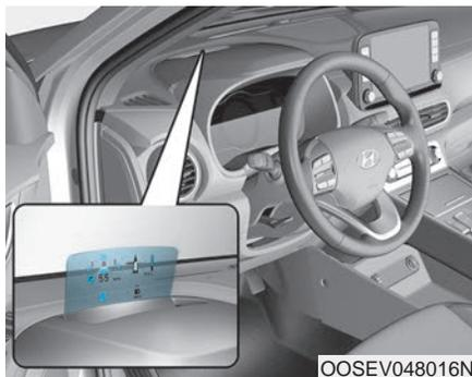
The Head-Up Display is an optional feature that allows the driver to view information projected onto a transparent screen while still keeping your eyes safely on the road ahead while driving.
