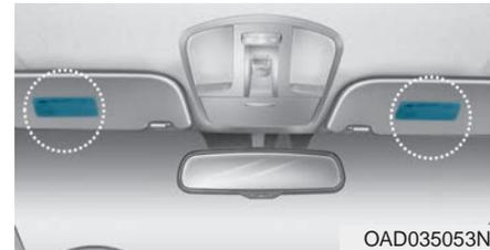
Air bag warning labels, required by the U.S. National Highway Traffic Safety Administration (NHTSA), are attached to alert the driver and passengers of potential risks of the air bag system. Be sure to read all of the information about the air bags that are installed on your vehicle in this Owners Manual.
