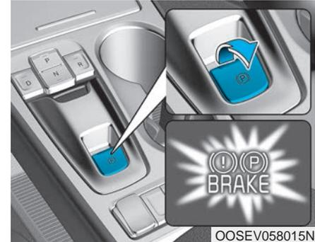
**To apply the EPB (Electronic Parking Brake):**
