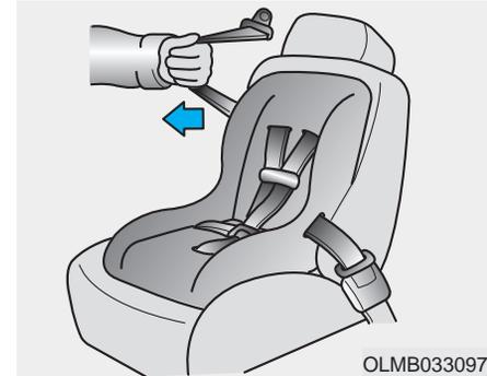
4. Pull the shoulder portion of the seat belt all the way out. When the shoulder portion of the seat belt is fully extended, it will shift the retractor to the "Automatic Locking" (child restraint) mode.
