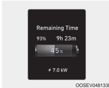
11. After charging has started, the estimated charging time is displayed on the instrument cluster for about 1 minute.
