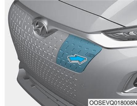
3. Unlock the vehicle before opening the charging door. From the outside the vehicle, push on the charging door in the area indicated by the arrow to open the door.
