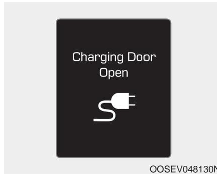
This message is displayed when you attempt to shift the vehicle out of P (Park) with the charging door open. You must close the charging door before driving the vehicle.
