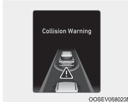
This warning message appears on the LCD display with a warning chime. Additionally, some vehicle system intervention occurs to help decelerate the vehicle.
