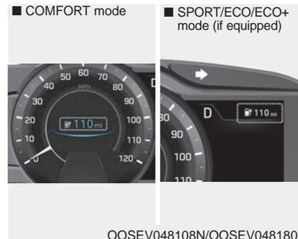
The location of where the vehicle range is displayed is different depending on which drive mode is active.
