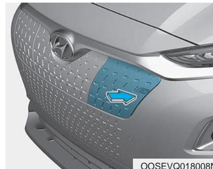
5. Unlock the vehicle before opening the charging door. Push on the charging door in the area indicated by the arrow to open the door.
