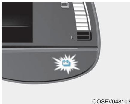
When there are only 2 bars remaining on the gauge, the SOC level is low. The warning lamp turns ON to alert you that the battery must be charged soon.
