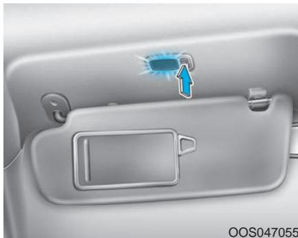
Push the switch to turn the light on or off.
