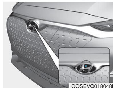
**When the function is activating the indicator lamp will illuminate and high voltage electricity will be flowing in the vehicle. Do not touch the high voltage electric wire (orange), connector, and all electric components and devices. This may cause electric shock and lead to injuries. Also, do not modify your vehicle in any way. This may affect your vehicle performance and lead to an accident.**
