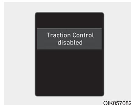
Press the ESC OFF button briefly. The ESC OFF indicator light and message "Traction Control disabled" will illuminate. In this state, the traction control function of ESC is disabled, but the brake control function of ESC still operates.
