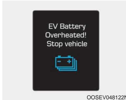
This warning message is displayed to protect battery and electric vehicle system when the high voltage battery temperature is too high.
