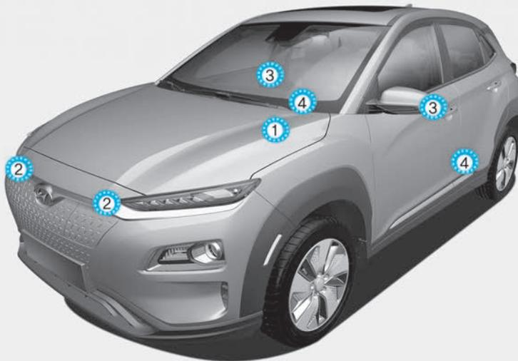
1. SRS control module/Rollover sensor
