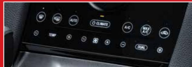
Press **AUTO** to switch on automatic operation. Adjust to select your desired temperature. Fan speed, air distribution, air conditioning operation and outside or recirculated air automatically adjust to heat or cool the vehicle, maintaining the desired temperature.
