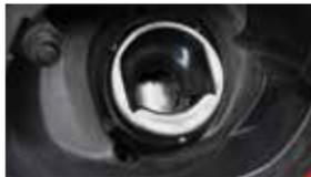
If you are refilling your tank from a fuel container, make sure you use the fuel filler funnel included with your vehicle. Using an aftermarket funnel may not work with the capless system and could cause damage to your vehicle. For more information and for your fuel filler funnel location, please see the *Fuel and Refueling* chapter in your *Owner's Manual*.
