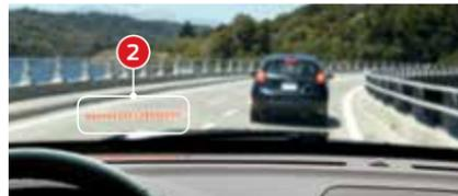
This system alerts the driver of certain collision risks. Radar sensors detect if vehicles ahead of you, moving in the same direction, may be a collision risk. The system alerts you with an audible tone and a red warning light **2** appears above the instrument panel. If the risk of collision increases, the system then increases brake support to help reduce collision speed.
