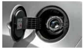
If you are refilling your tank from a fuel container, make sure you use the fuel filler funnel included with your vehicle. Using an aftermarket funnel may not work with the capless system and could cause damage to your vehicle. For more information and for your fuel filler funnel location, please see the **Fuel and Refueling** chapter of your **Owner's Manual**.
