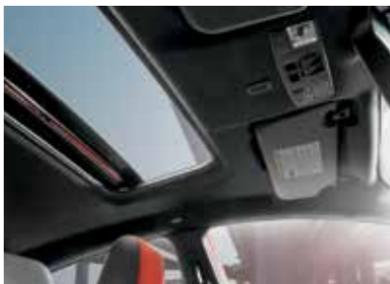
The moonroof controls are on the overhead console and have a one-touch open and close feature. To stop its movement during one-touch operation, press the control a second time. Press and release the rear of the **SLIDE** control to open the moonroof. Press and hold the front of the **SLIDE**
