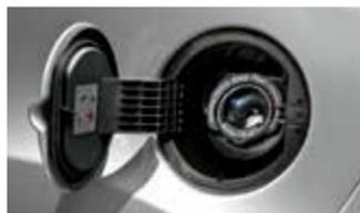
If you are refilling your tank from a fuel container, make sure you use the fuel filler funnel included with your vehicle. Using an aftermarket funnel may not work with the capless system and could cause damage to your vehicle. For more information and for your fuel filler funnel location, please see the **Fuel and Refueling** chapter of your **Owner's Manual**.
