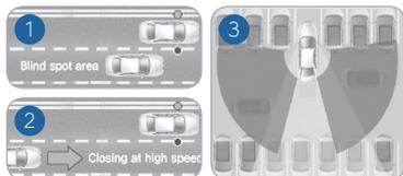
The BSD (Blind Spot Detection) system uses a radar sensor to alert the driver while driving. It senses the rear side territory of the vehicle and provides information to the driver.
