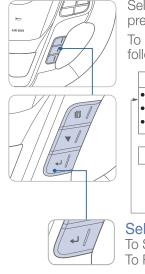
Select "Trip Computer" mode by pressing the MODE button **1**. To change the trip mode as follows, press the MOVE button ▼. **TRIP A** •Tripmeter [A] •Average Vehicle Speed [A] •Elapsed Time [A]
