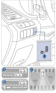
The BSD system sensor senses the rear side territory of the vehicle and provides information to the driver. Press the BSD switch. The indicator will illuminate on the button. If vehicle speed exceeds 9mph the system will activate. Press the switch again to deactivate the system.
