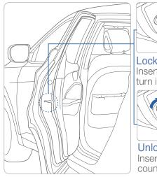
Lock ( $\bigcirc$ ) Insert a key into the hole and turn it to the lock ( $\bigcirc$ ) position.
