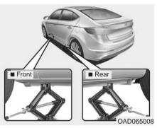
7. Place the jack at the designated jacking position under the frame closest to the tire you are changing. The jacking positions are plates welded to the frame with two notches. Never jack any other position or part of the vehicle. Doing so may damage the side seal molding or other parts of the vehicle.
