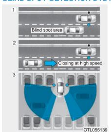
The Blind Spot Detection System (BSD) uses radar sensors in the rear bumper to monitor and warn the driver of an approaching vehicle in the driver's blind spot area.
