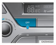
Push the OFF button of the front to turn off the air climate control system. You can still operate the mode and air intake buttons as long as the ignition switch is in the ON position.
