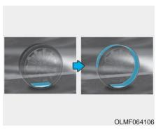
Immediately drive approximately 7~10 km (4~6 miles or, about 10min) to evenly distribute the sealant in the tire. Do not exceed a speed of 80 km/h (50 mph). If possible, do not fall below a speed of 20 km/h (12 mph).
