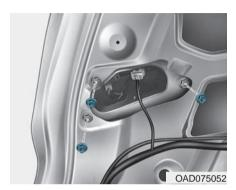
Disconnect the connector and then remove the nuts by turning the nuts counter clockwise.
