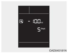
To reset the service interval, press the RESET button for more than 5 seconds and then when the miles and days blink press the RESET button for more than 1 second.
