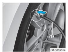
4. Unscrew the valve cap from the valve of the flat tire and screw the filling hose (9) of the sealant bottle onto the valve.
