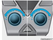
Turn the knob to the right to increase the fan speed temperature and airflow. Turn the knob to the left to decrease fan temperature.
