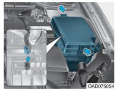
Before inspecting a fuse, you should turn OFF the engine as well as the other electric system switches.
