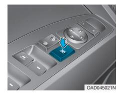
The driver can disable the power window switches on the passenger's doors by pressing the power window lock switch. When the power window lock switch is pressed:
