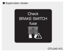
This warning message is displayed if the brake switch fuse is disconnected.
