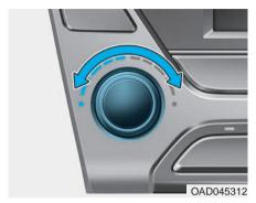
Turn the temperature control knob to the desired temperature. If the temperature is set to the lowest setting (Lo), the air conditioning system will operate continuously. To turn the automatic operation off, select any button of the following:
