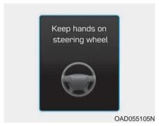
If the driver takes their hands off the steering wheel for several seconds while the LKAS is activated, the system will warn the driver with a visual and audible warning.
