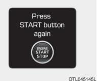
This message is displayed if you were unable to start the vehicle when the Start/Stop button was pressed.
