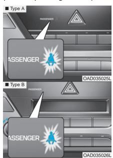
As a reminder to the front passenger, the front passenger's seat belt warning lights will illuminate for approximately 6 seconds each time you turn the ignition switch ON regardless of belt fastening.
