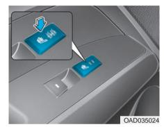
While the engine is running, push either of the switches to warm the rear seat. During mild weather or under conditions where the operation of the seat warmer is not needed, keep the switches in the OFF position.
