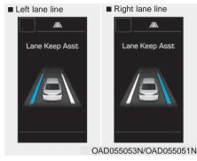
If all the conditions to activate LKAS is not satisfied, the system will convert to LDWS (Lane Departure Warning System) and warn the driver only when the driver crosses the lane lines.
