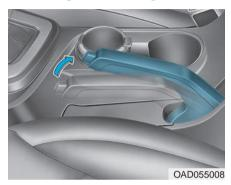
Check the stroke of the parking brake by counting the number of "clicks" heard while fully applying it from the released position. Also, the parking brake alone should securely hold the vehicle on a fairly steep grade. If the stroke is more or less than specified, have the parking brake adjusted by an authorized HYUNDAI dealer.
