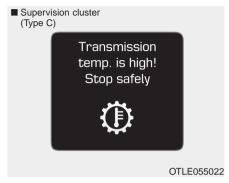
2. Transmission High Temperature When the clutch temperatures are too high, the "Transmission temp is high!" warning message will appear on the LCD display, a chime will sound, and the transmission shifting may not be smooth.
