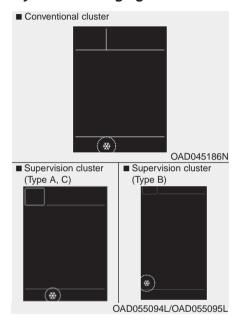
This warning light is to warn the driver the road may be icy. When the temperature on the outside temperature gauge is approximately below 40°F (4°C), the lcy Road Warning Light and Outside Temperature Gauge blinks, and then illuminates. Also, the warning chime sounds 1 time.
