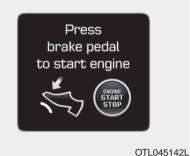
This warning message is displayed if the Engine Start/Stop button changes to the ACC position twice by pressing the button repeatedly without depressing the brake pedal.
