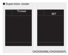
The indicator is displayed when the cruise control system is enabled and the cruise control speed is set.
