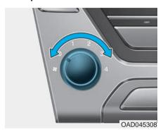
Turn the knob to the right to increase the fan speed and airflow. Turn the knob to the left to decrease fan speed and airflow.
