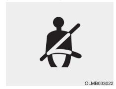
As a reminder to the driver, the seat belt warning light will illuminate and warning chime will sound for approximately 6 seconds each time you turn the ignition switch ON if the seat belt is unfastened.
