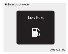
This warning message is displayed if the fuel tank is almost out of fuel.
