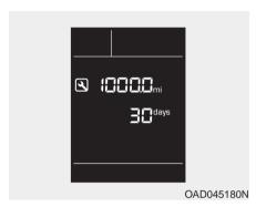
If the remaining mileage or time reaches 900 miles (1,500 km) or 30 days, the service symbol ( ) will blink for several seconds each time you set the ignition switch or Engine Start/Stop button to the ON position.
