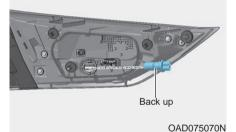
Remove the socket from the assembly by turning the socket counterclockwise until the tabs on the socket align with the slots on the assembly.
