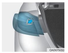
4. Remove the rear combination light assembly from the body of the vehicle.
