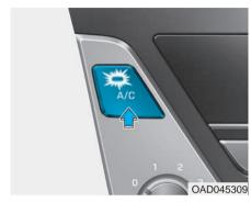
Press the A/C button to turn the system on (indicator light will illuminate) and off.
