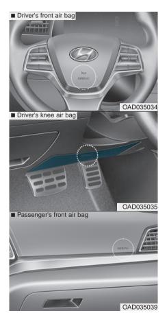
The purpose of the SRS is to provide the vehicle's driver and front passengers with additional protection than that offered by the seat belt system alone. The SRS uses sensors to gather information about the driver's and front passenger's seat belt usage and impact severity.
