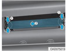
Remove the climate control air filter case by pulling out the both side of the cover.
