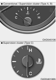
This gauge indicates the temperature of the engine coolant when the ignition switch or Engine Start/Stop button is ON.
