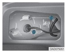
3. Loosen the assembly retaining nuts.
