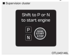
This warning message is displayed if you try to start the engine with the shift lever not in the P (Park) or N (Neutral) position.
