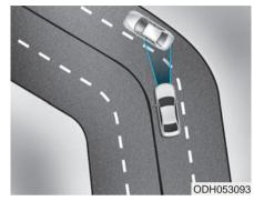
Your vehicle speed can be reduced due to a vehicle in the adjacent lane.
