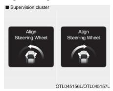
This warning message is displayed if you start the engine when the steering wheel is turned to more than 90 degrees to the left or right.
