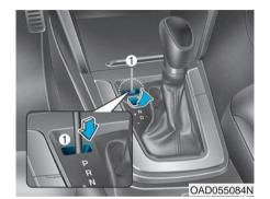
If the shift lever cannot be moved from the P (Park) position into R (Reverse) position with the brake pedal depressed, continue depressing the brake, and then do the following:
