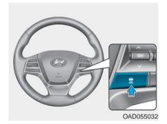
When the Smart Cruise Control System is ON, you can set and maintain the distance from the vehicle ahead of you without pressing the accelerator or brake pedal.
