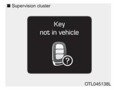
This warning message is displayed if the smart key is not in the vehicle when you press the Engine Start/Stop button.
