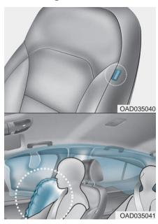
Your vehicle is equipped with a side air bag in each front seat. The purpose of the air bag is to provide the vehicle's driver and the front passenger with additional protection than that offered by the seat belt alone.
