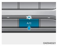
Push the A/C button to manually turn the system on (indicator light will illuminate) and off.
