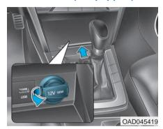
The power outlet is designed to provide power for mobile telephones or other devices designed to operate with vehicle electrical systems. The devices should draw less than 180 W (Watts) with the engine running.
