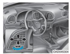
The outlet vents can be opened ( $\circledast$ ) or closed ( $\bigcirc$ ) separately using the thumbwheel.
