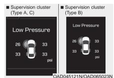
When the tire pressure monitoring system warning indicators are illuminated and the warning message is displayed on the cluster LCD display, one or more of your tires is significantly under-inflated. The LCD position indicator will indicate which tire is significantly under-inflated by illuminating the corresponding position light.
