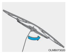
Raise the wiper arm and slightly rotate the wiper blade assembly to expose the plastic locking clip.
