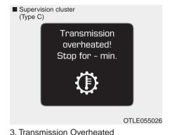
If the vehicle continues to be driven and the clutch temperatures reach the maximum temperature limit, the "Transmission overheated!" warning will be displayed. When this occurs the clutch is disabled until the clutch cools to normal temperatures.
