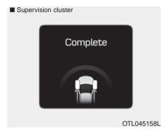
If the steering wheel aligning is completed after "Align steering wheel" warning message is displayed, this message is displayed for 2 seconds.
