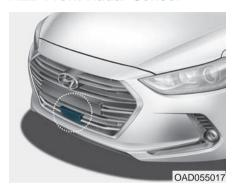
In order for the AEB system to operate properly, always make sure the radar sensor cover is clean and free of dirt, snow, and debris. Dirt, snow, or foreign substances on the lens may adversely affect the sensing performance of the radar.
