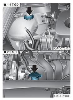
Check the condition and connections of all cooling system hoses and heater hoses. Replace any swollen or deteriorated hoses. The coolant level should be filled between the F and the L marks on the side of the coolant reservoir when the engine is cool.
