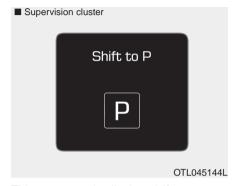
This message is displayed if you try to turn off the engine without the shift lever in P (Park) position.
