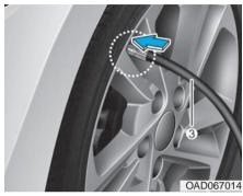
4. Unscrew the valve cap from the valve of the detective wheel and screw the filling hose (3) of the sealant bottle onto the valve.
