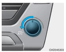
The MAX A/C mode is used to cool the inside of the vehicle faster. Air flow is directed toward the upper body and face. In this mode, the air conditioning and the recirculated air position cannot be selected. Turn the fan speed mode to adjust.
