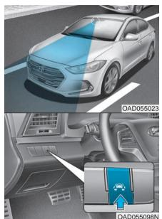
The Lane Keeping Assist System detects lane markers on the road, and assists the driver's steering to help keep the vehicle between lanes.
