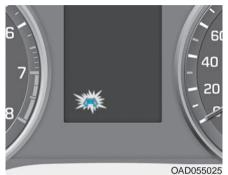
The LKAS failure indicator (yellow) will illuminate if the LKAS is not working properly. Have your vehicle checked by an authorized HYUNDAI dealer.
