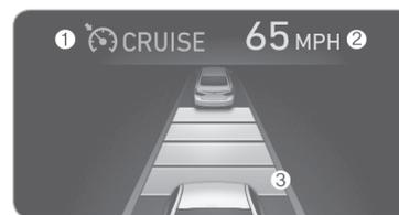
If your vehicle is equipped with Advanced smart cruise control and you wish to eliminate the vehicle distance function, you can change cruise control setting to a standard setting.
