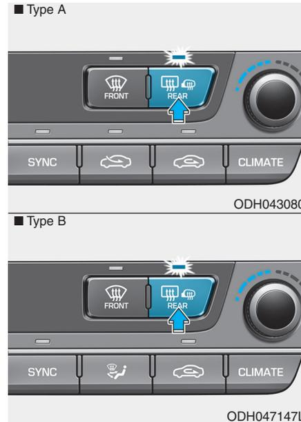
The defroster heats the window to remove frost, fog and thin ice from the interior and exterior of the rear window, while engine is running.
