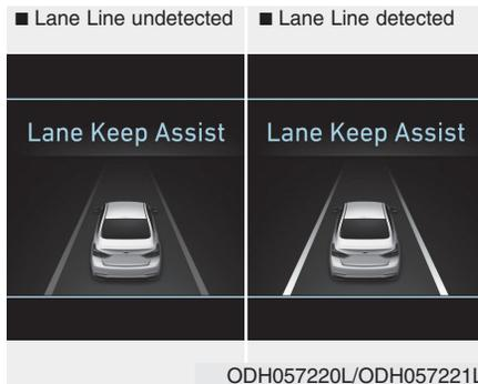
If the speed of the vehicle is over 40 mph (64 km/h) and the system detects lane markers, the color changes from gray to white.
