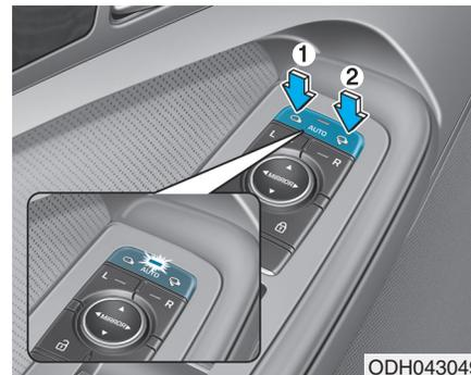
The side view mirror can be folded or unfolded by pressing the switch when:
