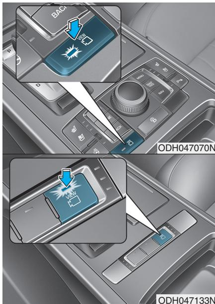
The Multi-View Camera System can assist in parking by allowing the driver to see around the vehicle.
