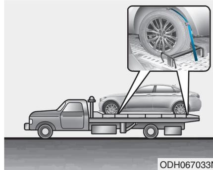
When towing the vehicle by flatbed equipment, secure wheels by using chocks and tie-down straps (or soft belts).
