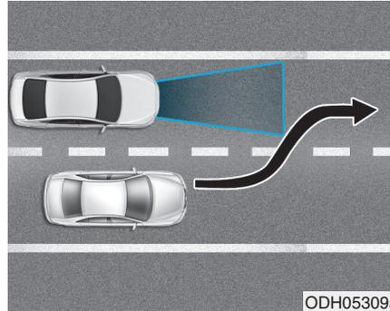
A vehicle which moves into your lane from an adjacent lane cannot be recognized by the sensor until it is in the sensor's detection range.
