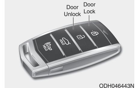
To lock the doors, press the button on the outside door handle while carrying the smart key with you or press the door lock button on the smart key.
