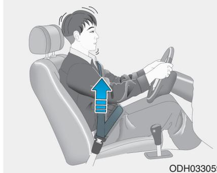
The purpose of the Pre-Active Seat Belt is to tighten the seat belt when a collision is sensed, driving emergency braking, or when a loss of control is sensed.
