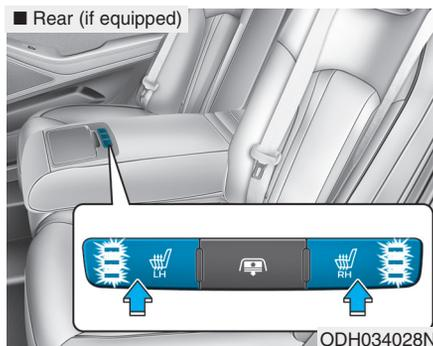
While the engine is running, push the switch to warm the seat.
