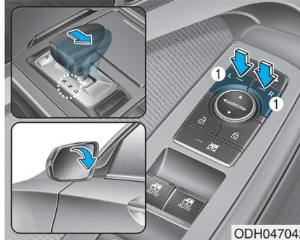
When you move the shift lever to the R (Reverse) position, the side view mirror(s) will rotate downwards to aid with driving in reverse. The position of the side view mirror switch (1) determines whether or not the mirrors will move:
