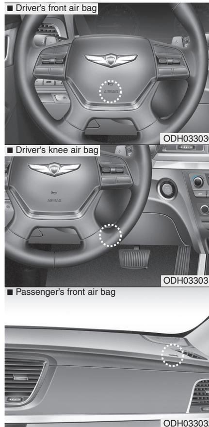
The purpose of the SRS is to provide the vehicle's driver and front passengers with additional protection than that offered by the seat belt system alone. The SRS uses sensors to gather information about the driver's seat position, the driver's and front passenger's seat belt usage and impact severity.
