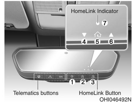
Your vehicle may be equipped with a Gentex Automatic-Dimming Mirror with a Z-Nav™ Electronic Compass Display and an Integrated HomeLink® Wireless Control System. During nighttime driving, this feature will automatically detect and reduce rearview mirror glare while the compass indicates the direction the vehicle is pointed. The HomeLink® Universal Transceiver allows you to activate your garage door(s), electric gate, home lighting, etc.
