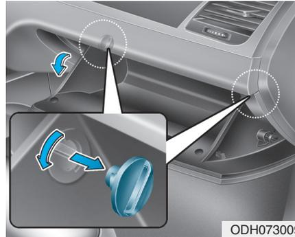
1. With the glove box open, remove the stoppers on both sides to allow the glove box to hang freely on the hinges.
