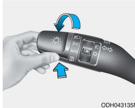
The Smart High Beam is a system that automatically adjusts the headlamp range (switches between high beam and low beam) according to the brightness of other vehicles and road conditions.
