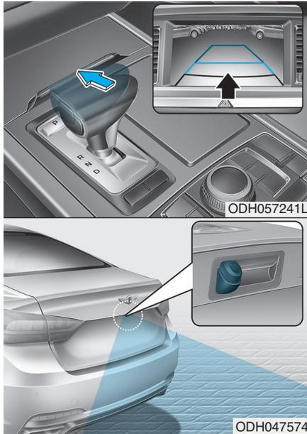
The Rear View Camera will activate when the engine is running and the shift lever is in the R (Reverse) position.
