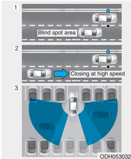
The Blind Spot Detection System (BSD) uses radar sensors in the rear bumper to monitor and warn the driver of an approaching vehicle in the driver's blind spot area.
