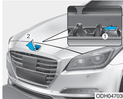
3. Raise the hood slightly, push the secondary latch up (1) inside of the hood center and lift the hood (2). After it has been raised about halfway, it will raise completely by itself.
