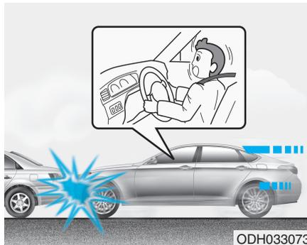
In certain low-speed collisions the air bags may not deploy. The air bags are designed not to deploy in such cases because they may not provide benefits beyond the protection of the seat belts.
