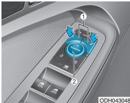
1. Press either the L (driver's side) or R (passenger's side) button (1) to select the side view mirror you would like to adjust.
