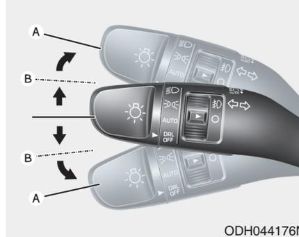
To signal a turn, push down on the lever for a left turn or up for a right turn in position (A). To signal a lane change, move the turn signal lever slightly and hold it in position (B). The lever will return to the OFF position when released or when the turn is completed.
