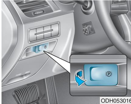
To apply the EPB (Electronic Parking Brake):
