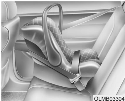
A rear-facing child seat provides restraint with the seating surface against the back of the child. The harness system holds the child in place, and in an accident, acts to keep the child positioned in the seat and reduce the stress to the neck and spinal cord.
