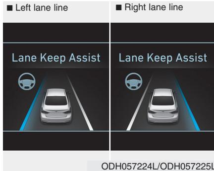
If the vehicle moves out its lane because steering torque for assistance is not enough, the line indicator of deviation direction will blink.
