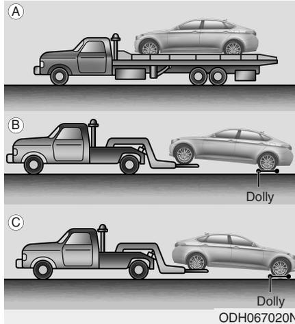
If emergency towing is necessary, we recommend having it done by an authorized retailer of Genesis Branded products or a commercial tow-truck service. Proper lifting and towing procedures are necessary to prevent damage to the vehicle. The use of wheel dollies or flatbed is recommended.
