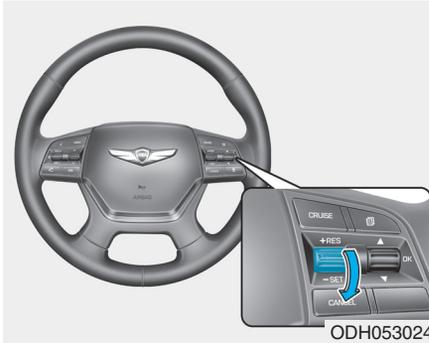
3. Push the toggle switch down (SET-), and release it at the desired speed. The Set Speed and Vehicle-to-Vehicle Distance on the LCD display will illuminate.
