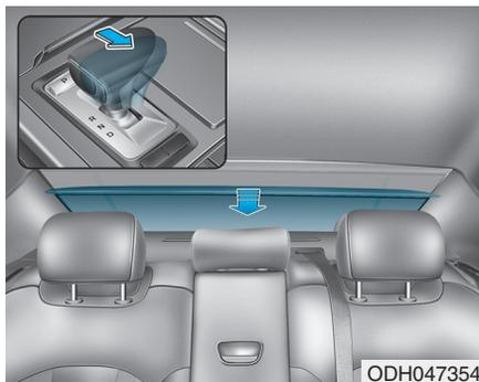
The rear curtain will be lowered automatically when you shift the shift lever into R (Reverse) and raised automatically when you shift the shift lever from R (Reverse) into P (Park). After the rear curtain is lowered by shifting into R (Reverse), if you drive more than 12 mph (20 km/h) with the shift lever in D (Drive), the rear curtain will be raised automatically.
