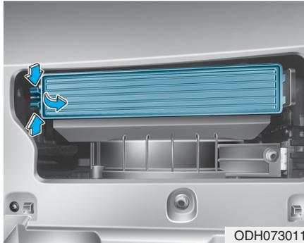
3. Remove the climate control air filter case by pulling out left sides of the cover.
