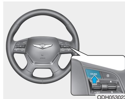
1. Push the CRUISE button on the steering wheel to turn the system on. The CRUISE indicator will illuminate.
