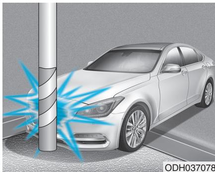
Air bags may not inflate if the vehicle collides with objects such as utility poles or trees, where the point of impact is concentrated and the collision energy is absorbed by the vehicle structure.
