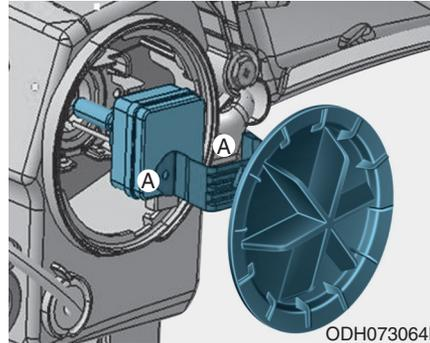
Push the socket into the assembly and turn the socket clockwise.
