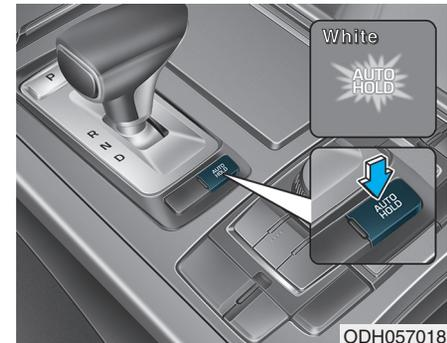
1. Press the [AUTO HOLD] switch. The AUTO HOLD indicator will illuminate white and the system will be in the standby position.
