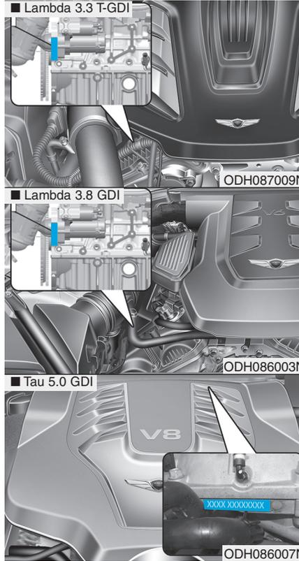
The engine number is stamped on the engine block as shown in the drawing.
