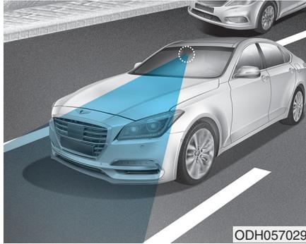
The Lane Keeping Assist System detects the lane markers on the road with a camera at the front windshield, and assists the driver's steering to help keep the vehicle in the lanes.
