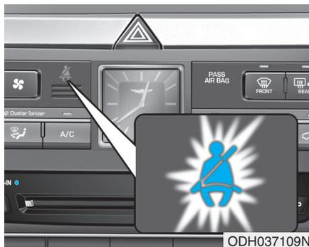
The front passenger's seat belt warning light will activate to the following table when the Engine Start/Stop button is in "ON" position.
