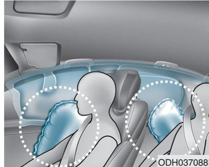
Your vehicle is equipped with a side air bag in each front and outboard rear seat. The purpose of the air bag is to provide the vehicle's driver and/or the front and outboard rear passenger with additional protection than that offered by the seat belt alone.
