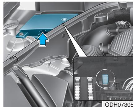
5. Pull the suspected fuse straight out. Use the removal tool provided in the engine compartment fuses panel.
